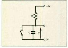
Fig.3. Simple circuit to demonstrate capacitor charging.
