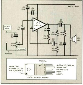
Fig.9. Circuit diagram for a single TDA2003 Amp.
