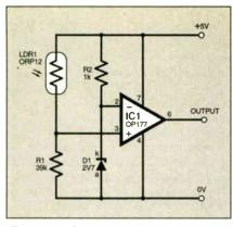
Fig.7.18. Comparator circuit without hysteresis.
