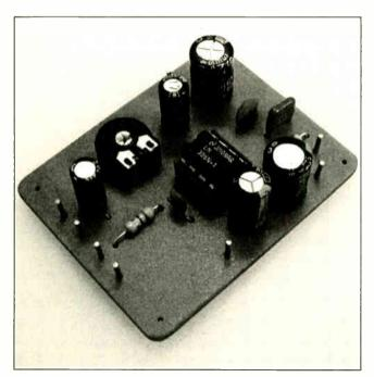
Completed LM386N-1 circuit board.
