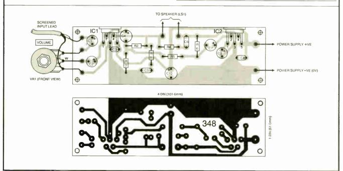
The printed circuit board component layout, wiring and copper foil master are detailed in Fig.12. Again, combined or separate heatsinks must be fitted to the integrated circuit's metal tabs. The p.c.b. is obtainable from the EPE PCB Service, code 348 (Twin TDA22003).
