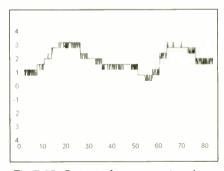
Fig.7.25. Output of anemometer showing wind speed variation.
