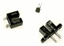
Typical examples of slotted and reflective photosensors. lamps, so precautions must still be taken to reduce ambient light as much as possible.
