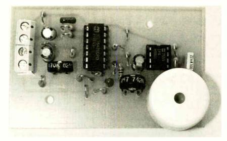
Component layout on the finished circuit board.
