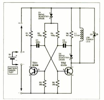
Fig.1. Circuit diagram for the Battery Discharger.
