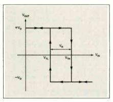
Fig.7.2. Response of an inverting regenerative comparator.
