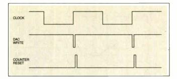
Fig.7.17 (above). Timing diagram of anemometer circuit. Fig.7.16 (left). Block diagram of anemometer circuit.
