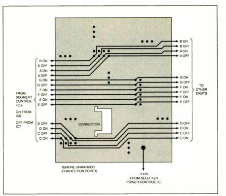
Fig. 13. Wiring details for a single digit.
