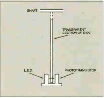
Fig.7.13. Slotted photosensor.
