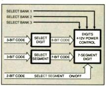
Fig.5. Multiplexed control logic.
