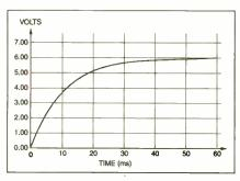
Fig.4. Capacitor charging curve.
