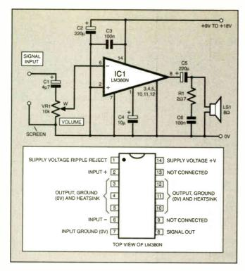
Fig.7. Circuit diagram for the LM380N Amplifier.
