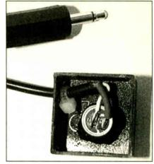
Using screened audio cable to connect the electret microphone to the main unit.
