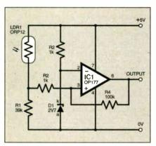
Fig.7.20. Comparator circuit with hysteresis.
