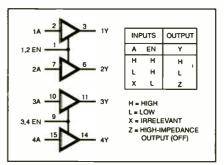
Fig.4. L293DN pinouts and logic table.
