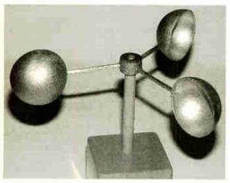
Prototype "homemade" anemometer assembly.
