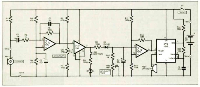
Fig.2. Complete circuit diagram for the Washing Ready Indicator. The battery pack B1 is made up of 4 x AA alkaline cells. Everyday Practical Electronics, May 2002
