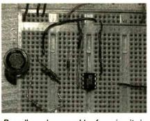
Breadboard assembly for circuit in Fig.7.18.
