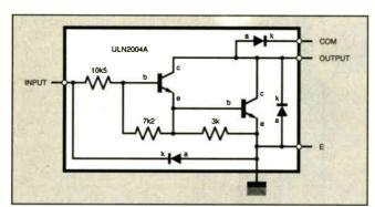
Fig.3. Schematic of one stage within a ULN 2004A 7-stage line driver.
