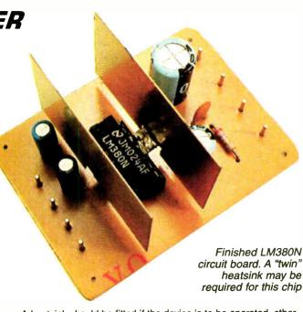
A heatsink should be fitted if the device is to be operated, other than intermittently, at output levels in excess of 1W. Without a heatsink, the suggested maximum supply voltages are: with a 4 ohm speaker 12V with an 8 ohm speaker 15V Frequency response up to 100kHz
