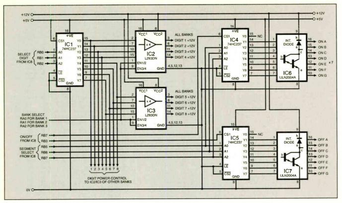
Fig.6. Circuit diagram for the multiplexed control of the digits, basically for eight, but can be modified to control 64 digits.
