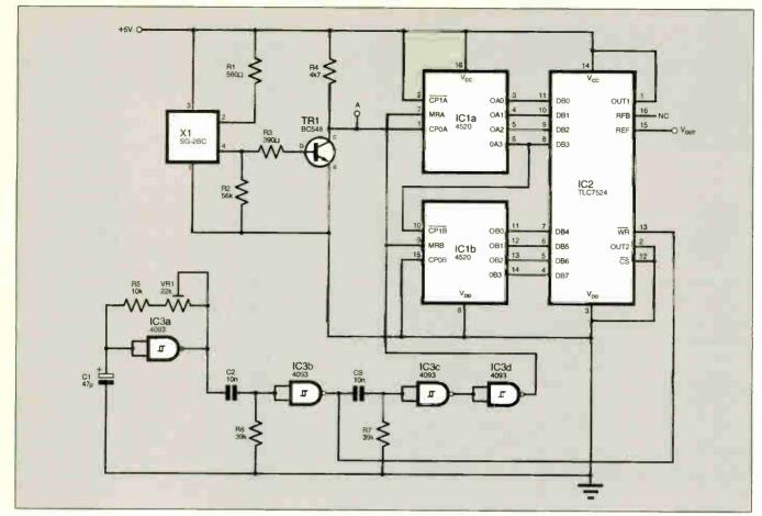
Fig.7.22. Circuit diagram for the anemometer.
