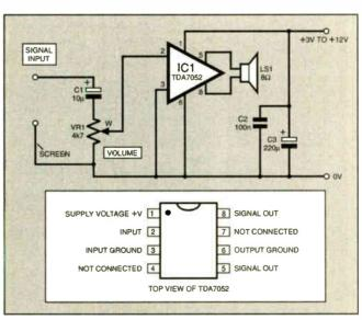
Fig.3. Circuit diagram and pinout details for the TDA7052 Amp. See left for performance guide.
