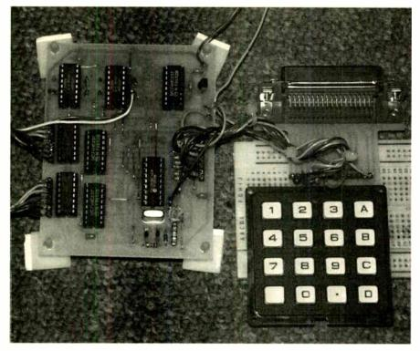
Prototype display controller board during development testing using a plug-in breadboard to temporarily connect a data keypad and a PC via a Centronics connector (mounted on the p.c.b. used with Teach-In 2000 Part 4 – Feb '00).
