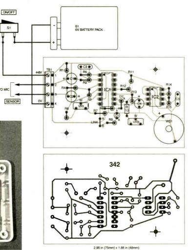
Fig.3. Printed circuit board component layout, full-size copper foil master and wiring
