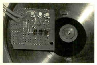
Above: Stripboard assembly mounting for the wind vane.
