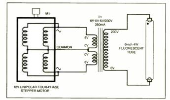
Fig.2. Emergency Light circuit diagram.
