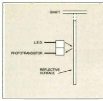
Fig.7.14. Reflective photosensor.
