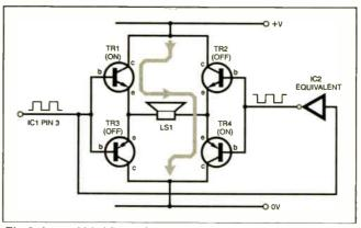
Fig.3. In an H-bridge driver, opposing pairs of complementary transistors drive the load as shown by the path (tint) taken by the current. (One phase of full circuit is shown.)
