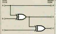
Fig.7.9. Gray code to binary code converter.
