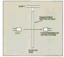
Fig.7.12. Sensing using a separate l.e.d. and photosensor.
