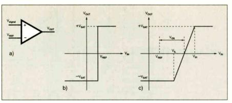
Fig.7.1. Comparator input-output characteristics, (a) schematic, (b) ideal response, (c) realistic response.
