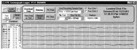
Example of recorded data recalled and displayed on screen. The timings and zone values to the left relate to the white markers in the zones.
