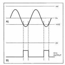
Fig.4. Switching waveforms.
