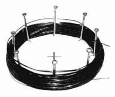
Enamelled copper wire (30s.w.g.) wound around the guide pins.
