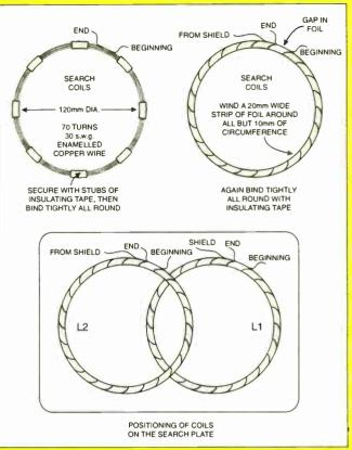
Fig.3. Suggest coil winding details and general positioning of coils on the search head plate. The full coil winding sequence is shown in the photographs.
