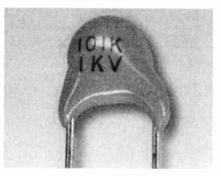
100pF 1kV (1,000V) ceramic capacitor
