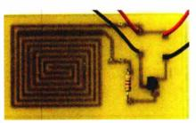
Photo 7.1. Moisture sensing printed circuit board.
