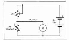
Fig.7.3. A preset potentiometer and resistive sensor as a potential divider.
