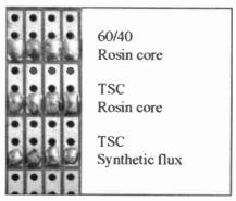
Fig.3. Comparing TSC solder wires with rosin and synthetic flux cores.
