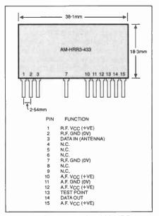
Fig.7.6. Pinouts for the AM-HRR3-433 receiver module.
