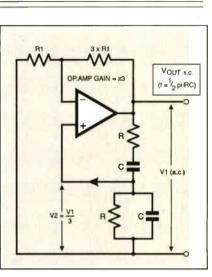
Fig.2. The Wien circuit as the feedback element in an oscillator
