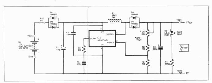
Fig.3. Complete circuit diagram for the In-Car Laptop Power Supply Unit (PSU).
