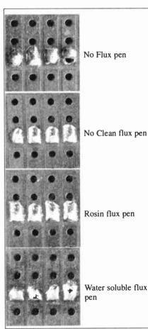
Fig.4. Comparing flux pens on 0.7mm TSC wire.
