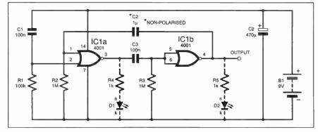
Fig.7.11. Astable circuit with a non-uniform mark-space ratio.
