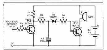
Fig.7.12. Fail-safe signal monitoring circuit.
