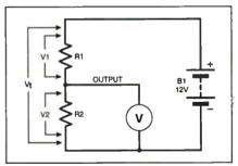
Fig.7.2. Principle of a potential divider circuit.
