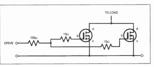
Fig.1. Paralleled MOSFETs with differential gate drive resistors.
