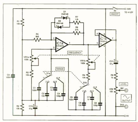
Fig.3. Complete circuit diagram for the Low-Frequency Wien Oscillator. Everyday Practical Electronics, May 2004
