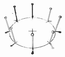
Search coil "pin guide" former, splayed outwards, in a 120mm diameter circle.
