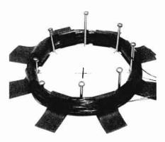
Strips of insulating tape used to hold coil windings together.
