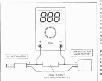
Fig.2. Set-up for monitoring Laptop current.
