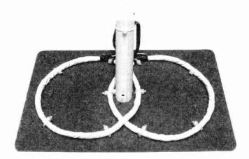
Completed search head, with the coils firmly secured in position by a ring of cable ties, awaiting the potting resin.
