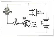
Fig.7.1. Illustrating how an npn transistor can enable a small current, from a moisture sensor for example, to trigger a buzzer.
