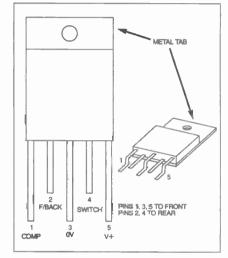
Fig.5. Pinout details for the LM2587.
