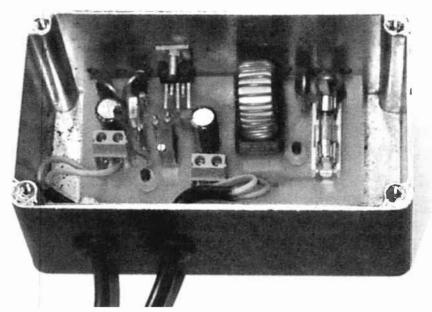
Finished power supply showing the p.c.b. mounted in a diecast box.
