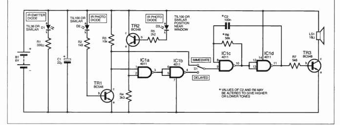
Fig.1. Full circuit diagram for the Mouse Trapped Indicator. Infra-red (IR) emitter diode D1 and IR photo diode D2 are mounted on opposite sides of the "flap".
