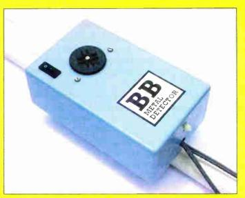
Completed detector unit showing the Sensitivity control knob (disc), on/off switch and search head cable entry.
