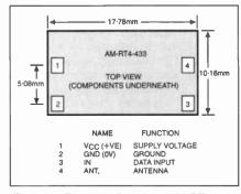
Fig.7.5. Pinouts for the AM-RT4-433 transmitter module.
