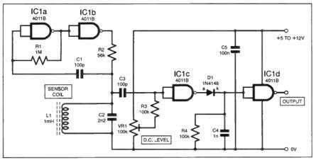
Fig.3. Circuit diagram for a Proximity Switch.
