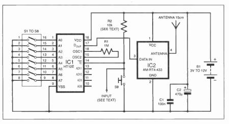
Fig.7.8. Encoder and transmitter circuit.
