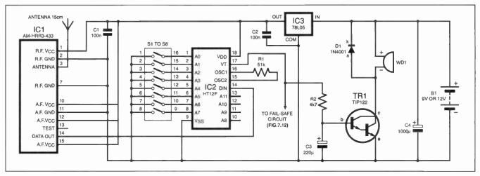
Fig.7.9. Receiver, decoder and driver circuit.
