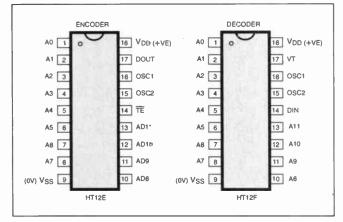
Fig.7.7. Pinouts for the Holtek HT12E and HT12F encoder/decoder i.c.s.
