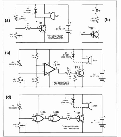
Fig.7.4. Three techniques for monitoring a resistive sensor, plus l.e.d. output instead of a buzzer.
