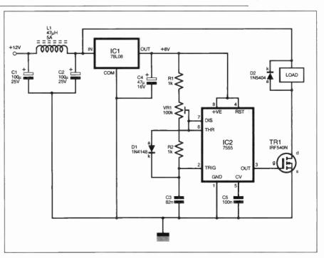
Fig.6. Versatile D.C. Power Controller circuit diagram.
