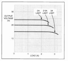
Fig.1. Graph showing maximum current against voltage output.
