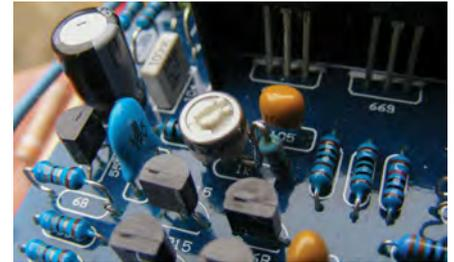
Fig.12a. A quiescent current trimmer  $VR_1$  enables optimisation of bias current.
