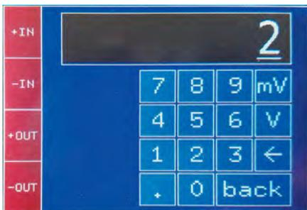
Fig.6: when you touch a value that can be changed, a keyboard like this appears. The keyboard layout changes to suit the value being entered.
