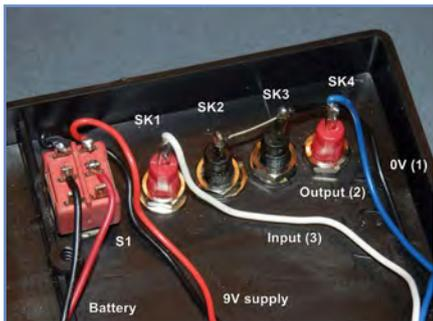
Fig.3.13. Rear panel wiring
