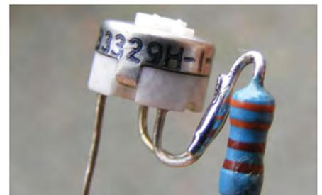
Fig.12d. It is simpler to solder  $R_{17}$  and the  $TO_5$  preset  $VR_1$  together before installing on the board in place of the original  $1\text{k}\Omega$  resistor.
