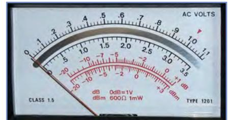
Fig.3.3. Typical dB scales on an AC voltmeter
