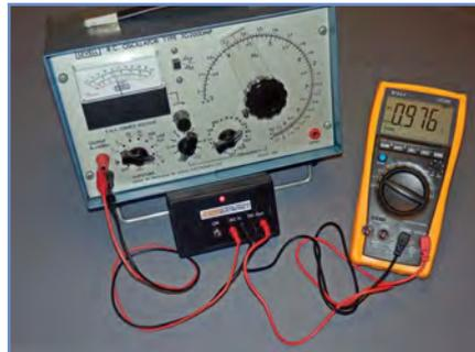
Fig.3.15. Using the wideband AC range extender to check the output of a signal generator. The meter is indicating 0.976V when the signal generator is set to 1V RMS output
