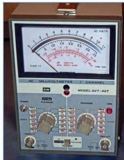
**Fig.3.5. Dual-channel AC millivoltmeter (the meter movement has two separate pointers so that two indications can be produced at the same time)**
