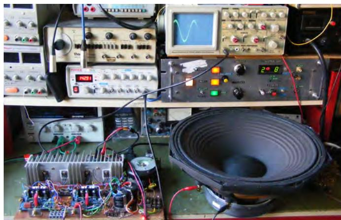
*Fig.13. MX50 prototype being tested for instability with a massive Citronic bass unit. The Citronic unit is rated at 500W and has an inductance of 3.7mH with plenty of resonant back electromotive force (emf) – it upsets most power amplifiers.*
