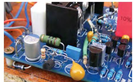
Fig.12c. The new decoupling arrangement showing the capacitance multiplier  $TR_{15}$  with its associated tantalum capacitor. Note also the polymer decoupling capacitor  $C_{11}$ .
