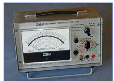
**Fig.3.7. A Level TM6B AC millivoltmeter capable of reading less than 1mV at 3MHz using its external probe**
