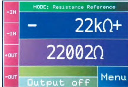
Fig.10: the resistance reference mode is somewhat limited; the selected resistance is shown at the top while the actual resistance is shown below.
