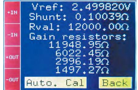
Fig.12: the calibration screen after pressing the Automatic calibration button. Note that the PGA resistors are now shown with the measured values.
