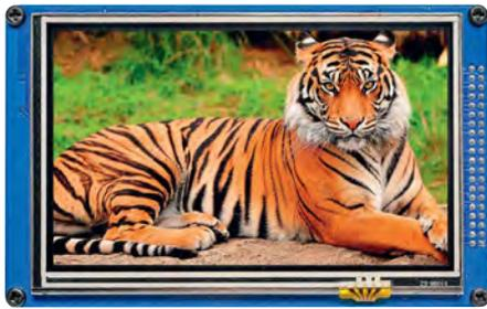
Fig.6: the *Micromite Plus* can drive an LCD panel with up to 800x480 pixels in true (24-bit) colour. This image was loaded from an SD card using the `LOAD IMAGE` command. The speed of loading is not super fast, so you would not use this as a photo frame but it is useful for loading logos and background images.
