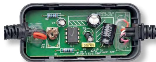
In this amplifier module, the leads were soldered and glued to the PCB, making removal quite difficult.
