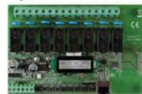
**Computer Controlled / Standalone Unipolar Stepper Motor Driver**
