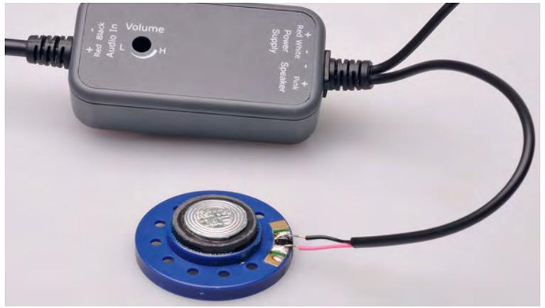
**Step 1:** the Speaker lead from the amplifier module needs to be soldered to the underside of the speaker. It doesn't matter which leads go to which solder pad.
