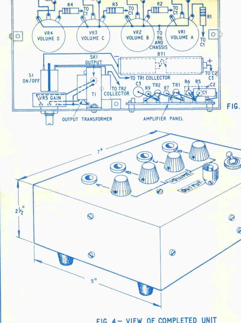
FIG. 4 - VIEW OF COMPLETED UNIT
