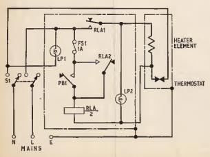
In operation from cold the push button PB1 is depressed energising relay RLA, which is held on by contacts RLA2. Contacts RLA1 are now closed allowing current to be passed through the heater and to lamp LP2. When the circuit is broken by the thermostat, switch S1, or mains failure, relay RLA is deenergised releasing the contacts.
