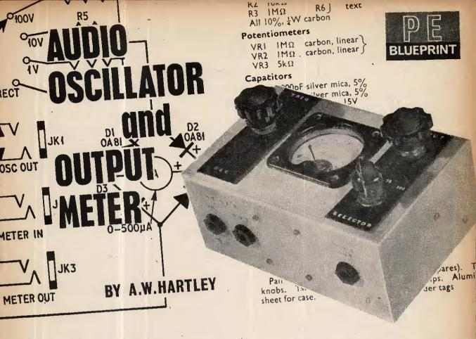
WITH the increasing interest of the experimenter in the field of audio, a compact device which will give an indication of the performance of audio amplifiers and other similar equipment and be a useful guide to the location of a fault during trouble-shooting, is always in demand.
