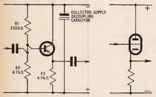
Fig. 4.3. Grounded collector transistor (emitter follower); and grounded anode triode (cathode follower)
