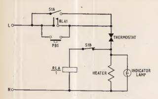
The circuit shows S1 in the "one shot" condition with the thermostat cold. The circuit operation is as follows:
