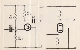
Fig. 4.2. Grounded base transistor and grounded grid triode
