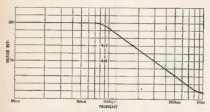
Fig. 13. This curve shows how the response of the Y amplifier falls of at the higher frequencies
