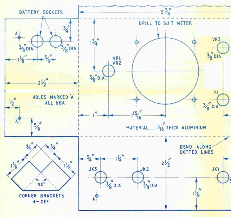
FIG. 4 - CHASSIS DRILLING DETAILS
