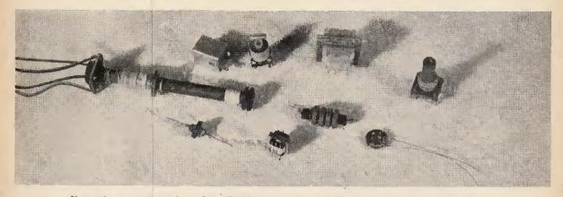
Shown here are a number of small inductors and transformers such as are commonly used in transistorised equipment.
