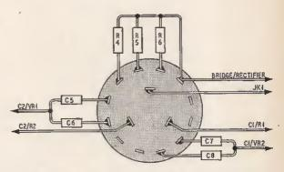
Fig. 6. Connections to SI for modification described in text.
