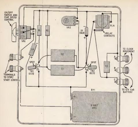
Fig. 2. Details of the component wiring showing positioning of the battery, transistors, relay and preset control VR2. Note that VRI is ganged to the on/off switch
