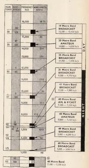
Fig. 11. This chart shows the approximate tuning range of the simple Short Wave Receiver.
