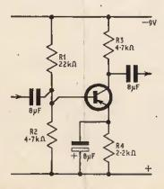
Fig. 4.1. Grounded emitter, or common emitter, connection
