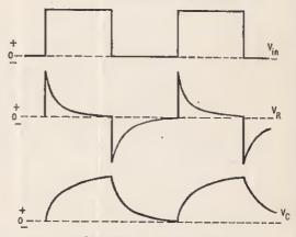
Fig. 2.5d. Shows the voltage that will appear across the input, the resistor and the capacitor
