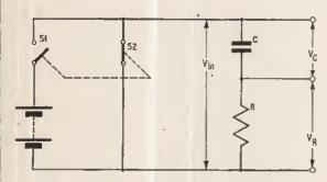
Fig. 2.5c. Circuit rearranged with two switches across the input
