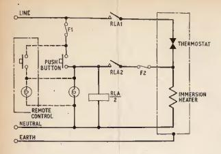
Should contact RLA2 in Peter A. Collier's circuit beat RLA1, then the heater current will be drawn through F1, push button, RLA2, and F2. This means that F1 and F2 will be blown and the push button burnt. This could be avoided by adjusting the relay so that contact RLA1 makes before RLA2. The adjustment of relay contacts is not at all difficult, and only requires time, care and patience.
