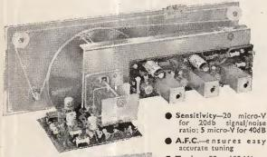
Sensitivity-20 micro-V for 20db signal/noise for 20db signal/noise ratio: 5 micro-V for 40dB
