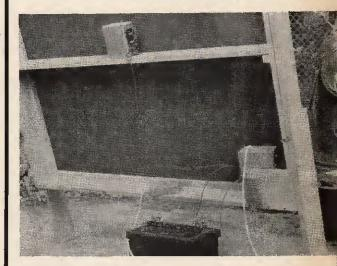
Rear view of the clock showing the units in position and the leads to the I2V car battery which is required to energise the actuating mechanism. The small box houses a press-button switch for remote start and stop
