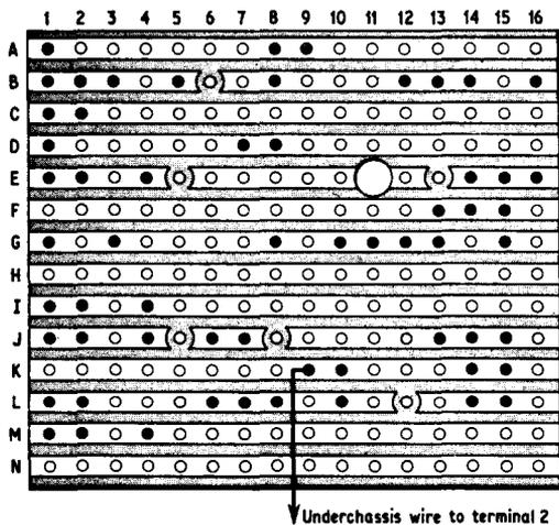
Fig. 2a (right). Modified wiring and layout for negative "earth" systems
