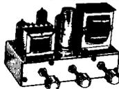
Designed for Hi-Fi reproduction of records. A.C. Mains operation. Ready built on plated heavy gauge metal chassis, size 7 1/2 in. w. x 4 in. d. x 4 1/2 in. h. Incorporates ECC83, EL84, EZ80 valves. Heavy duty, double wound mains transformer
