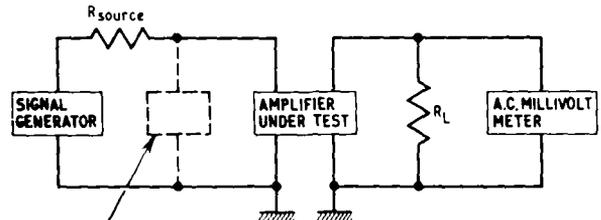
A.C. MILLIVOLT METER MOVED FROM THE OUTPUT, TO CHECK INPUT VOLTAGE.
