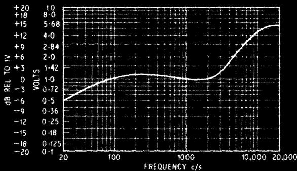
**Fig. 7b.** A typical graph of the frequency response of an audio amplifier with treble boost. The output is plotted in volts (log scale) or decibels (linear scale) against frequency (log scale)
