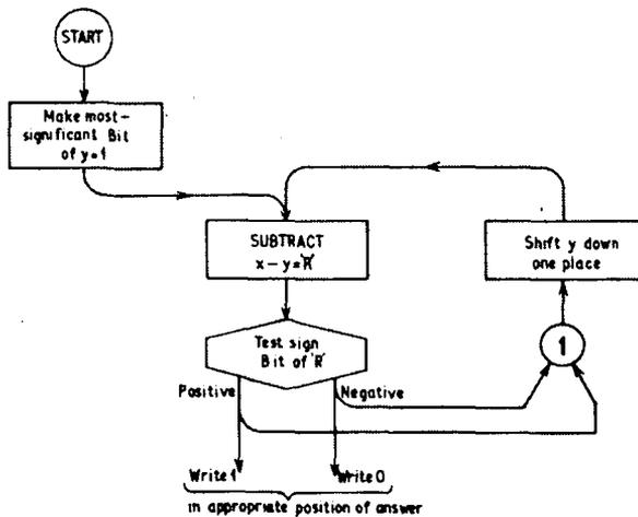
Fig. 6.1. Basis of a flow diagram for division operation
