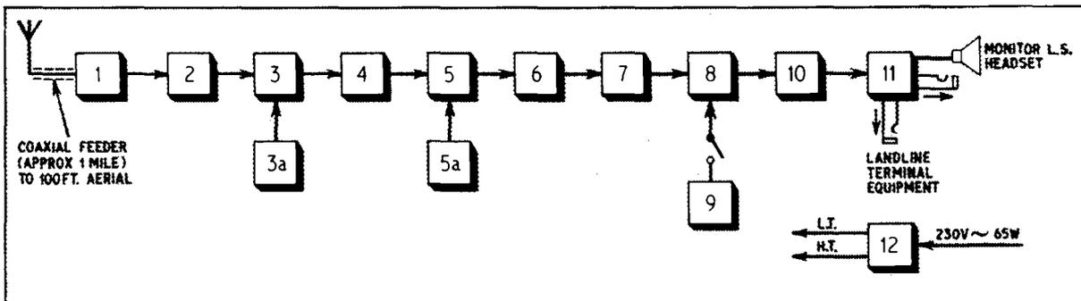
Fig. 4. Block diagram of Marconi "Mercury" receiver
