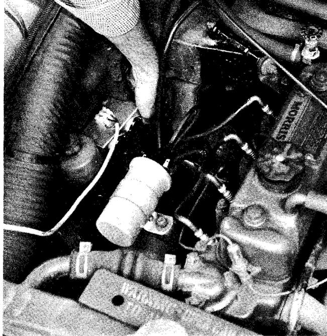
Mount the unit away from heat source and in the direct path of air flow to keep it cool
