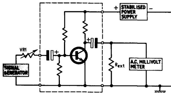
Fig. 9. Set-up for measuring input impedance
