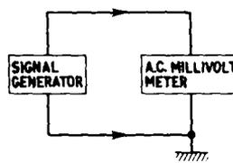
Fig. 3. Measurement of signal generator output—no load condition
