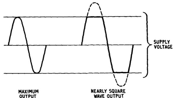
Fig. 6. The effect of boosting any frequency above specified maximum voltage causes distortion
