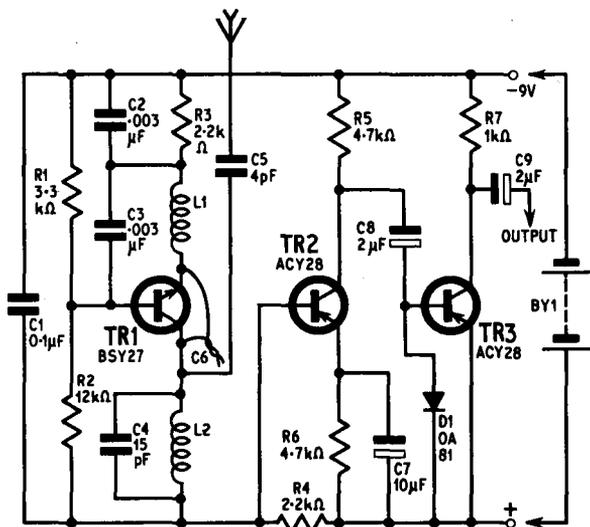
Fig. 1. Circuit diagram of the complete receiver
