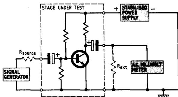
Fig. 8. Set-up for measuring distortion and stage gain
