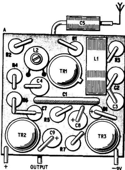
Fig. 2a (left). Layout of components on the board shown double scale
