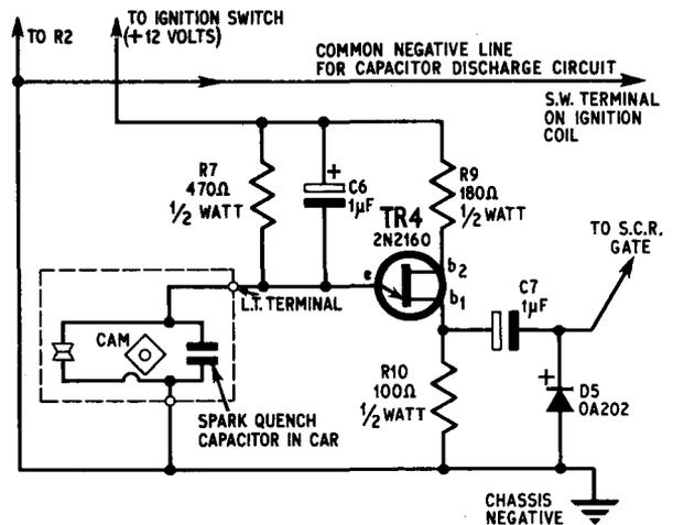
Fig. 1. Amended circuit of the trigger for negative "earth" systems
