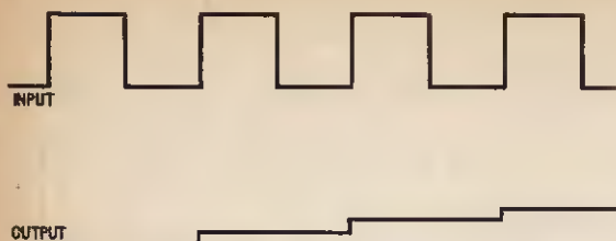
Fig. 6. Waveforms of the diode pump input and output
