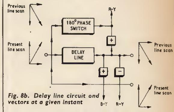
Fig. 8b. Delay line circuit and vectors at a given instant
