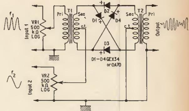
Fig. 5. Ring modulator. The output signal consists of  $f_1$  and  $f_2$  plus their sum and difference frequencies. The resulting sound is an unusual chord
