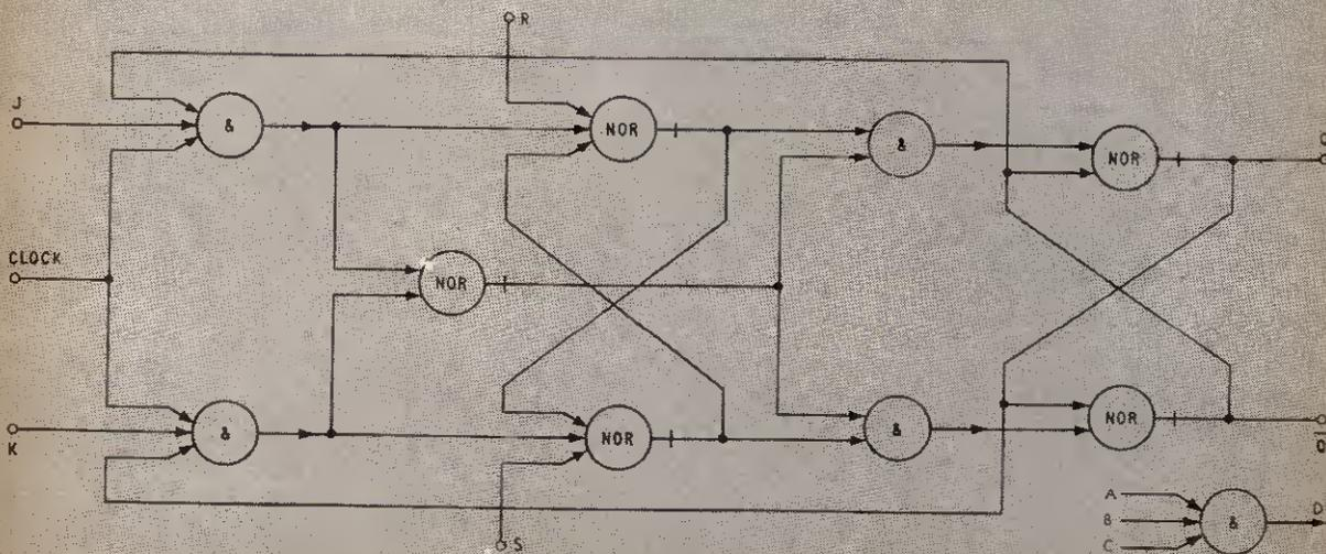
Fig. 20a. Logic diagram of the JK binary
