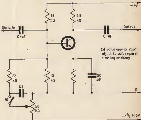
Fig. 2b. A suggested transistor decay circuit; prone to generating clicks when key S1 is closed
