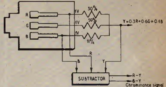
Fig. 2b. Attenuation to each colour to provide chrominance signals
