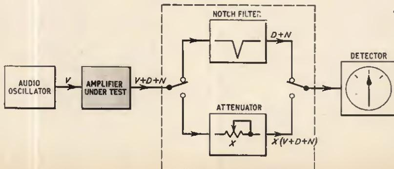
Fig. 2. Block diagram showing method of measuring distortion
