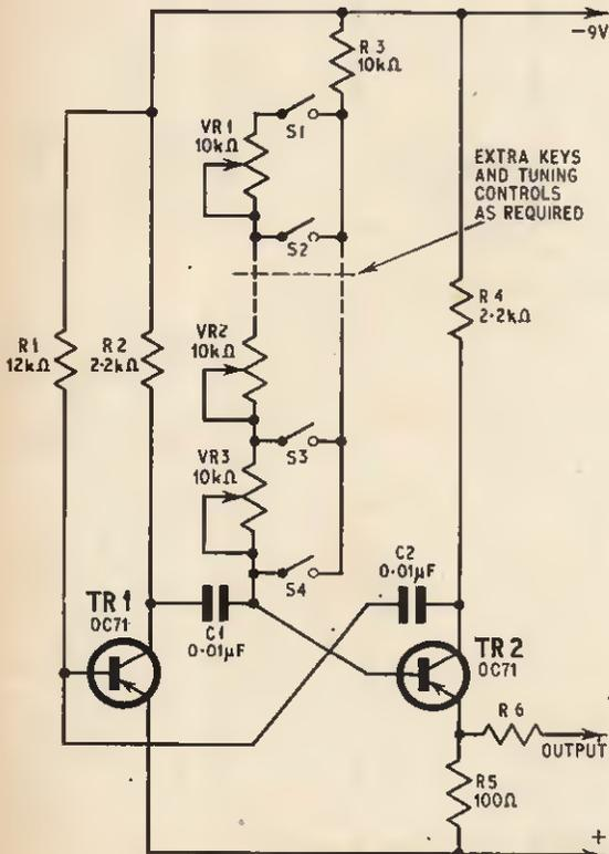
Fig. 4. A suggested transistor square wave generator tuned by adjustment of VR1, 2, and 3. Pitch can be selected by S1, 2, 3, 4
