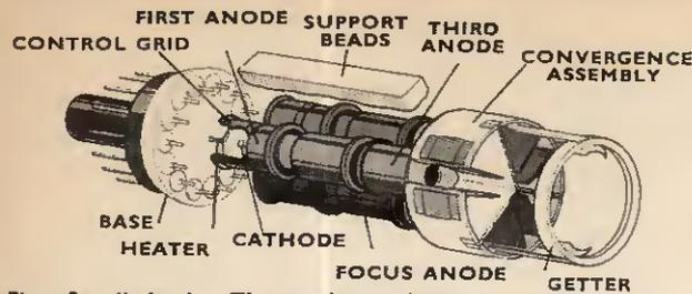
Fig. 5a (below). Three-colour electron gun assembly
