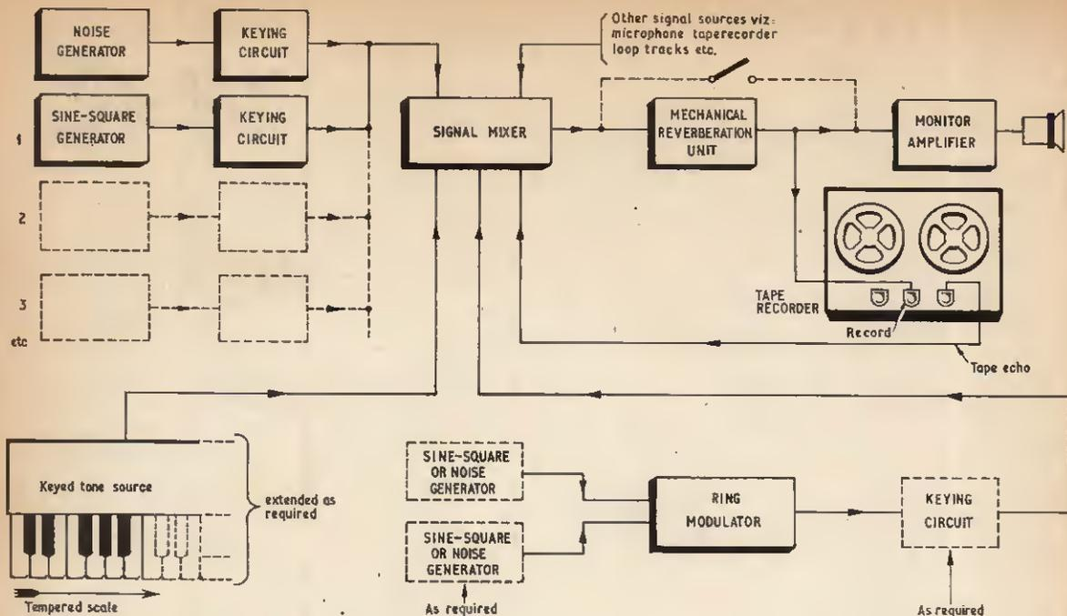
Fig. 8. Typical set-up for recording various tones and sound effects
