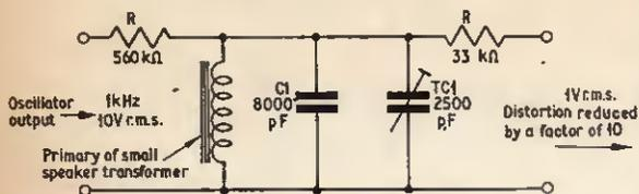
Fig. 12b. Inductive filter circuit
