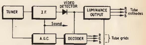
Fig. 6. Block diagram of the colour receiver
