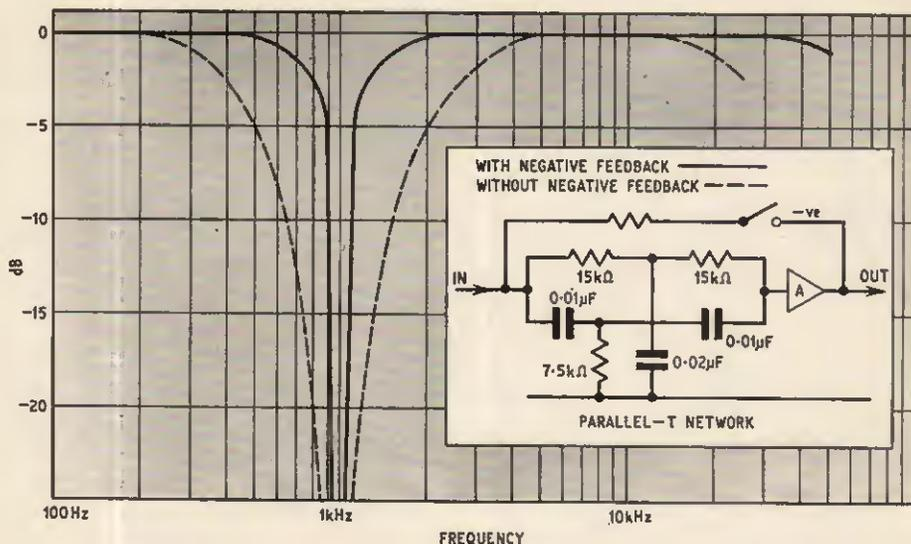
Fig. 1. Frequency response of parallel-T network
