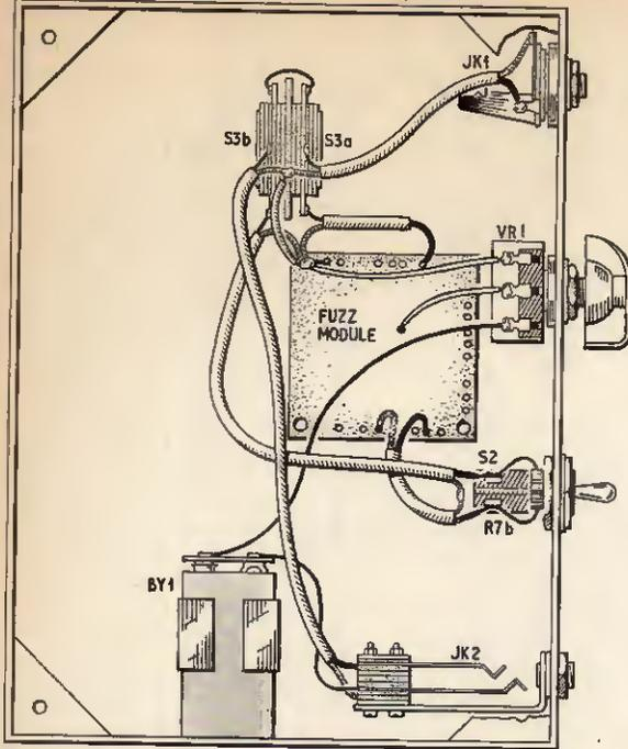
Fig. 6. Layout of components in the chassis for the simple version of the fuzz box
