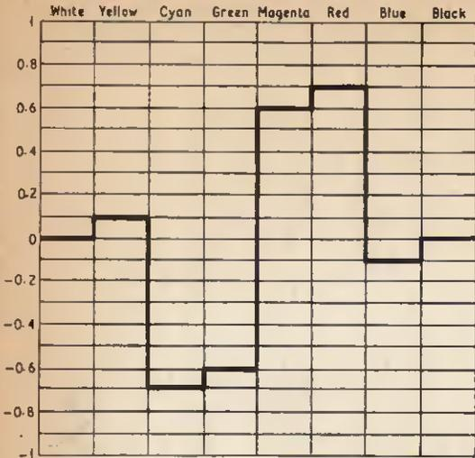
Fig. 3.  $(R - Y)$  waveform through the light spectrum
