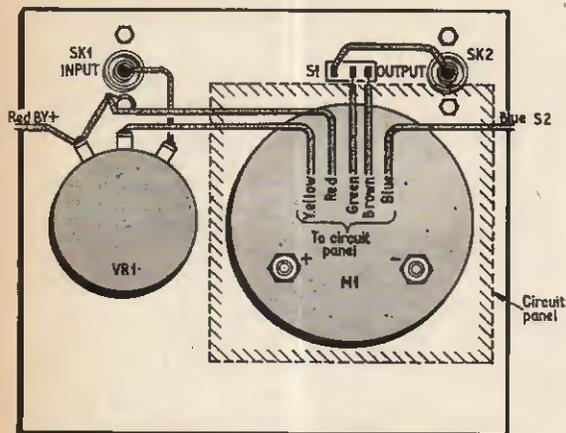
Fig. 10b. Front panel controls and wiring
