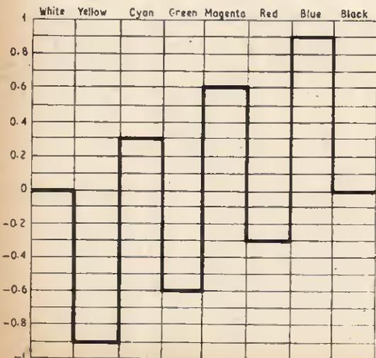
Fig. 4.  $(B - Y)$  waveform through the light spectrum
