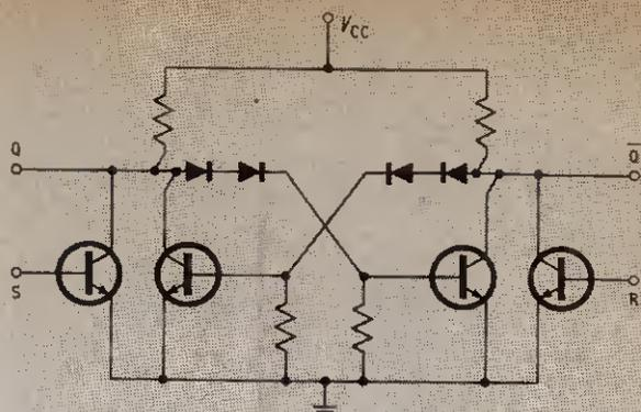
Fig. 19b. Typical circuit of an RS flip-flop
