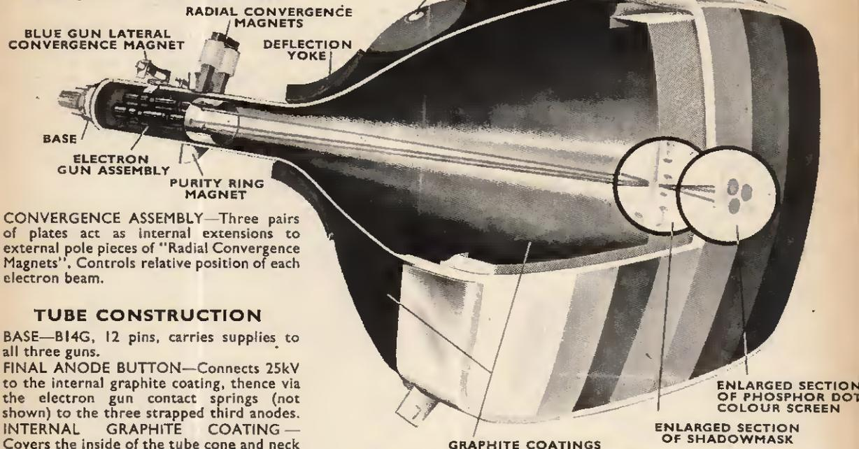
**CONVERGENCE ASSEMBLY**—Three pairs of plates act as internal extensions to external pole pieces of "Radial Convergence Magnets". Controls relative position of each electron beam.
