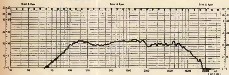
The above curve was taken by an independent testing laboratory and shows clearly why the Sinclair Q.14 achieves such remarkable standards of reproduction. Level response is maintained to assure the user of the finest possible results from the equipment to which the speaker is coupled.
