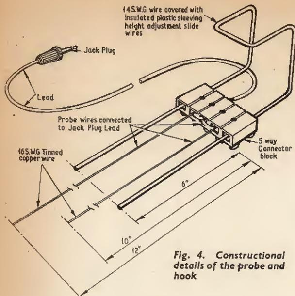
Fig. 4. Constructional details of the probe and hook
