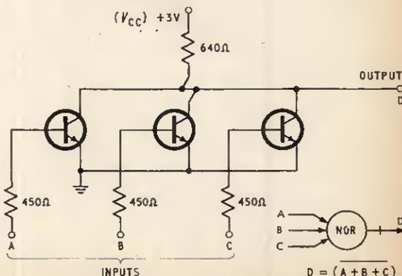
Fig. 15a. A typical RTL NOR gate
