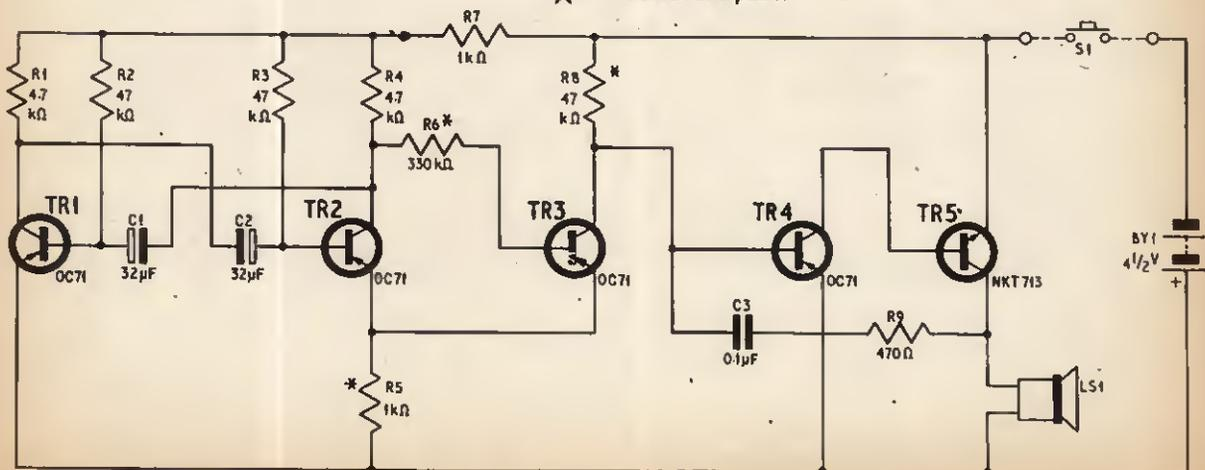
Fig. 1. Circuit diagram of the complete "Yodeller" Door Monitor
