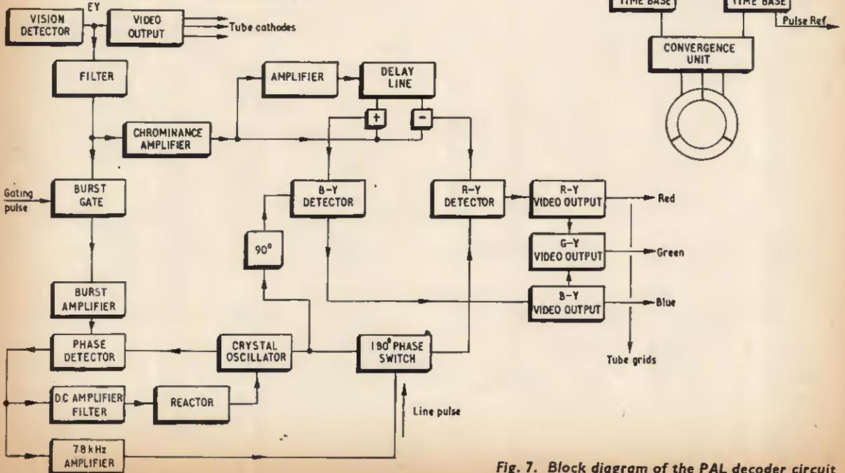
Fig. 7. Block diagram of the PAL decoder circuit
