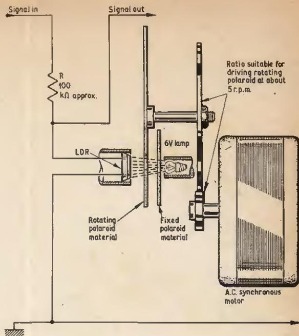
Fig. 6. No-thump vibrato using a photo-sensitive cell with polarised light filters
