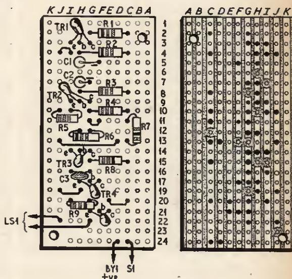
Fig. 2. Component layout and underside view of the Veroboard panel
