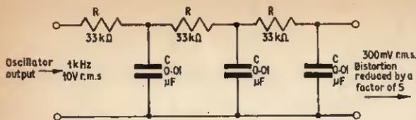
Fig. 12a. Ladder filter circuit
