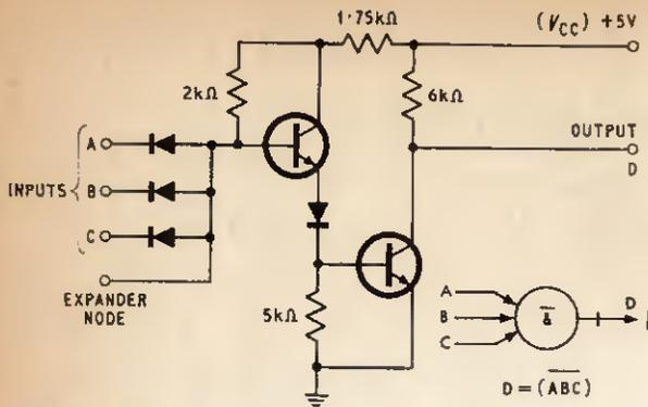
Fig. 16a. Basic DTL NAND gate Fig. 16b. Logic symbol for NAND gate
