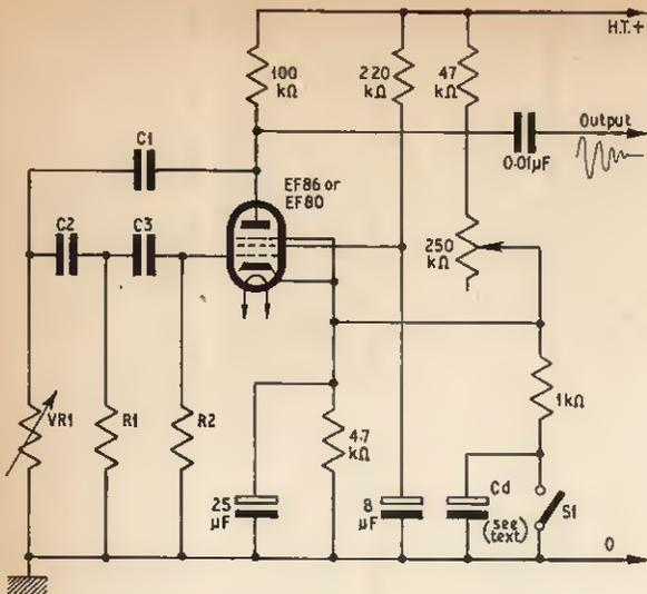
Fig. 3. Decay applied directly to a phase shift oscillator. The values of C1, C2, C3, VR1, R1, and R2 will depend on the frequency required. VR1 gives a fine adjustment of the nominal frequency
