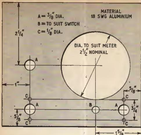
Fig. 10a. Front panel drilling details
