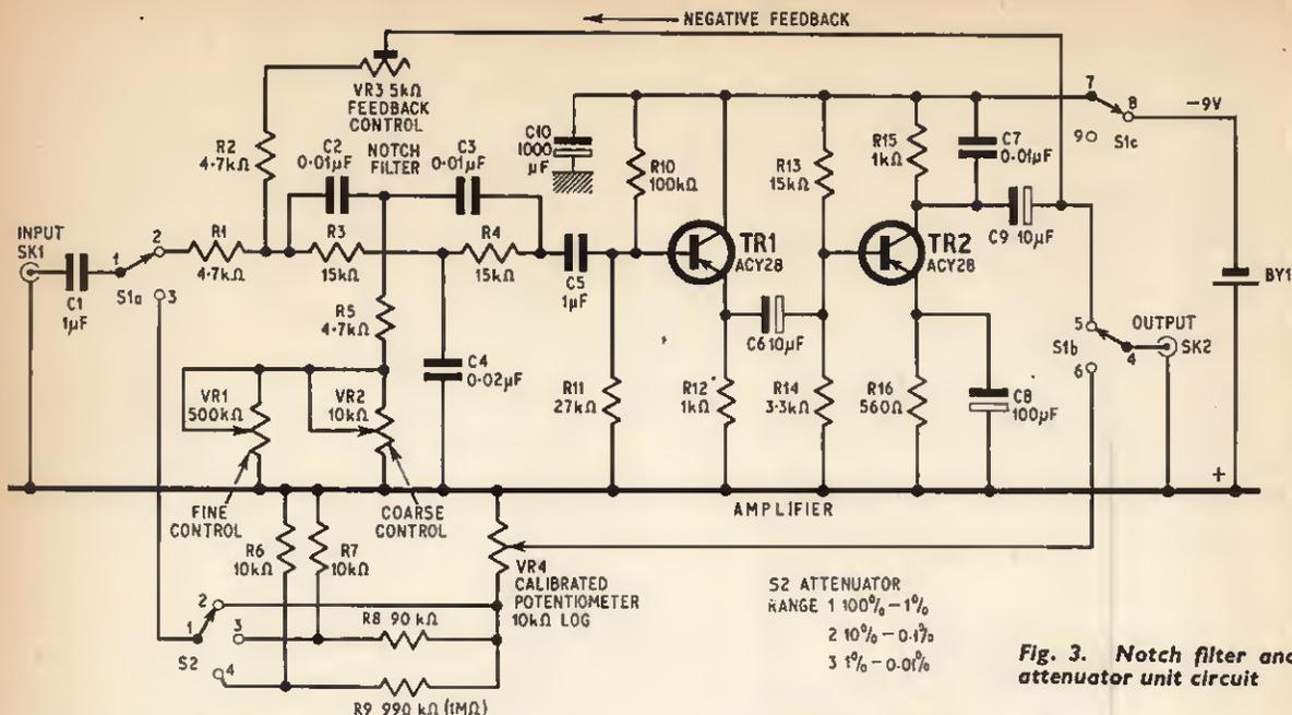
Fig. 3. Notch filter and attenuator unit circuit
