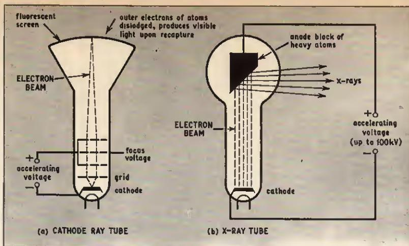
Fig. 1.2. Comparison of a Cathode ray Tube and an X-Ray Tube. In the cathode ray tube (a), electrons are accelerated with relatively low voltages and then impart a fraction of their energy (a few eV) to atoms in the fluorescent screen material, thereby dislodging only outermost electrons. When these are recaptured, the binding energy is released as electromagnetic radiation in the visible light spectrum.
