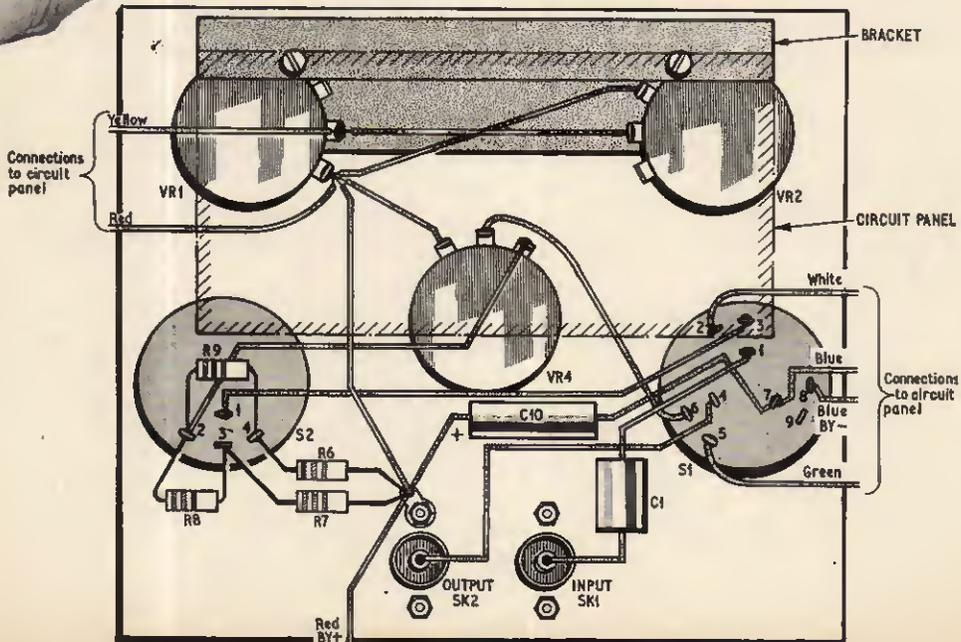
Fig. 6. Front panel controls and wiring
