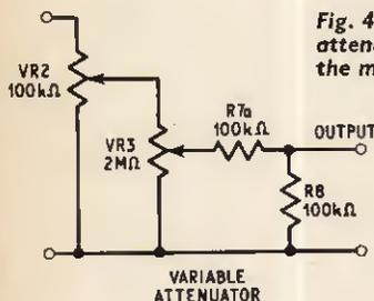
Fig. 4 (left). Simple variable attenuator used when testing the module
