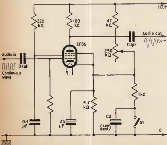
Fig. 2a. Sound decay circuit using a single valve
