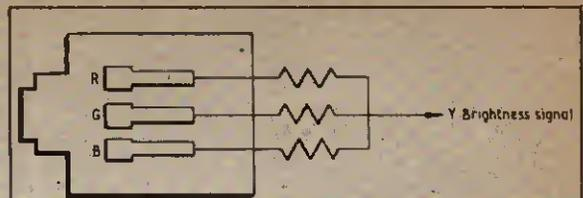
Fig. 2a. Three basic colour units in the camera
