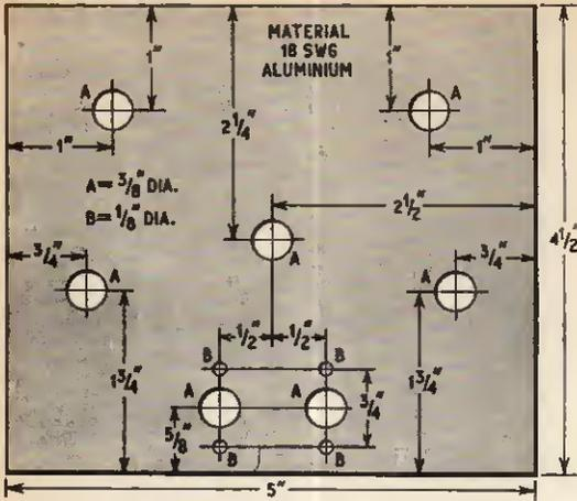
Fig. 4. Front panel drilling details
