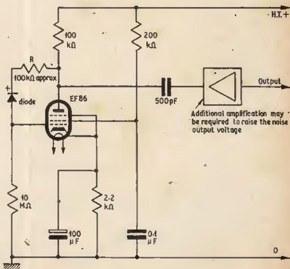
Fig. 7. White noise generator. Resistor R may need adjustment to produce maximum noise output, which may have to be further amplified. This circuit is unsuitable for adaptation using a transistor
