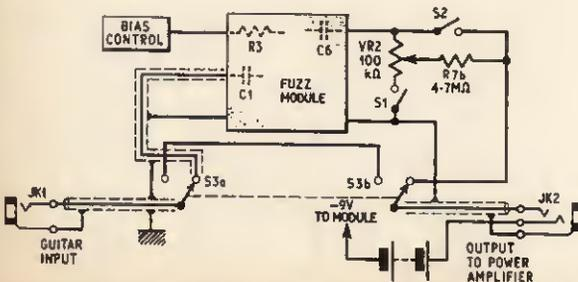
Fig. 7. Circuit diagram of the advanced fuzz box
