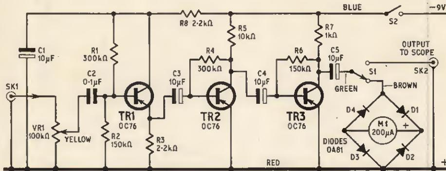
Fig. 9. Detector unit circuit
