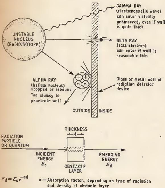
Fig. 1.4. The penetrating power of nuclear radiations
