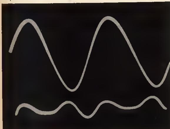
Fig. 13. Oscillograph of sine wave containing 1 per cent distortion. Lower trace shows distortion signal
