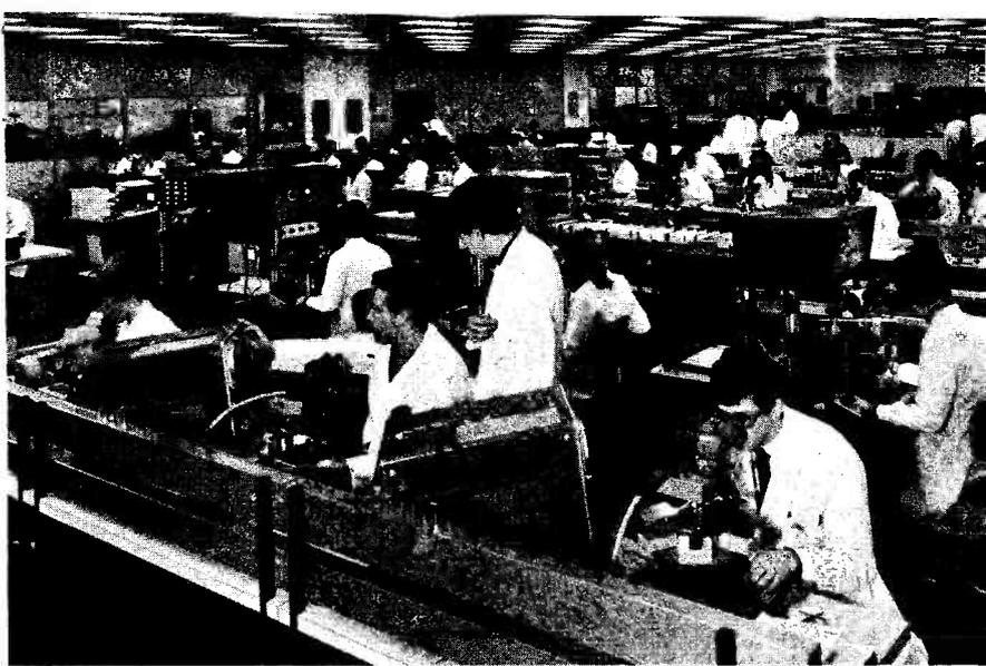
*A general view of the main 6,000 sq ft assembly area. The front row of girls in the photograph are testing circuits before they are assembled into their final packages*
