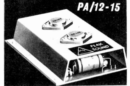
THE PEAK SOUND PA/12-15 (12 watts R.M.S. out into 15Ω) is for the constructor who appreciates both sensible design and genuine power and hi-fi performance. Available built or in kit form. Response 10 Hz – 45 KHz ±0.5 dB Distortion at max. output –0.1% 43 dB neg. feed back. Size 5" x 3 1/2" x 1 1/2". With full instructions. Pre-amp. details available. (P/P for kit or built 2/6)
