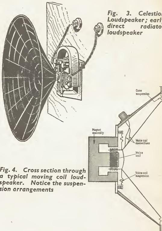
Fig. 4. Cross section through a typical moving coil loudspeaker. Notice the suspension arrangements
