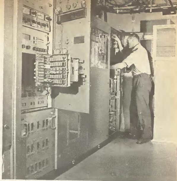
*Part of the transmitter cabin with an operator adjusting the coolant supply for the output travelling wave tube of one of the transmitters. The local control panel in the foreground is open to show the controls for setting up the drive unit*
