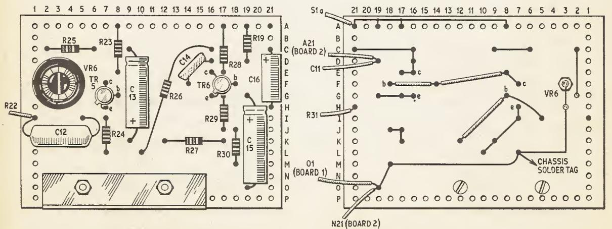
Fig. 4. Component layout and wiring for Board 3, comprising the mixing amplifier
