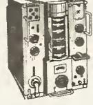
Just released by the Ministry. High quality 10 valve receiver manufactured by Murphy. Coverage in 5 bands 650kc/s - 30Mc/s, 1/1F 500kc/s. Incorporates 2 R.F. and 3 I.F. stages, band-pass filter, noise limiter, crystal controlled B.F.O., calibrator 1/F, output, etc. Built-in speaker, output for phones. Operation 150/230V a.c. Size 19 1/2 x 13 1/2 x 16in. Weight 114lb. Offered in good working condition. £22.10.0. Carr. 30/-.
