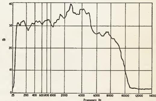
Fig. 6. Frequency response to be expected with a typical 10in moving coil loudspeaker mounted on an infinite baffle
