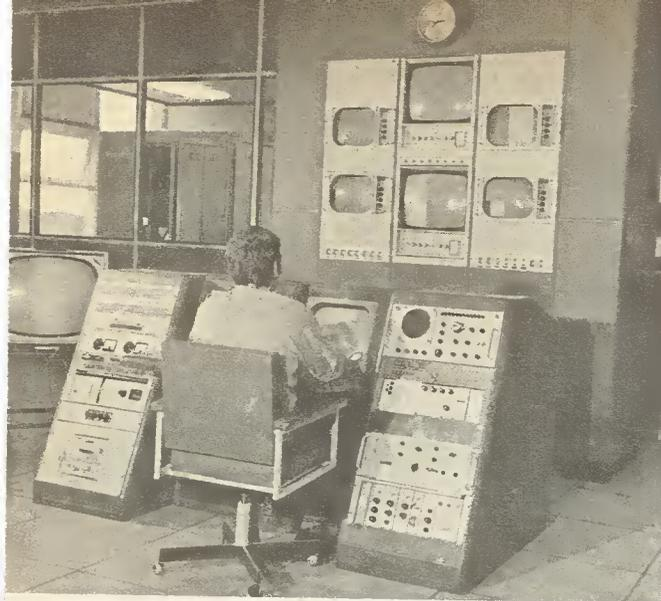
*Comprehensive testing and monitoring facilities for both colour and black and white television signals is provided at this control console*
