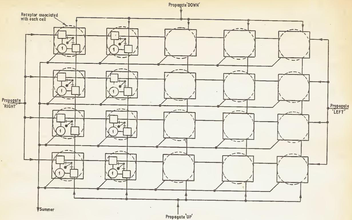
Fig. 6.10a. Basic principles of the fixed matrix system. Note: separate hold, trigger, and reset lines not shown
