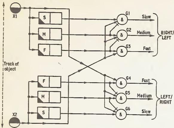
Fig. 6.2. Property detector for judging direction and speed of passing objects
