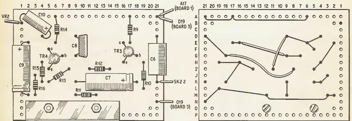
Fig. 3. Component layout and wiring for Board 2, comprising the pre-amplifier for Microphone 2
