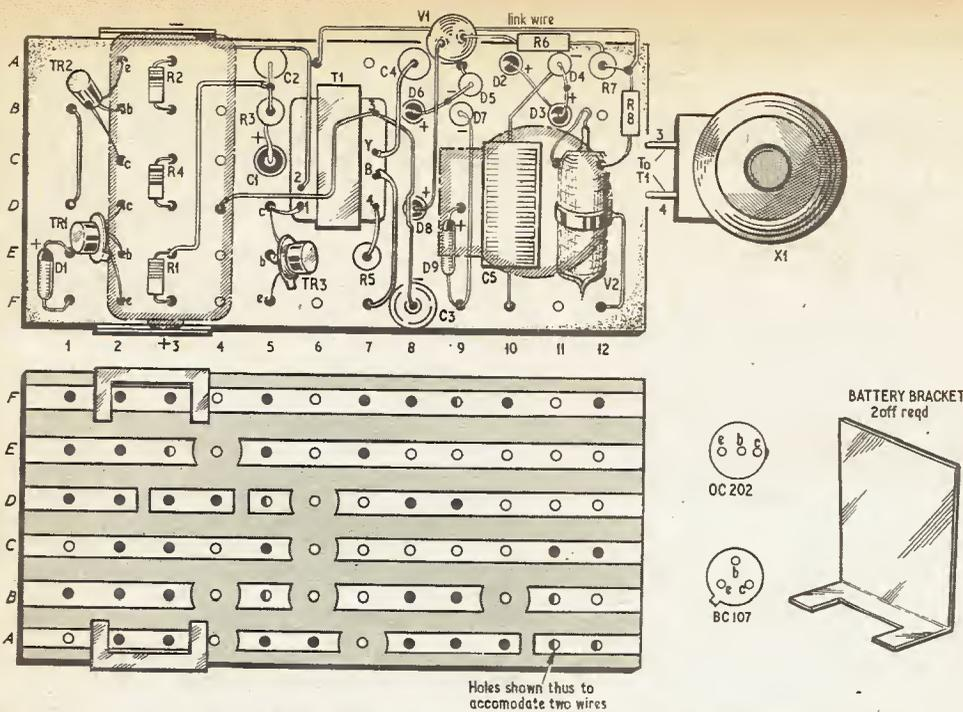
Fig. 3. Layout and wiring of the board. The battery and microphone are positioned as indicated by the dotted lines, see text. The battery clips are made from strips of brass or similar material
