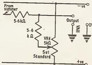
Fig. 6.6 Standardisation circuit for use in conjunction with the device shown in Fig. 6.5
