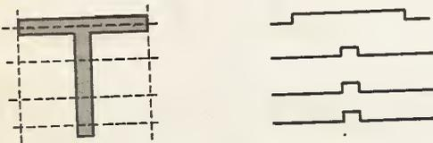
Fig. 6.8. A scanning process used in some character recognition systems
