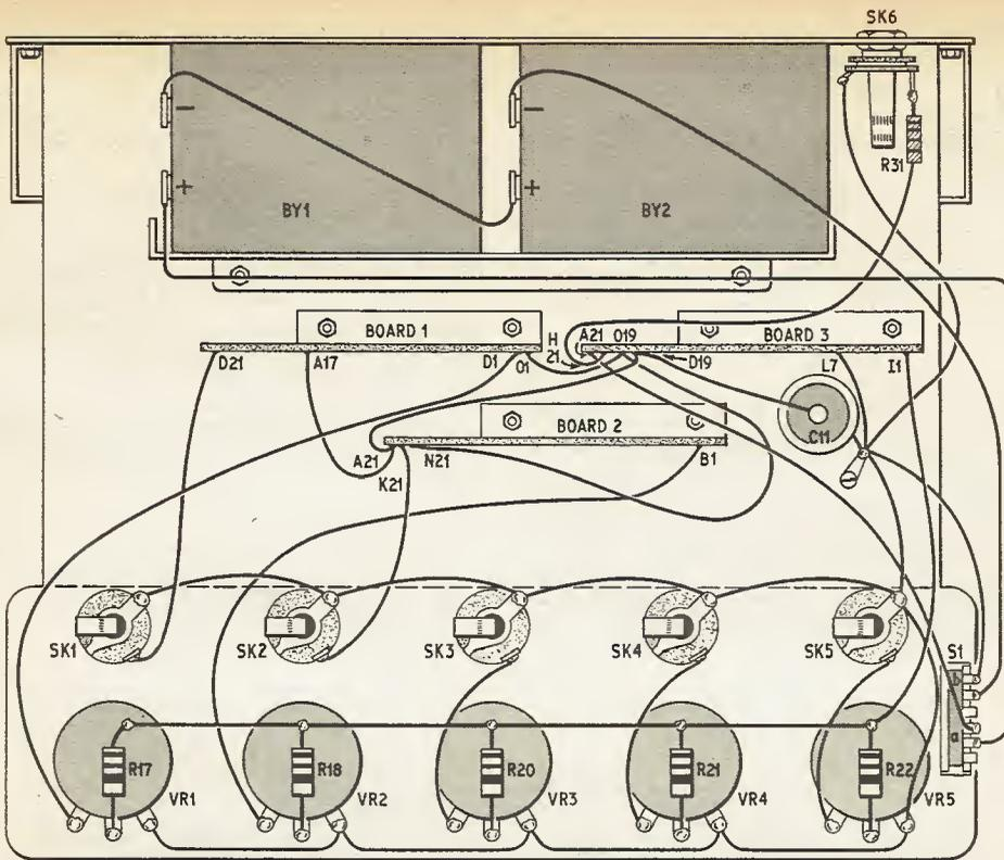
Fig. 8. Wiring of microphone mixer unit
