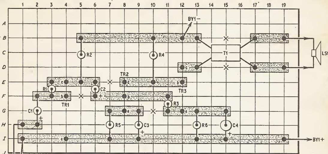
Fig. 2. Use squared paper to draw plan of component layout based on layout of circuit. External components VR1, LSI, and BY1 are connected by flying leads to the board. Collector is wire nearest spot; base is centre wire on all transistors
