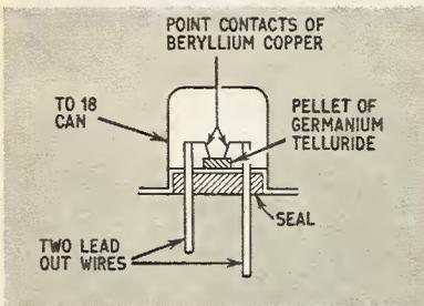
Fig. 1 Structure of the germanium telluride device of 1964
