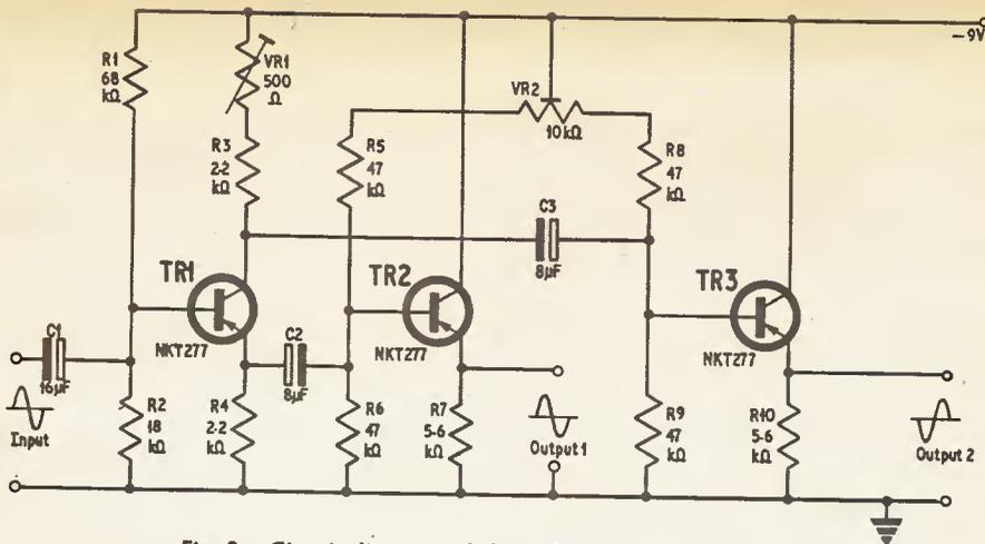
Fig. 3. Circuit diagram of the balanced phase splitter
