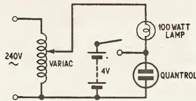
Fig. 2 Prototype test rig for the Quantrol device using a 4V battery for the high current pulse
