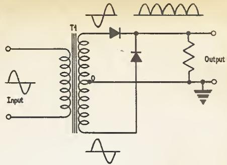
Fig. 5. Principle of the frequency doubler
