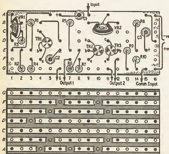
Fig. 4. Layout and wiring of components on the Veroboard
