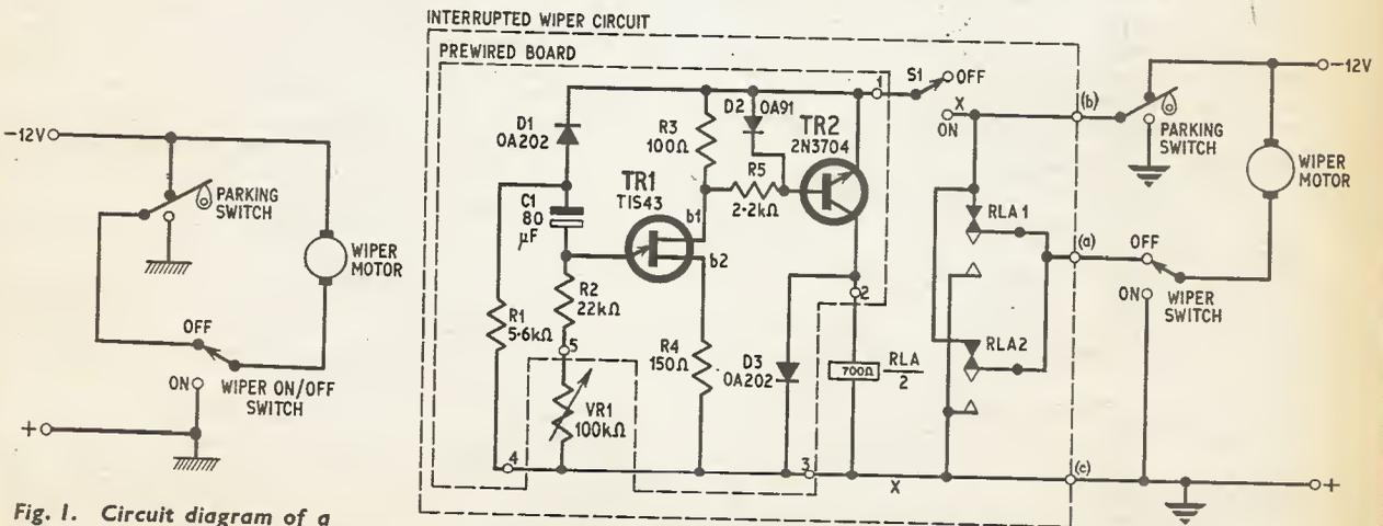
Fig. 1. Circuit diagram of a modern screenwiper using a permanent magnet motor
