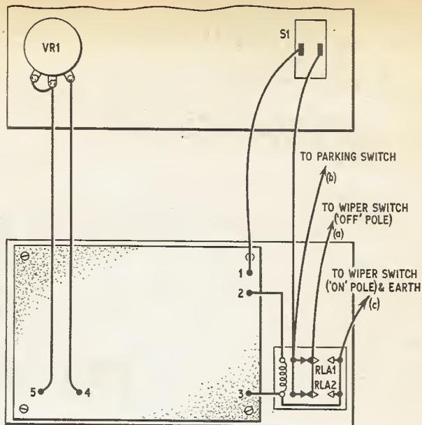
Fig. 4. Layout and wiring of the components mounted in the diecast case; all interconnections should be made using plastic covered wire. S1 and VR1 are positioned to avoid contact with the relay and component board when the front of the case is screwed down
