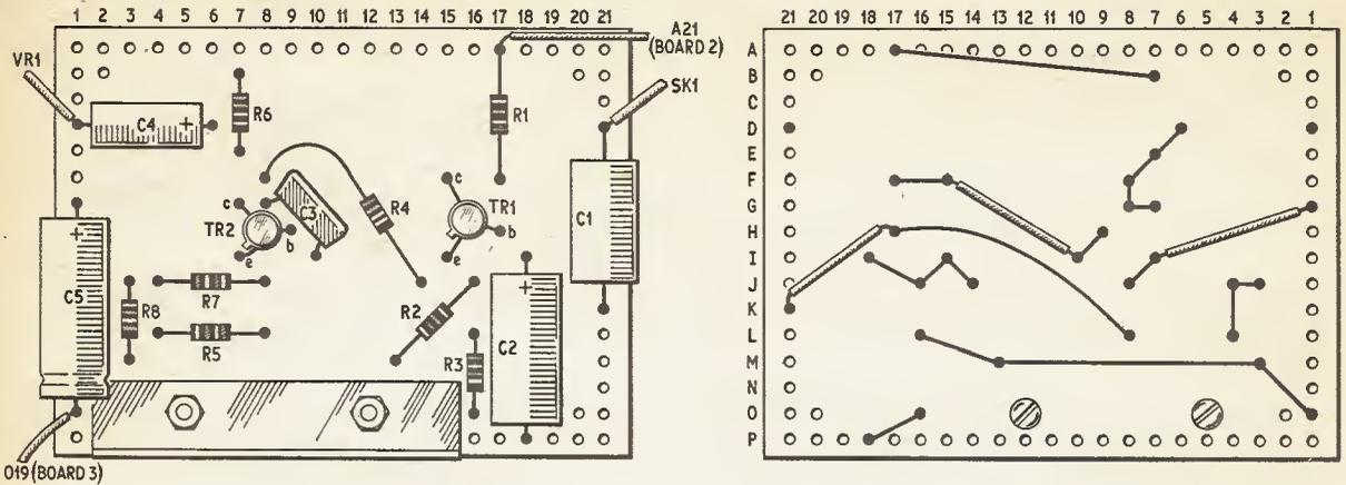
Fig. 2. Component layout and wiring for Board 1, comprising the pre-amplifier for Microphone 1
