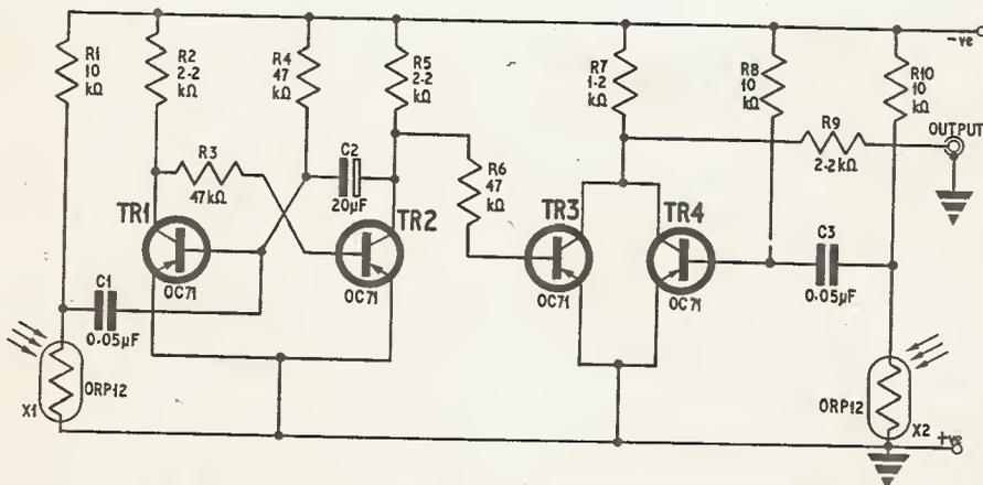
Fig. 6.3. Circuit diagram for property detector outlined in Fig. 6.1
