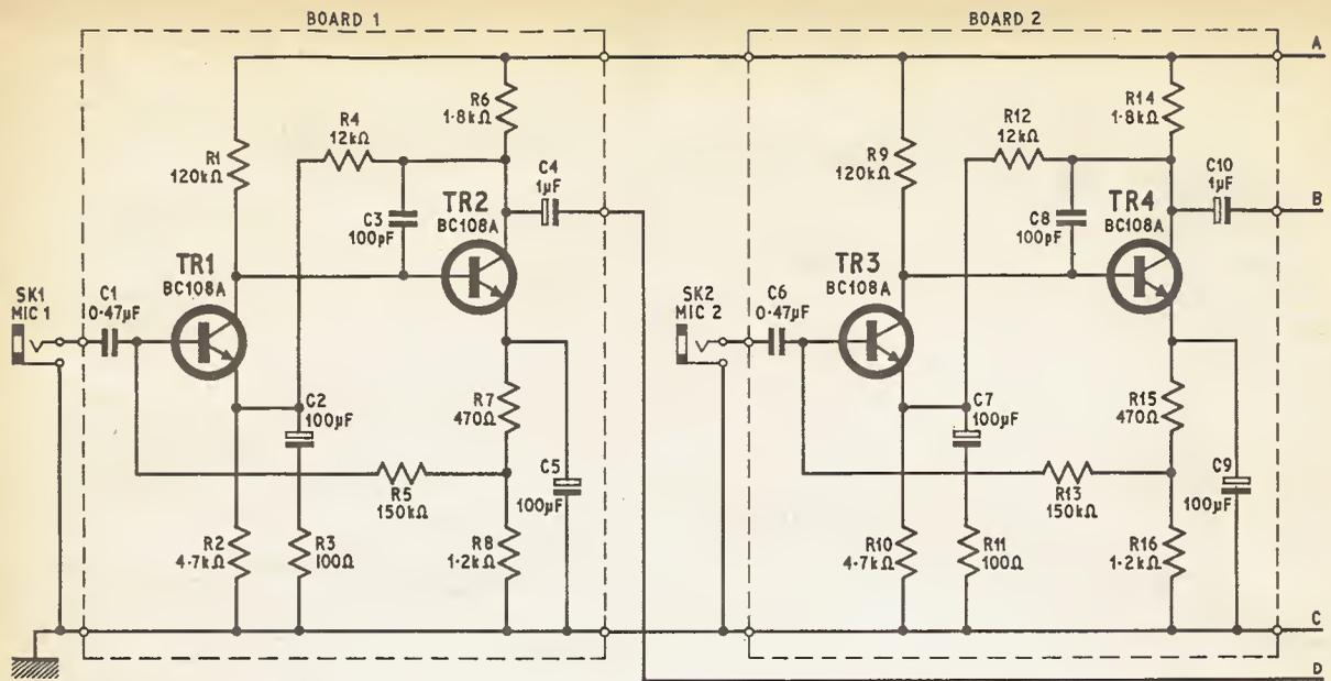
Fig. 1. Circuit diagram of mixer unit. Amplifier sub-assemblies are contained within the dashed lines
