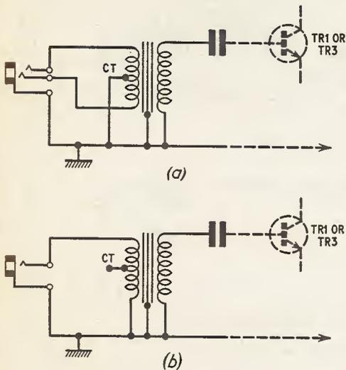
Fig. 9. Microphone transformer connections for (a) balanced input; (b) unbalanced input
