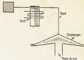
Fig. 3. Celestion Loudspeaker; early direct radiator loudspeaker
