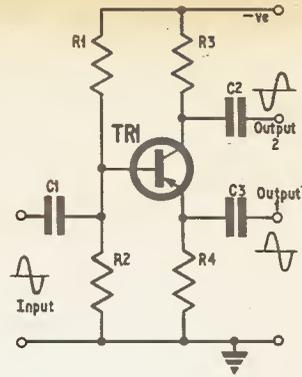
Fig. 1. The balanced inverter phase splitter
