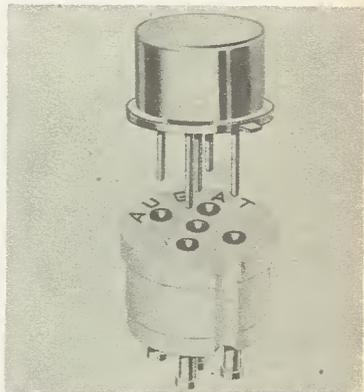
Augat 5-pin TO5 relay socket from Electrosil
