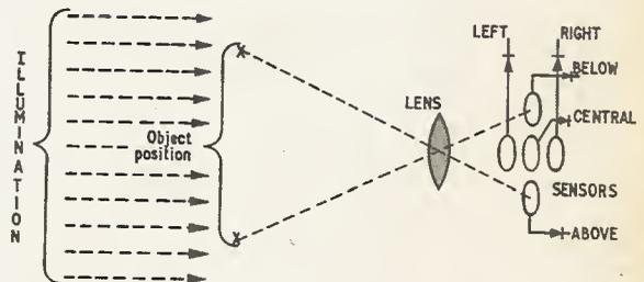
Fig. 6.4. Position detector employing a number of photo receptors. Each sensor delivers an output "1" if the source of illumination is obscured by an object
