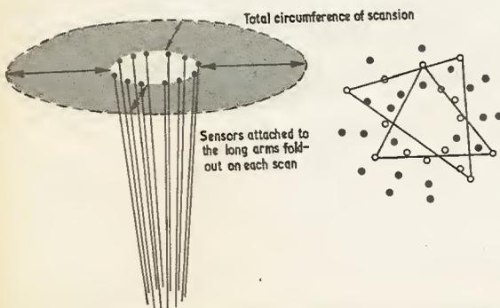
Fig. 6.9. A circular scan system used by one type of machine designed to recognise line drawings (left) pulse pattern when scanning a triangle
