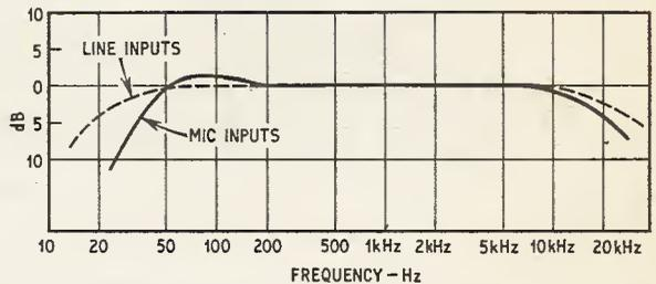
Fig. 10. Frequency response for microphone and line inputs
