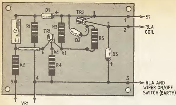
Fig. 3. Wiring diagram of the component-board
