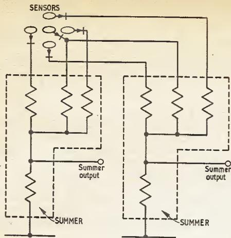
Fig. 6.5. Device for determining length of passing object
