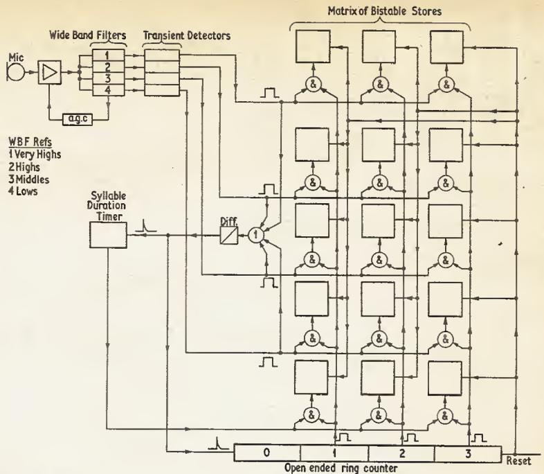
Fig. 6.11. A possible system designed for simple word recognition
