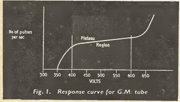
Fig. 1. Response curve for G.M. tube
