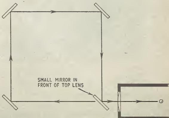
Fig. 1d. Mirrors arranged to enclose an area
