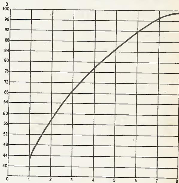
Fig. 3. Graph of  $Q$  against frequency for a coil of 510 turns of 40 s.w.g. wound on an FX 2236 ferrox core
