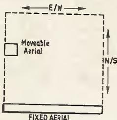
Fig. 3. An example of aperture synthesis such as was used in early Cambridge work
