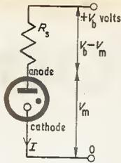
Fig. 1.1. Basic circuit for operating a cold cathode tube
