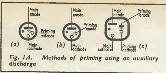
at very high speeds. One of the most common methods of priming involves the use of an auxiliary priming discharge. The latter generates ions which diffuse to all parts of the tube.
