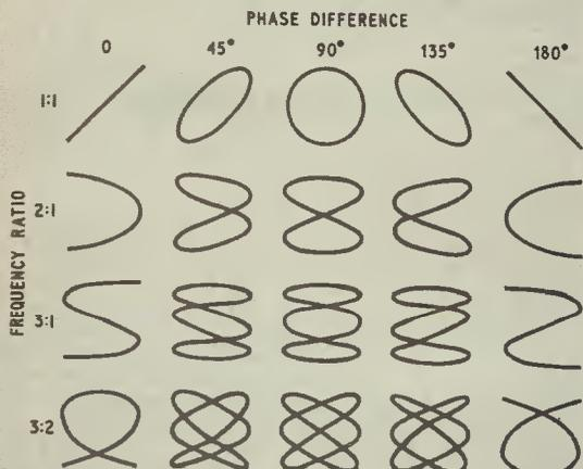
Comparison of cycloid patterns with Lissajous figures for certain frequency ratios. Note that the shapes of both forms of figure depends on the phases of the input voltages, frequency and magnitude
