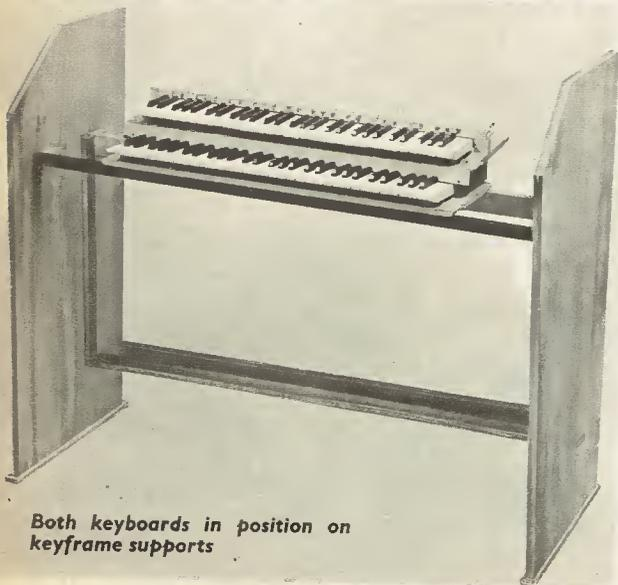
Both keyboards in position on keyframe supports
