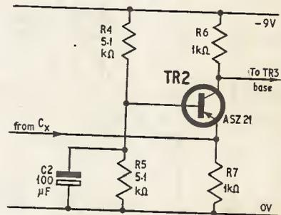
Fig. 8. Alternative grounded base stage used to reduce gain in the two stage unit
