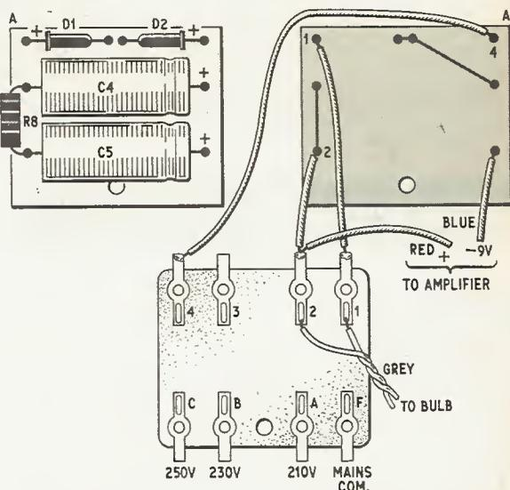
Fig. 5. Component layout and wiring of the power supply
