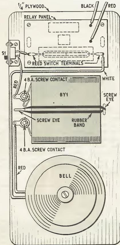
Fig. 9. Details of relay and alarm bell unit
