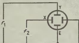
Fig. 1. Simple method of displaying Lissajous figures on an oscilloscope connecting to the X and Y plates
