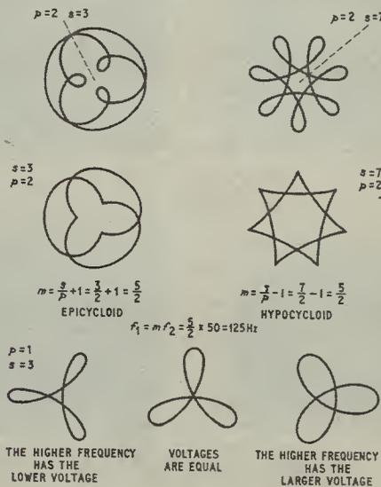
Fig. 11. Cycloid patterns of various frequency ratios.
