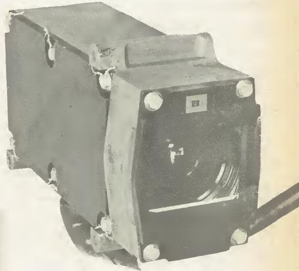
Three of these cameras have been fitted within various small spaces available in engine nacelles to enable possible in-flight icing conditions to be observed and recorded. Special optical devices have been engineered to give the necessary viewing angles required in the confined spaces available.
