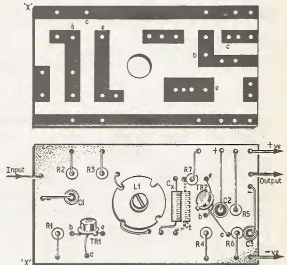
Fig. 5. Layout and wiring diagram of the printed circuit board for one complete tone filter capacitor. Capacitor  $C_x$  may be needed if two units are used in series—see text
