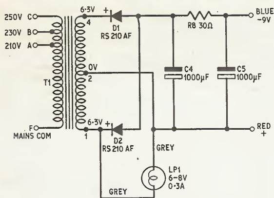
Fig. 4. Circuit diagram of the power supply
