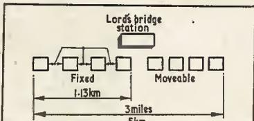
Fig. 1. Layout of the three mile telescope
