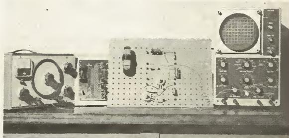
The oscilloscope is set up with an a.f. signal generator and phase splitting circuit for displaying cycloids
