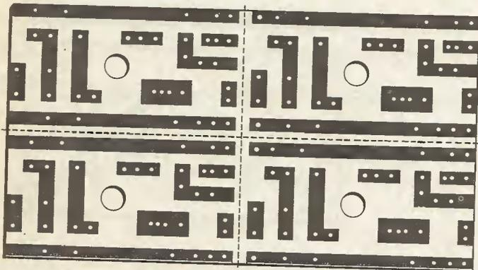
Fig. 7. Printed circuit board layout for four tone filter circuits
