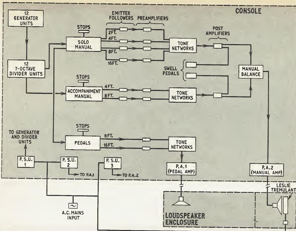
Fig. 1.1. Block diagram of the complete organ
