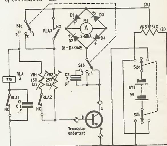
Fig. 1. Circuit diagram of the transistor checker
