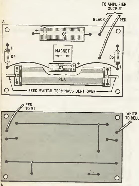
Fig. 7. Component layout and wiring for the relay board
