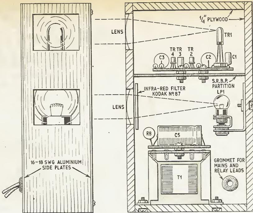
Fig. 8. Positioning of components inside the lens housing case
