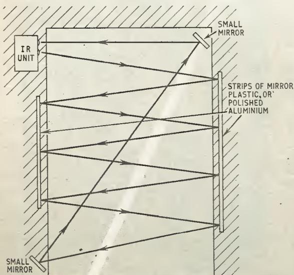
Fig. 1c. Method of lacing beam across doorway
