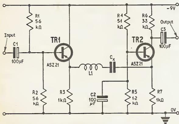
Fig. 1. Circuit diagram of the basic tone filter
