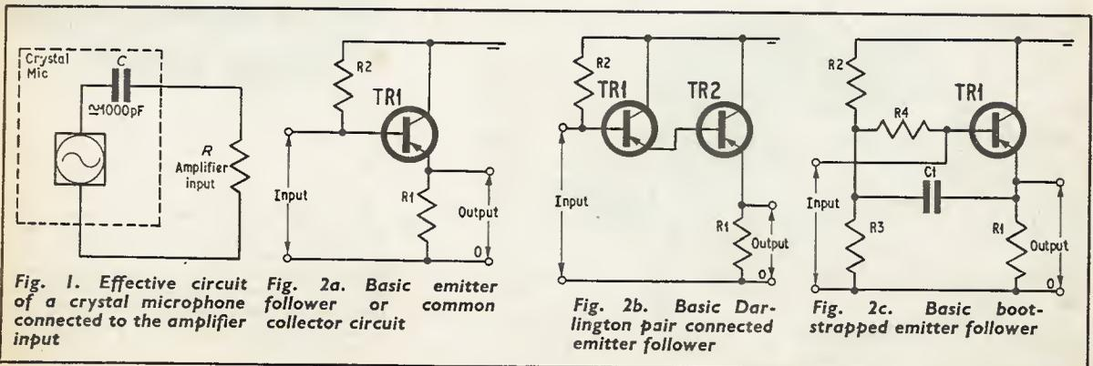
Fig. 1. Effective circuit of a crystal microphone connected to the amplifier input
