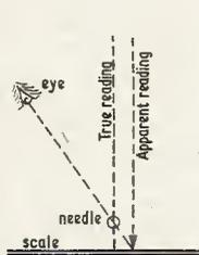
Fig. 2. Parallax error due to incorrect position of the eye in relation to the meter needle
