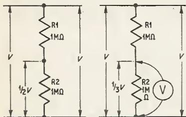
Fig. 1. False readings can be obtained by a poor meter resistance characteristic. (a) The true reading across R2 is equal to half the supply voltage. (b) The meter resistance presents an additional shunt path reducing the voltage across R2
