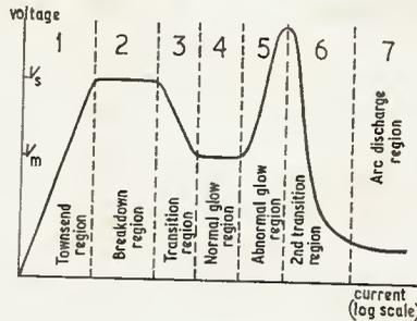
Fig. 1.3. Tubes operating in the normal glow region have a space charge surrounding the cathode
