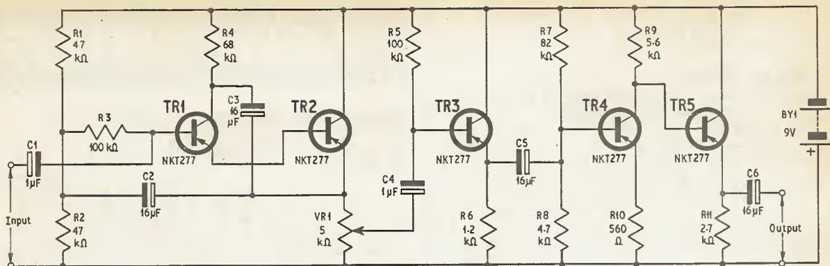
Fig. 3. Circuit diagram of the very high impedance amplifier
