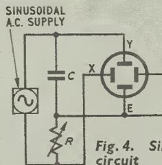
Fig. 4. Simple phase splitting circuit
