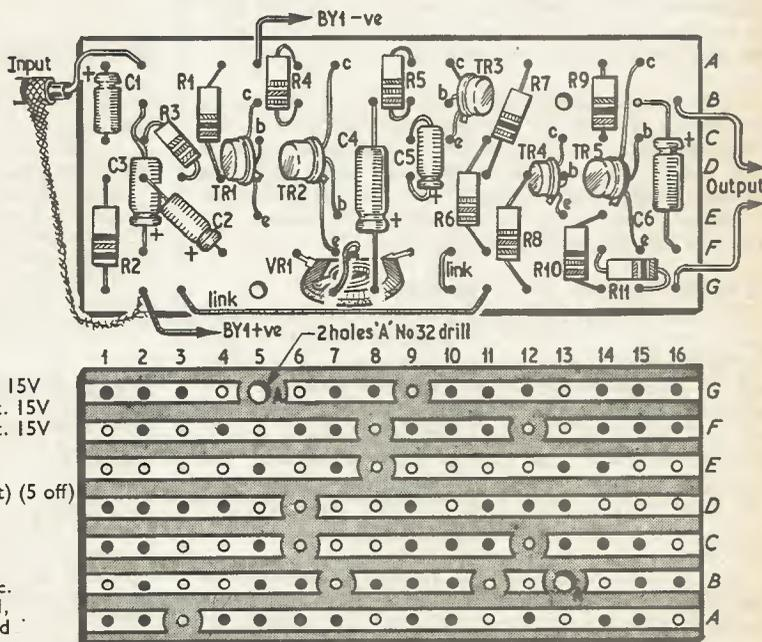
Fig. 4. Layout of components on the board and underside view showing the breaks in the copper strips
