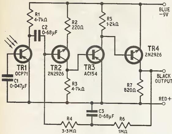
Fig. 2. Circuit diagram of the detector and amplifier stages
