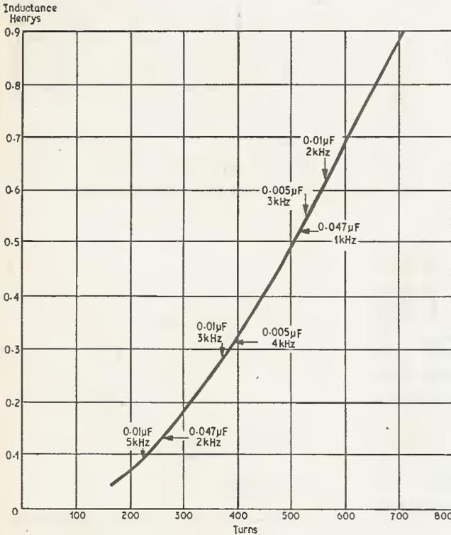
Fig. 4. Graph for determining inductance of coil and value of capacitor  $C_x$ , for various frequencies
