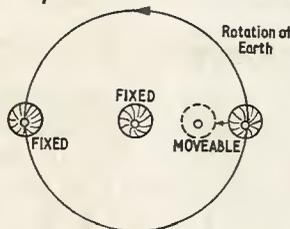
Fig. 2. How the aperture is "filled" by the rotation of the earth and the change of position of the moveable aerial on successive scans of the sky
