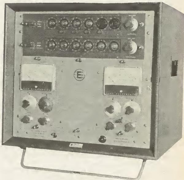
*The Echo N610A Automatic Scaler. This nucleonic counter employs decade stepping tubes for counting, but the two tubes on the upper right are point indicators. The lower group of decade stepping tubes are used for timing and for stopping the count after a preset time*
