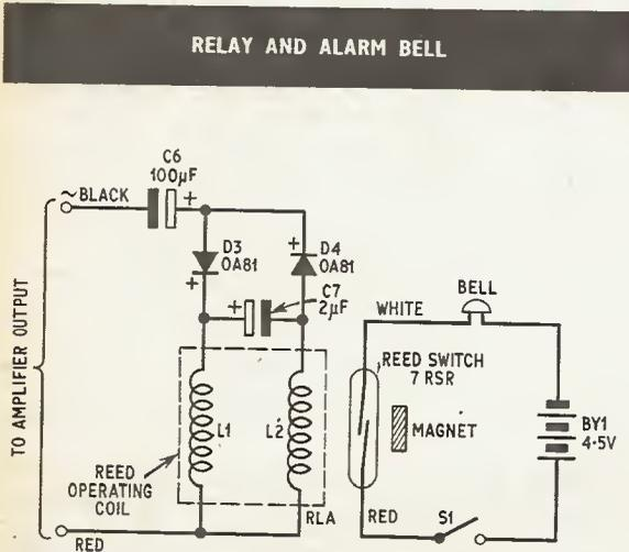
Fig. 6. Circuit diagram for the a.c. latching relay and alarm bell
