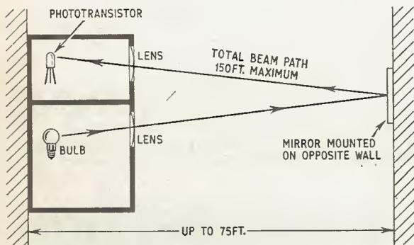
Fig. 1a. Principle of operation of the infra-red alarm
