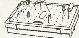
Solderless breadboard panels, for fast reliable component connections. Control Single DeCs. One S-DeC with Control Panel, Jigs and Accessories for solderless connections to controls, etc., with booklet "Projects on S-DeC" giving construction details for a variety of circuits. 29/6. P. & P. 2/6.
