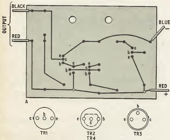
Fig. 3. Component layout and wiring for the amplifier board
