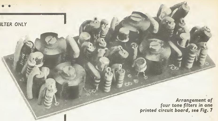
Arrangement of four tone filters in one printed circuit board, see Fig. 7
