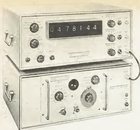
The Marconi TF1417 counter/frequency meter which employs cold cathode tubes to provide a display of the count in digits
