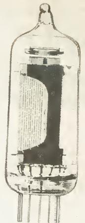
micro-microamp), but when the applied voltage reaches a certain value known as the ignition or striking voltage, the current suddenly increases (typically to some milliamps if the series resistor is of a suitable value). Simultaneously the potential across the tube falls.
