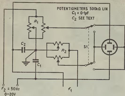
Fig. 7. Circuit for showing epicycloids and hypocycloids
