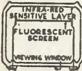
Famous war-time "cat's eye" used for seeing in the dark. This is an infra-red image converter cell with a silver caesium screen which lights up (like a cathode ray tube) when the electrons released by the infra-red strike it. A golden opportunity for some interesting experiments. 7/8 each, post 2/6. Data will be supplied with cells, if requested.
