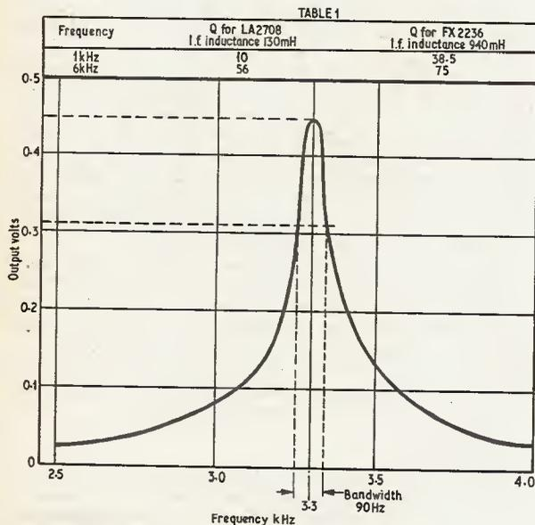
Fig. 2. Frequency response curve of the basic tone filter circuit. Bandwidth, measured at the 3dB down point, is 90Hz at a frequency of 3.3kHz
