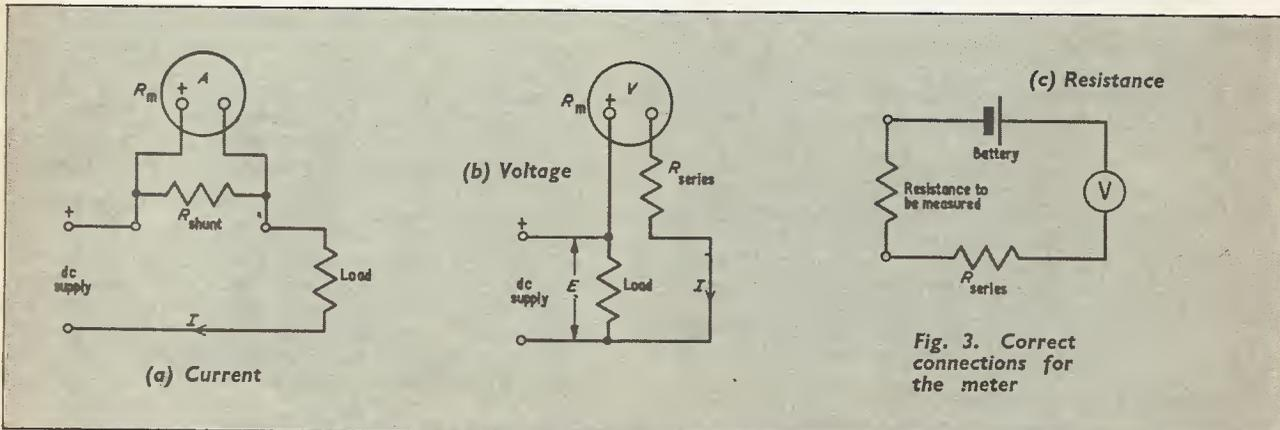
Fig. 3. Correct connections for the meter
