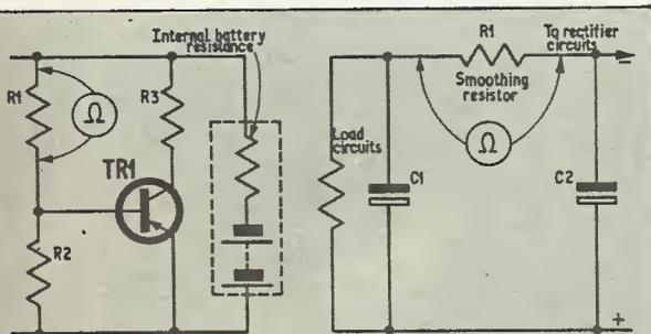
Fig. 4. Misleading errors occur, when measuring resistance in circuit, due to other resistive paths
