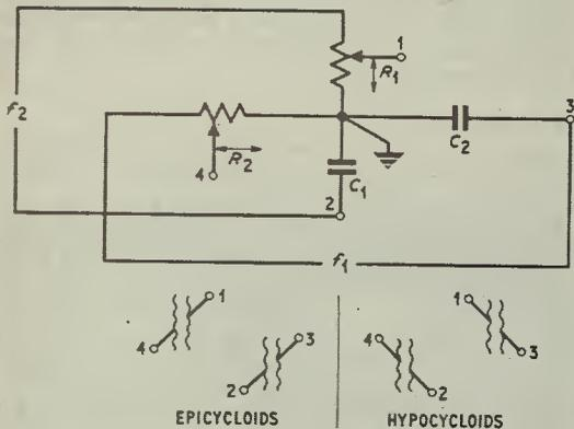
Fig. 5. Basic circuit for cycloid frequency measurement. Here the numbered outputs refer to the oscilloscope connections for horizontal and vertical amplifiers
