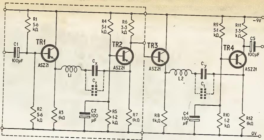
Fig. 6. Circuit diagram of a two stage unit. Area enclosed by the broken line indicates one stage
