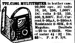
**TFC C1001 MULTIMETER** in leather case. 20,000 opv. AC volts 10, 50, 250, 1,000V. DC volts 5-25, 125, 500, 2,500V. D.C. Current 0-50µA, 0-250mA Resistance 0-60K, 0-6 Megohm. Decibels -20 to +22dB. Size of meter 4 1/4 x 3 1/4 in. 85/- P. & P. 3/6.
