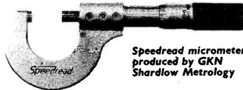
**Speedread micrometer produced by GKN Shardlow Metrology**
