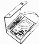
Popular model but with extra scale range 20,000 ohms per volt. 0/5/25/50/250/500/2500V d.c. 0/10/50/100/500/1000V a.c.; 0/50µA, 0/2½/250mA. Resistance 0-6kΩ and 6MΩ. Also dB scales and capacitance. 200H. Price 77/6 pp. 2/-
