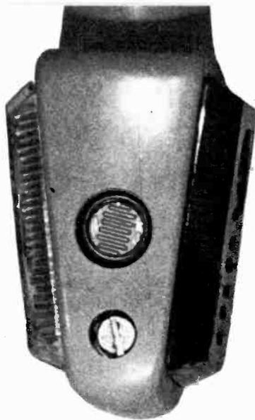
The completed photo electric parking light ; position of X1 can be clearly seen
