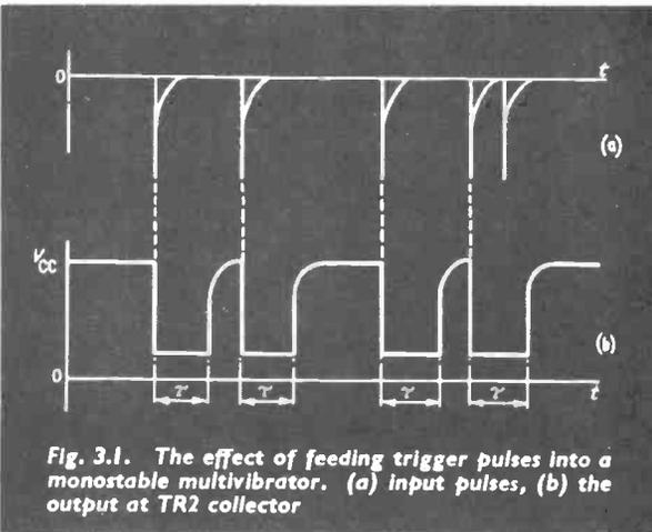
Fig. 3.1. The effect of feeding trigger pulses into a monostable multivibrator. (a) input pulses, (b) the output at TR2 collector
