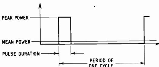
Fig. 1.10. The relationship between peak and mean power
