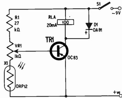
Fig. 2. Relay circuit
