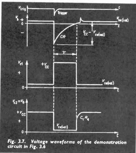
Fig. 3.7. Voltage waveforms of the demonstration circuit in Fig. 3.6
