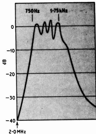
Fig. 5.2. Passband curve using the five stage filter
