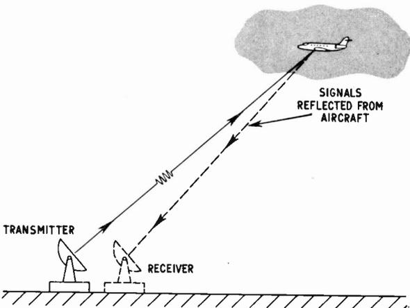
Fig. 1.1. The basic principle of a pulsed radar set
