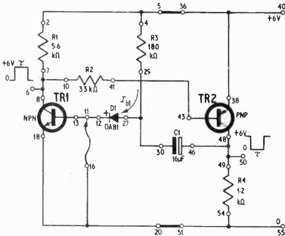
Fig. 3.8 Alternative monostable circuit using one npn and one pnp transistor
