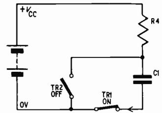
Fig. 3.5. Alternative configuration when TR1 is on and TR2 off
