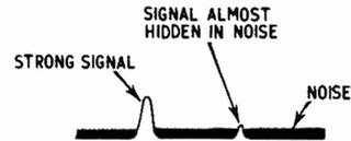
Fig. 1.9. The appearance of noise on an "A" scope
