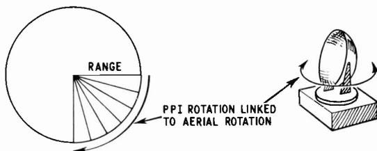
Fig. 1.4. The p.p.i. display principle for indicating both range and bearing
