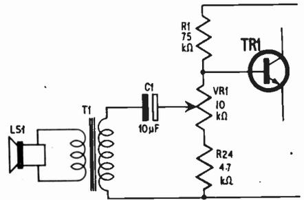
Fig. 5. Circuit for a sensitivity control
