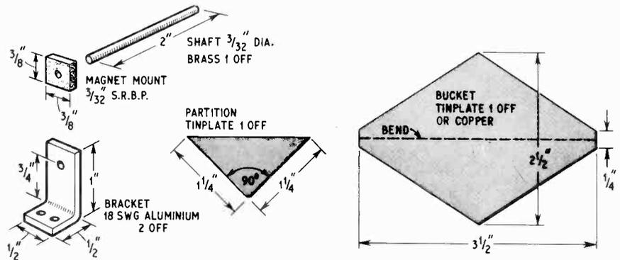
Fig. 5. Construction details of the liquid metering module
