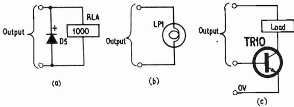
Fig. 4. Output load connections, (a) using relay to switch load, (b) miniature bulb as load, (c) power transistor used to switch load directly
