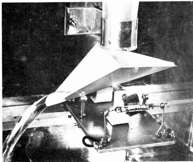
Fig. 2 (left). Low force magnet actuated reed switch operation
