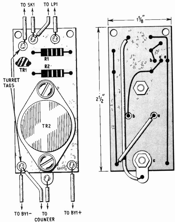
Fig. 6. Amplifier panel, components side and underside
