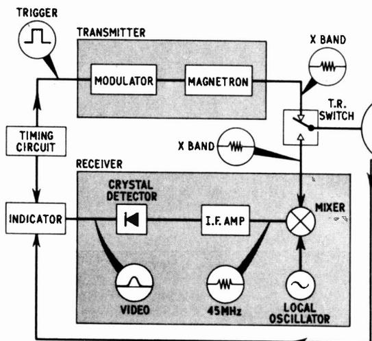
Fig. 1.7. The block diagram for a typical pulsed radar installation
