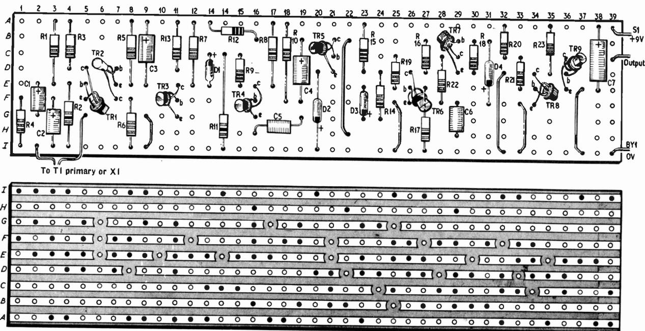
Fig. 3. Veroboard layout and wiring for the sound operated switch
