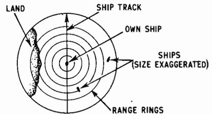
Fig. 1.5. A typical p.p.i. display for a ship
