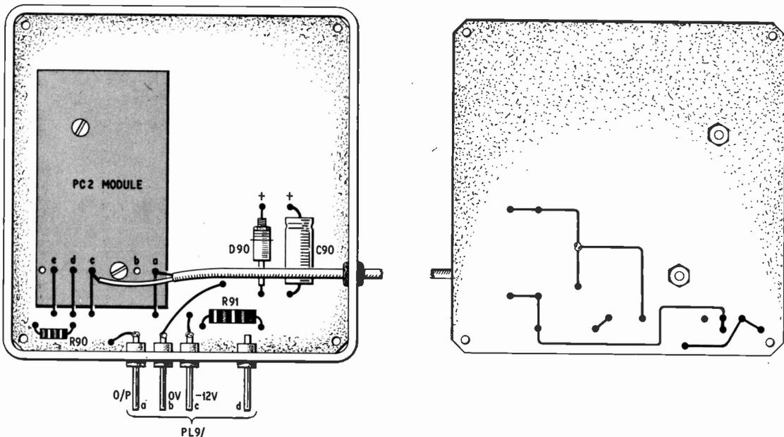
Fig. 5.7. Layout and wiring diagram of the A.F. Unit
