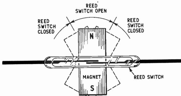
Fig. 3. Counter circuit and reed switch
