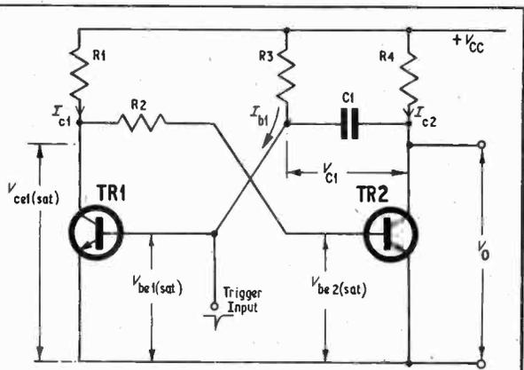
Fig. 3.2. Theoretical circuit of the monostable multivibrator
