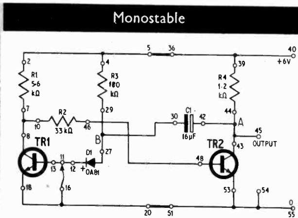
Fig. 3.6. Monostable circuit with hole numbers for S-Dec "breadboard"
