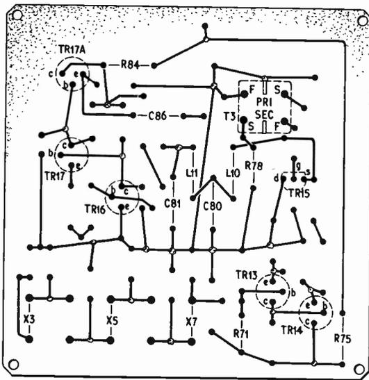
Fig. 5.5. Layout and wiring diagram of the Sideband Filter Unit
