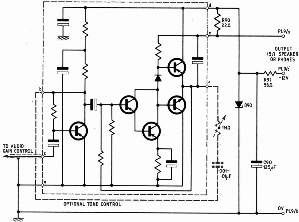
Fig. 5.6. Circuit diagram of the A.F. Unit
