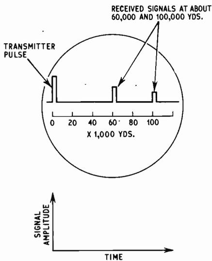
Fig. 1.3. "A" scope display of range
