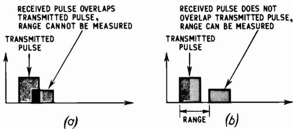
Fig. 1.8. Minimum range depends on pulse width
