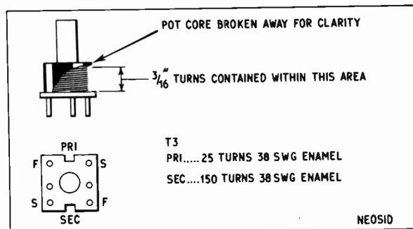
Fig. 5.4. Coil winding details for T3
