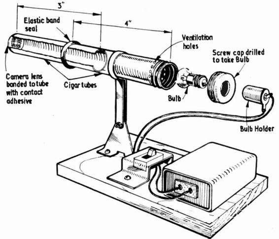
Fig. 1. Light source for light operated switch
