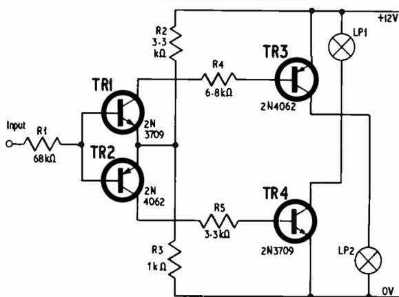
I AM enclosing a circuit diagram for a "0" and "1" logic test-probe which I have recently made. It is designed around a simple gating circuit. The probe operates from a +12V supply and has a threshold voltage of +3V at the input.
