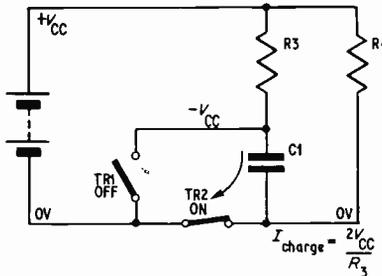
Fig. 3.4 TR1 off and TR2 on
