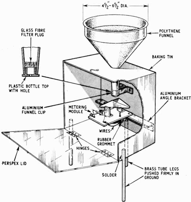
Fig. 4. Suggested layout for rain metering unit
