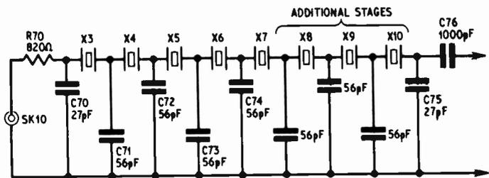
Fig. 5.3. Alternative eight stage crystal filter
