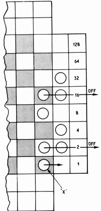
Fig. 4. Arrangement of counters at start of subtraction. Notice the position of the X counter
