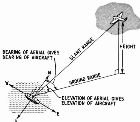
Fig. 1.2. The three information requirements for a radar set
