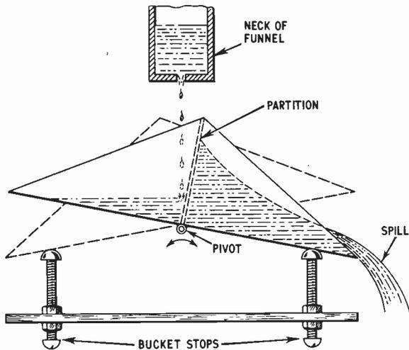
Fig. 1. Sectional view of the "bistable bucket" for metering liquid
