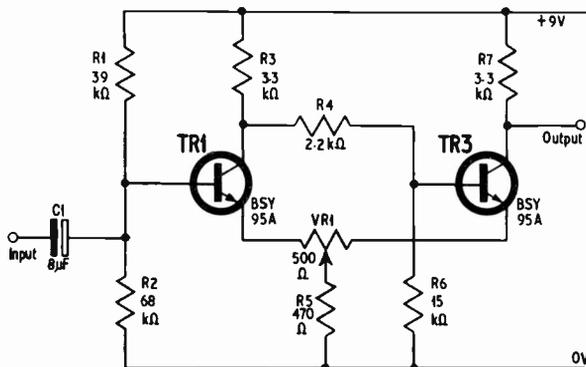
Fig. 1. Circuit diagram of the improved Schmitt trigger
