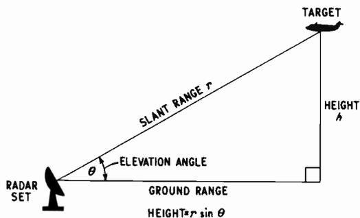
Fig. 1.6. Calculation of height from slant range and elevation information
