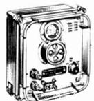
Small portable crystal controlled wavemeter. Size 7" x 7 1/4" x 4". Frequency range 500 Kc/s-10 Mc/s (up to 30 Mc/s on harmonics). Calibrated dial. Power requirements 300 V.D.C. 15mA and 12 V.D.C. 0.3A. Excellent condition. 89/6. Carr. 7/6.
