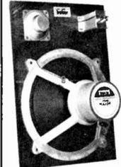
30-14,500 c.p.s., 12in double cone, woofer and tweeter cone together with a BAKER ceramic magnet assembly having a flux density of 14,000 gauss and a total flux of 145,000 Maxwells. Bass resonance 45 c.p.s. Rated 20 watts. Voice coils 3 or 8 or 15 ohms.
