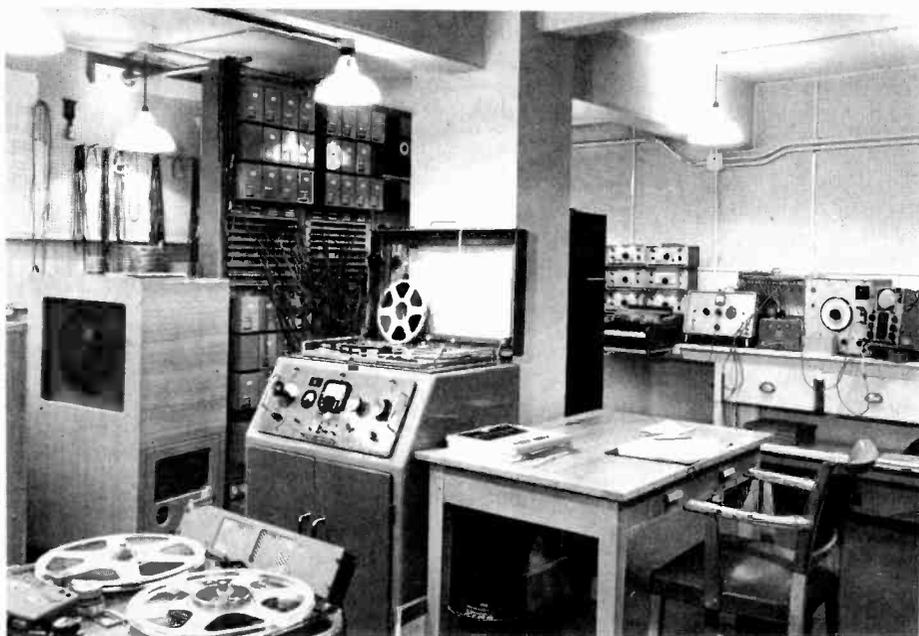
General view of the BBC Radiophonic Workshop. In the background is a bank of signal generators, keying unit and oscilloscope. The EMI BTR/2 tape recorder is in the centre. Behind this are the jackfields associated with the mixing desk (behind TR90 recorder on left)
