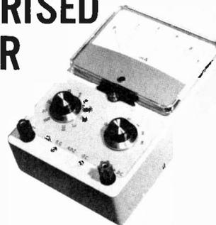
A highly useful and reliable piece of test equipment for the home constructor. The multimeter employs a solid state amplifier to drive a moving coil meter, thus increasing the sensitivity of the meter by up to 100,000 times and at the same time protecting it against overload. The testmeter covers the d.c. voltage range 2mV to 500V f.s.d. and the d.c. current range 200mA to 500mA. An external adapter for a.c. measurements can be added.
