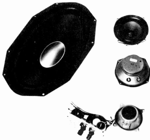
**EMI 215 system incorporating a 14in x 9in elliptical bass unit, two 5in mid-range units, a moulded chassis high frequency unit, and crossover network**
