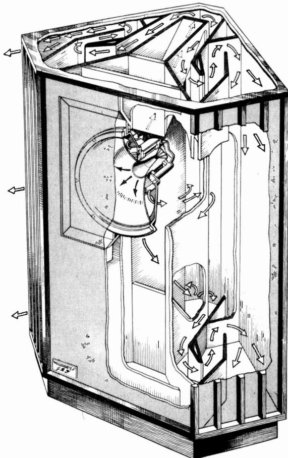
Cutaway view of a Tannoy folded horn enclosure used with a 15in dual concentric unit
