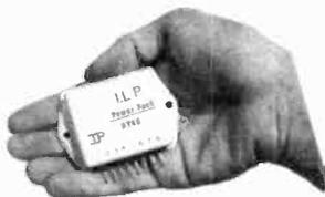
**OUTPUT POWER** British Rating 40 WATTS PEAK, 20 watts RMS continuous.
