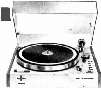
Philips GA202 uses electronic controlled d.c. motor and belt drive
