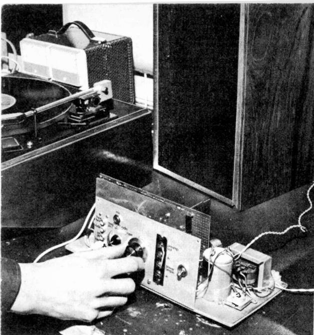
The amplifier being used to check a record deck. One of the many bench applications of the unit
