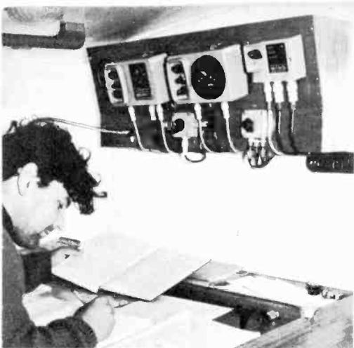
This photo shows Chay Blyth at the chart table of the boat *British Steel* which uses Brooks and Gatehouse electronic instruments, including speed, depth and wind indicators; depth transducer selection switch is at bottom right of the panel. The instrument dials are often duplicated in a waterproof housing on the top of the cabin as shown on the 36ft cruiser racer below
