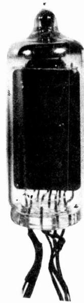
A seven segment incandescent filament indicator tube. Almost any colour filter can be used unlike the cold cathode tubes which are either red or orange
