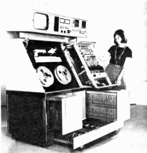
The latest Ampex Video Tape Recorder, type AVR-1
