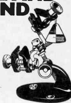
This unique all purpose vice is just like a 'third hand' countless uses for the electronics enthusiast —assembly, soldering, gluing, wiring, drilling, etc. Firm base, positive grip for all shapes of work, with independently adjustable twin jaws.
