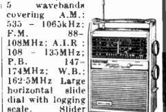
5 wavebands covering A.M.: 535-1065kHz; F.M.: 88-108MHz; A.I.R.: 108-135MHz; P.B.: 147-174MHz; W.B.: 162-5MHz Large horizontal slide dial with logging scale. Slider volume and squelch controls. 7 section telescopic aerial for F.M. and built in ferrite bar for A.M. A.F.C. 3in speaker. Earpiece socket. Green leatherette covered cabinet with metal side panels. Size 152 x 79 x 219mm. Battery/mains operation.
