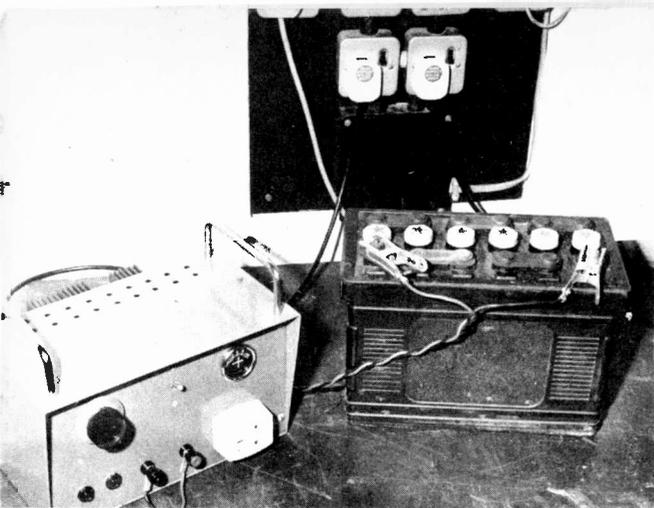
The second prototype equipment boxed in a case and using a circular potentiometer and centre-off control switch
