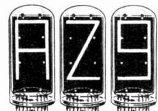
numeric NIXIE tube provides many unique benefits including \* All d.c. operation \* Uniform, continuous line characters of equal height \* Memory with simple solid state drive circuits \* Readability in high ambient light \* 200 footcandle brightness \* Long life with no loss of brightness \* Character height 2 1/2in.
