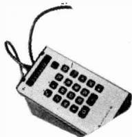
**Advance 88** — a fully user-orientated hand-held machine with 2 independent memories, %,  $\sqrt{\quad}$ , 16 digits. Algebraic logic.
