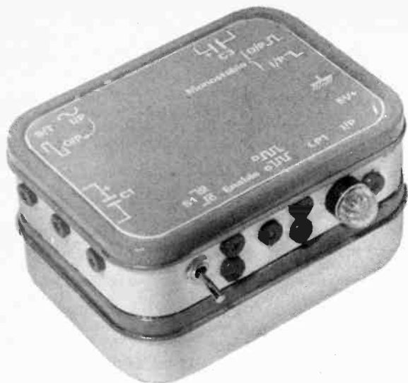
Fig. 6. A simple Schmitt trigger circuit using half of a SN7400N
