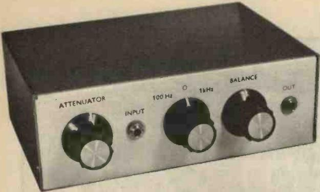
at the position which gives the lowest indication on an oscilloscope or millivolt meter connected to the output of the filter. VR3 should be set at its midway setting during this operation.
