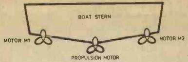
In this circuit an SN7493 four bit binary counter i.c. is used to switch motors on either side of a model boat so giving directional control by bringing about an imbalance in the forces propelling the boat and so turning it. Two motors are used, one on either side of the main propulsion unit (as far from it as possible).
