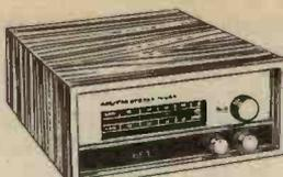
200/240V Mains operated Solid State A/M F/M Stereo Tuner. Covering M.W. A.M. 540-1605 KHz, VHF/FM 88-108 MHz. Built-in Ferrite rod aerial for M.W. Full AFC and AGC on AM and FM. Stereo Beacon Lamp Indicator. Built-in Pre-amps with variable output voltage adjustable by pre-set control. Max o/p Voltage 600 mV RMS into 30K. Simulated teak finish cabinet. Will match almost any amplifier. Size 8 1/2" w. x 4" h. x 9 1/2" d. approx. LIMITED NUMBER ONLY at £28 + £1-30 P. & P.
