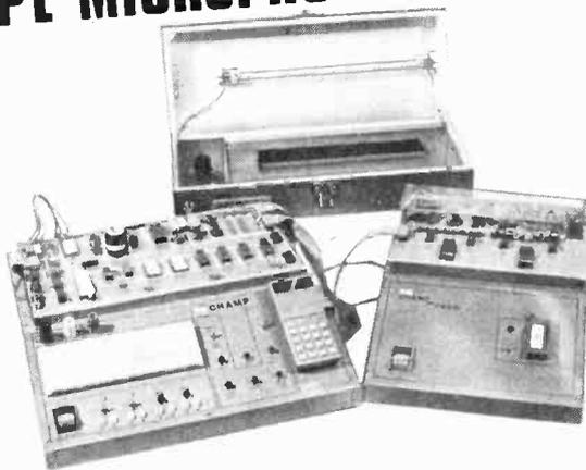
A design which allows the small user and the home constructor to design and develop practical microprocessor based hardware and software for a very small outlay. Comprising three units, Development System, Programmer and UV Eraser, the overall component cost is around £200. The microprocessor used is the Intel 4040, and features include calculator-based hexadecimal keyboard and display, battery-powered CMOS RAM store, and a programmable input/output array.
