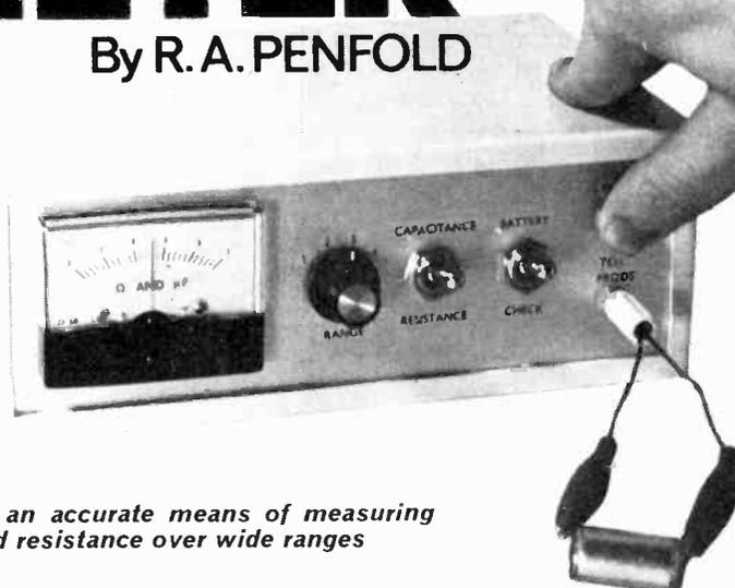
*Fulfils the need for an accurate means of measuring capacitance and resistance over wide ranges*
