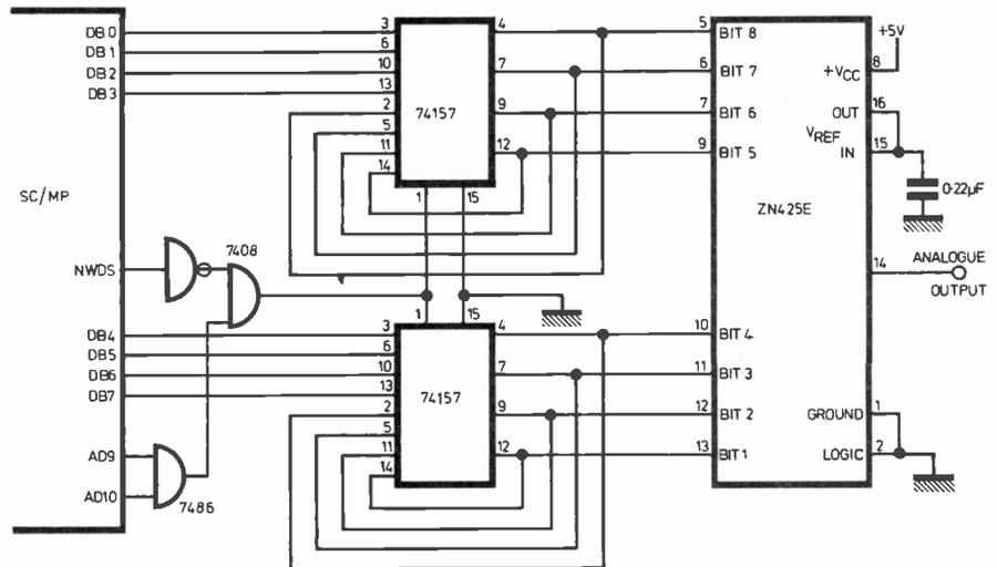
Fig. 1. Circuit showing a latch formed from a pair of 74157 quad 2-input data selectors
