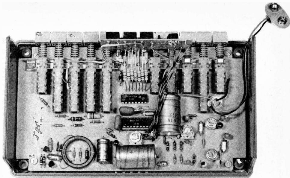
Interior view of the multimeter showing the arrangement of the range switches and segment driver resistors
