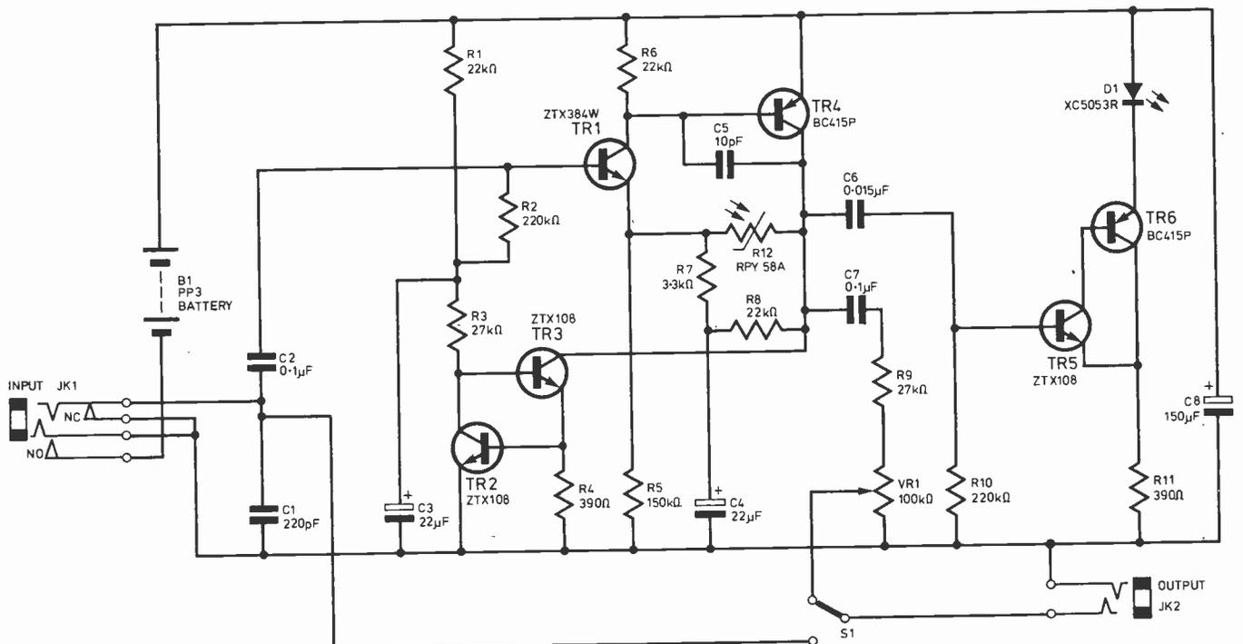
Fig. 5. Circuit diagram of sustain unit
