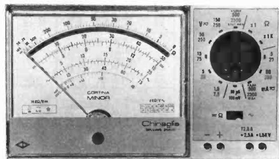
This 33-range instrument uses a Class 1.5 movement with 20kΩ/V d.c. and 4kΩ/V a.c. sensitivity. Accuracy is 2.5% d.c. and 3.5% a.c. Self-powered and pocket-sized, the Minor is guaranteed for 12 months and there is an optional 30kV probe available at £9.70.
