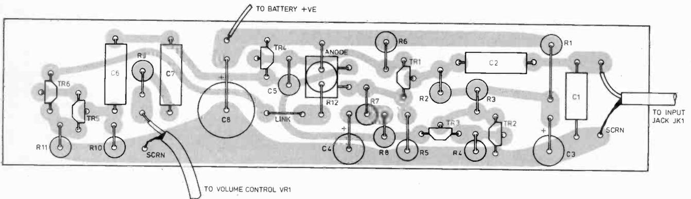
Fig. 7. Component layout and mounting details for D1 and R12 shown above
