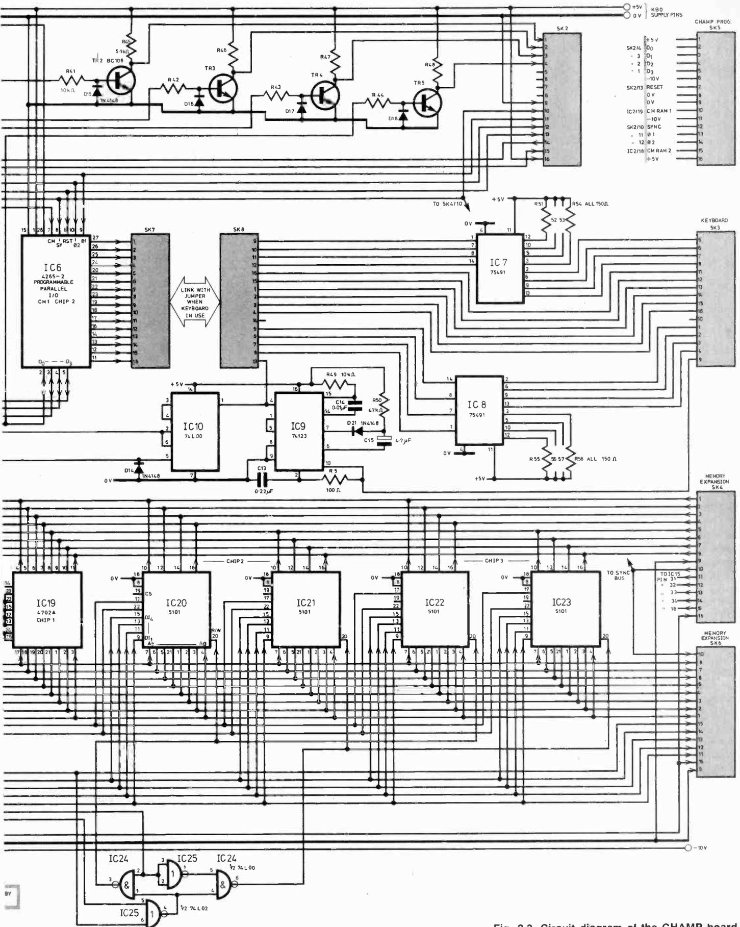
Fig. 2.3. Circuit diagram of the CHAMP board
