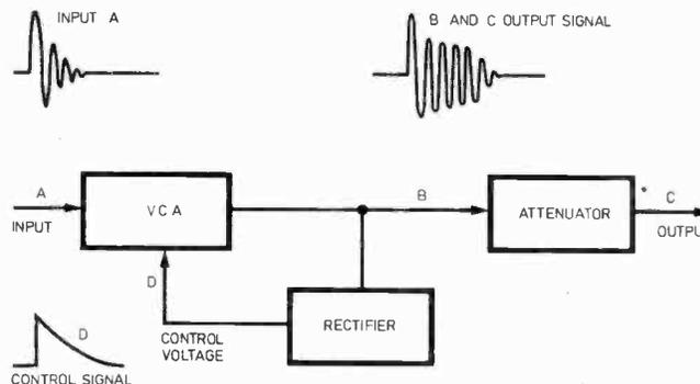
Fig. 2. Block layout for producing a non-distorting sustain unit using a voltage controlled amplifier
