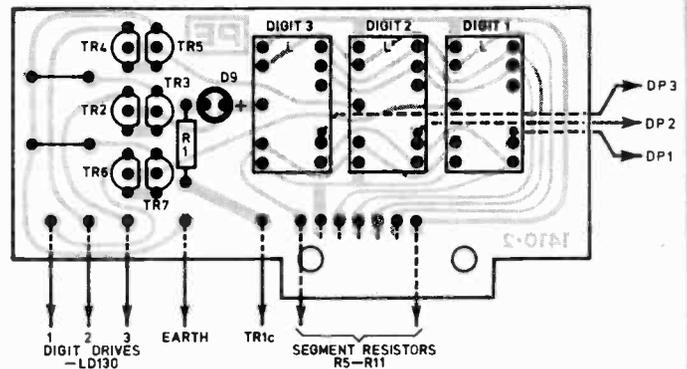
Fig. 7. Display p.c.b. This is mounted on the input socket bracket
