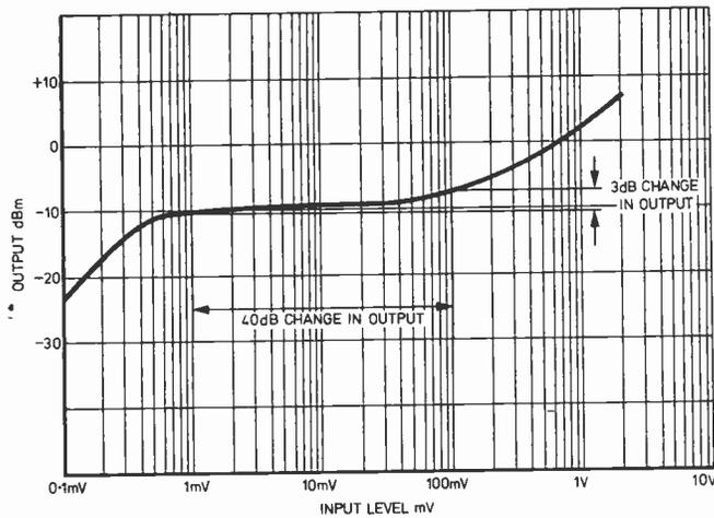
Fig. 3. Output response for different input levels
