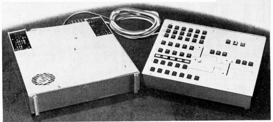
Experimental digital vision mixer developed by the IBA. Input and output signals are coded in linear PCM, at a sampling rate of  $2f_{sc}$ . The mixer offers additive mixing and split-screen wipe facilities
