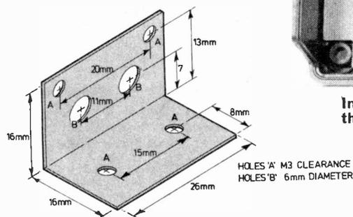
Fig. 9. Dimensions of the aluminium input socket bracket
