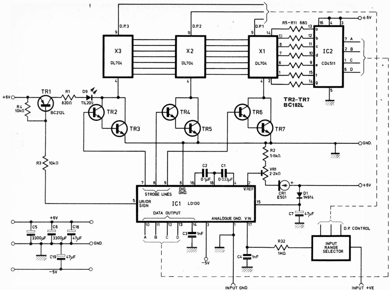
Fig. 2. Circuit diagram of the DMM
