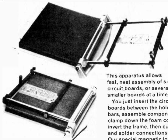
This apparatus allows fast, neat assembly of single circuit boards, or several smaller boards at a time.
