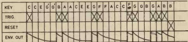
Fig. 12. Demonstrating a simple tune for the sequencer
