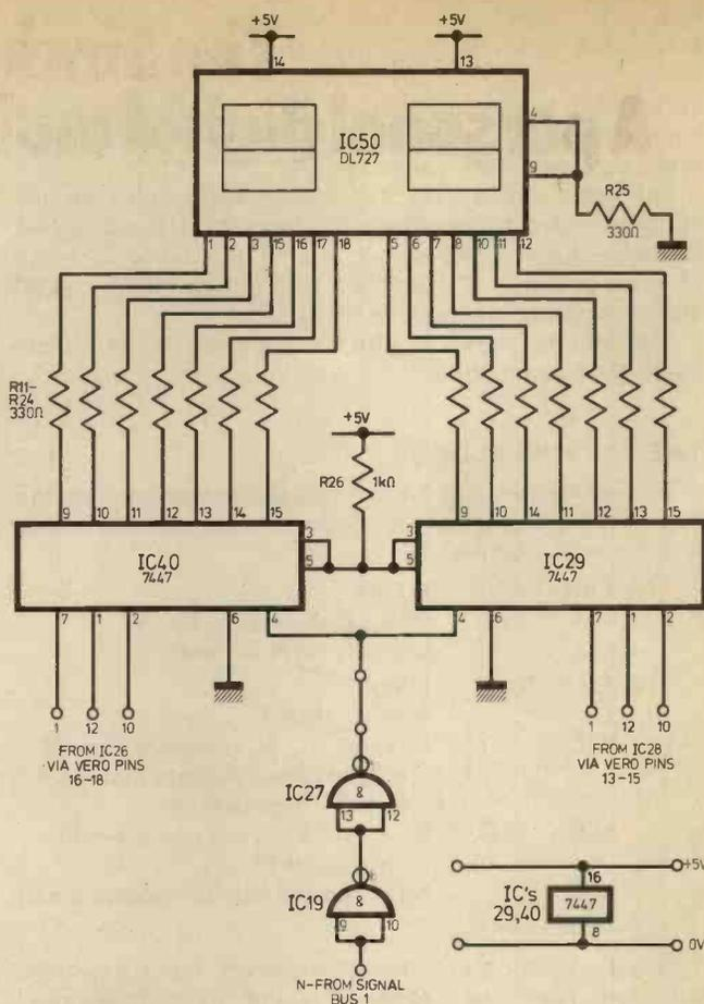
**Fig. 5.5. Circuitry for the display logic**
