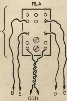
The details shown for wiring up RLA are only correct for the Doram type 72-722-0 relay
