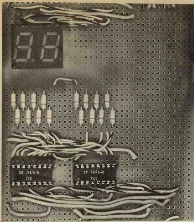
Fig. 5.6. Component layout for the display logic. A photo of the prototype is shown above. For assembly details Fig. 5.3 should be referred to
