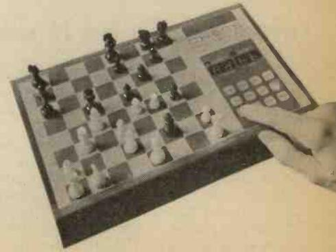
The player enters his move at a keyboard to the right of the chess-board, and the machine gives its reply on a four-digit seven-segment display. The moves are entered as the co-ordinates of the two squares involved (in what is unfortunately the opposite of standard algebraic notation): e.g. FROM 4b TO 4d. The "EN" key then enters the move and the machine replies in about two seconds.
