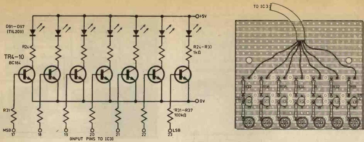
Fig. 9. Circuit of counter and prototype Veroboard layout
