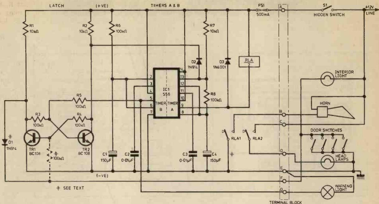
**Fig. 1. Burglar Alarm circuit diagram. For positive earth vehicles, D1 is replaced by a 100kΩ resistor which goes to the base of TR1**
