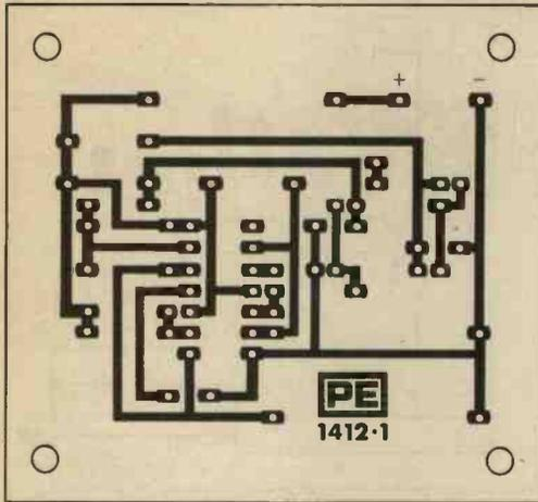
Fig. 3. Printed circuit for Car Burglar Alarm
