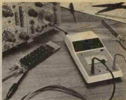
**Sinclair PDM35 digital multimeter**
