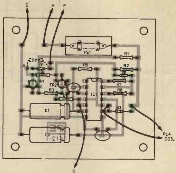
Fig. 4. Component layout of Burglar Alarm board. The spare pad (marked X) is for the "positive earth" modification
