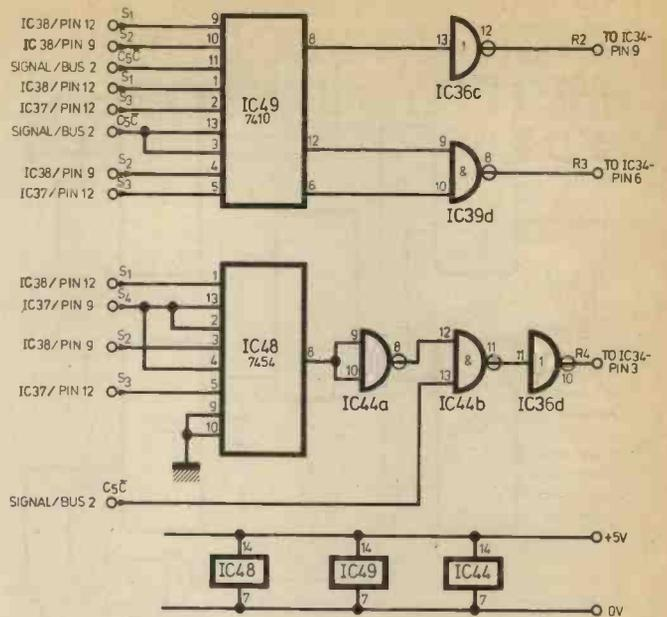
Fig. 5.2. The reset logic circuitry
