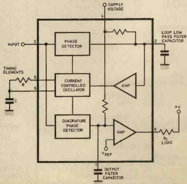
Fig. 2. (a) Block diagram of the NE567 phase locked loop tone-decoder integrated circuit used in the receiver
