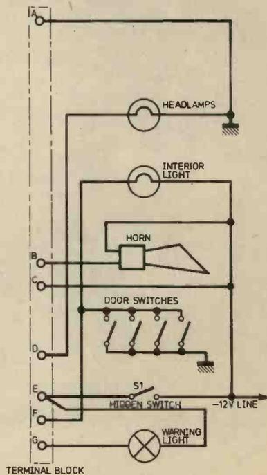
**Fig. 2. External wiring arrangement for positive earth vehicles**
