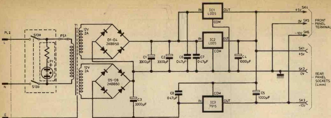
Fig. 4.2. Circuit diagram of CHAMP power supply. Fuse FS1 is only essential if a fused mains plug is not used and should be 2A
