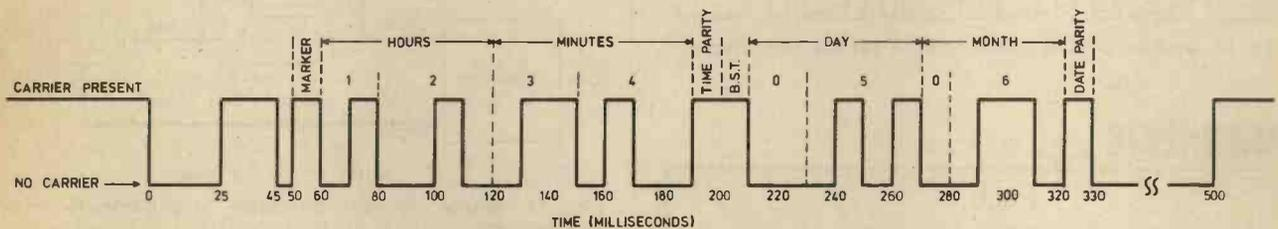
Fig. 1. Format of the encoded time and date information transmitted at the start of each minute
