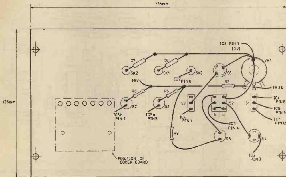
Fig. 10. Interwiring and component layout for control panel
