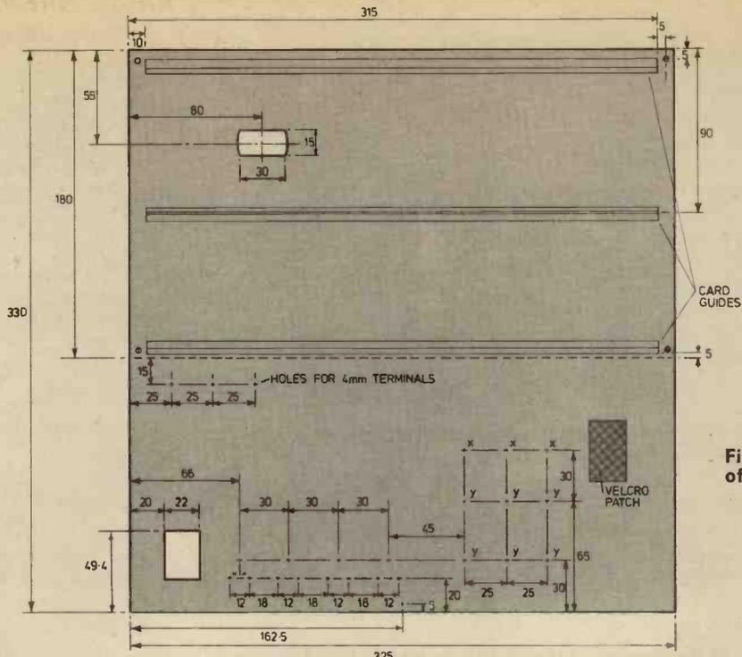
Fig. 4.5. Top/front panel of CHAMP unit
