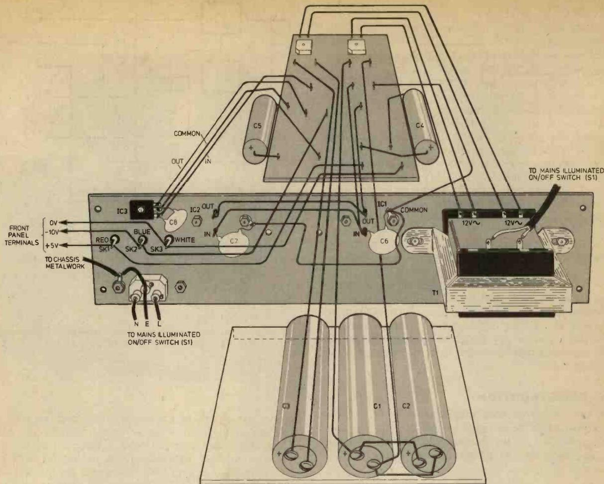
Fig. 4.3. Exploded view and wiring layout of CHAMP power supply. The p.c.b. and the large electrolytic support plate are both mounted on the CHAMP back-plate
