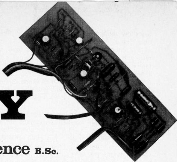
**T**HIS article describes a high performance power supply with voltage control down to zero (yes, zero, not two and a half volts or five and a quarter or, as in the case of many supplies, whatever the Zener voltage used in the system happens to be) and current limit from a few milliamps to several amps.
