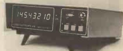
A pre-scaler and amplifier provide facilities for extending the 8 digit counter block to 600Mhz. This is switched in from the front panel. Also provided is switching for gate time and power. A "gate open" l.e.d. indicates when the count is active. A special Xtal in a proportionally controlled Xtal oven is also available.
