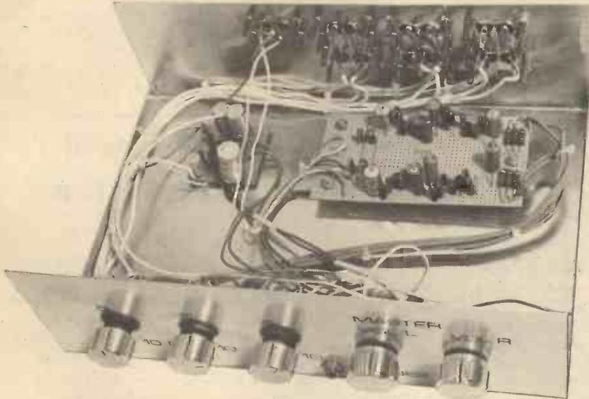
(Left). Chassis interior showing board placement (Below). Wiring to control panel components. All lettered flying leads refer to the main board and the headphone amplifier board
