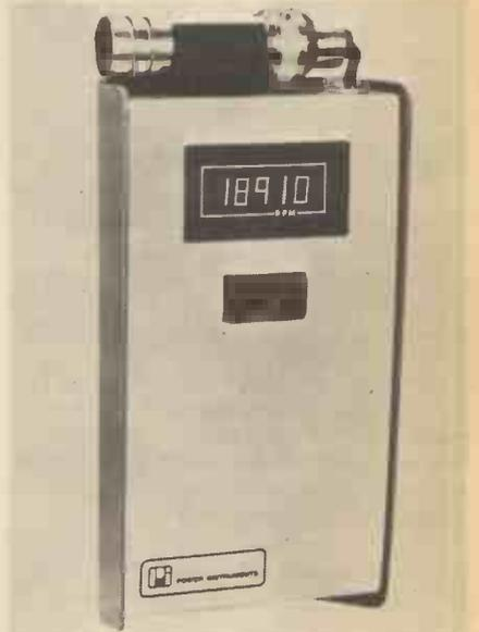
Being touchless, the tachometer can be used in places awkward to reach, and there is a 24in cord attached to the probe. The readout is quartz crystal controlled, with an accuracy of  $\pm 1$  digit up to 0.03 per cent. There is direct reading up to 30,000 r.p.m.
