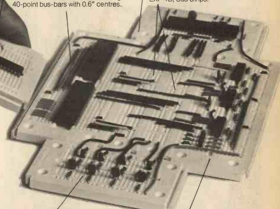
**No soldering** simply plug all standard components in and out, nickel-silver contacts allow Breadboard and components to be used over and over again without damage.
