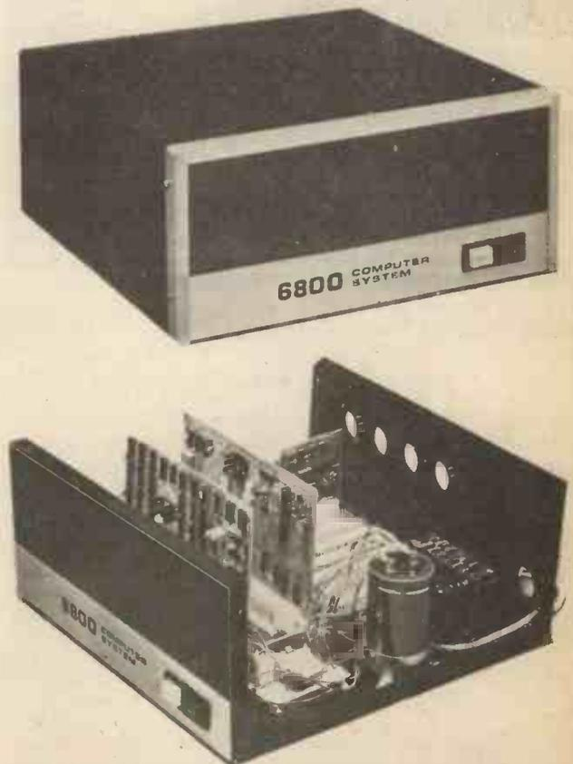
The MP-68 computer system is based upon the Motorola 6800 microprocessor
