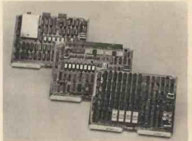
**The SGS-ATES Euro card system is based upon the Z80 microprocessor**
