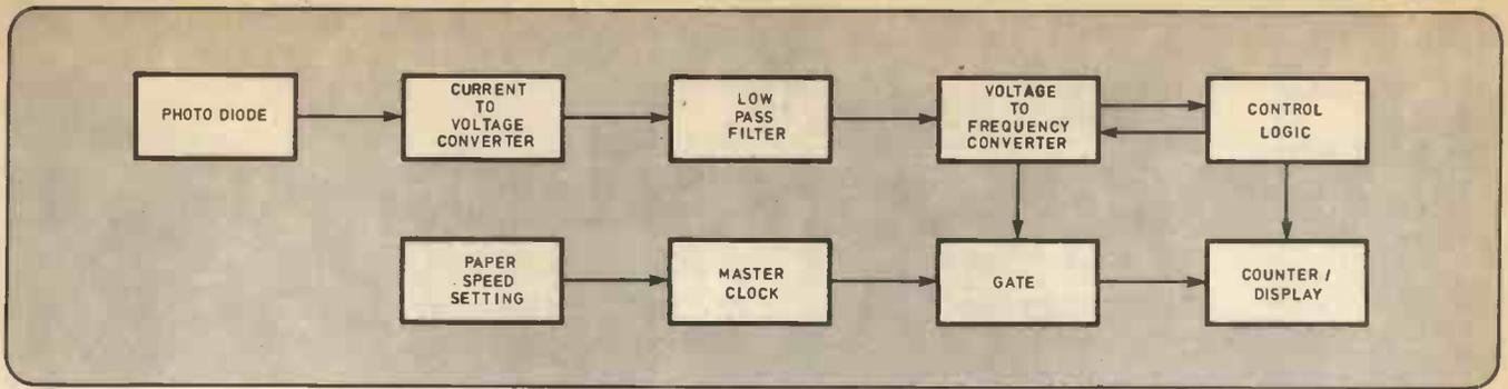
Fig. 1(a). Block diagram of Exposure Meter
