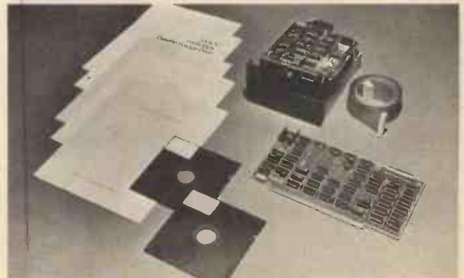
A complete floppy disc system for an S100 computer
