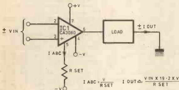
EG 57 Fig. 8. An operational transconductance amplifier
