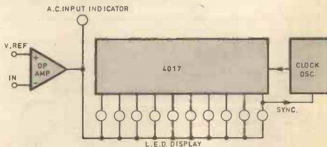
Fig. 2. Block diagram of the Logiscope
