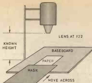
Fig. 5. Making a test strip
