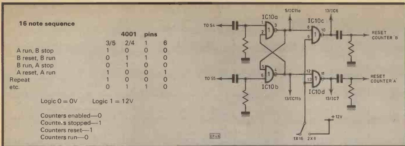
Fig. 4. Showing logic for 16 note sequence. For 2 x 8 sequence the latch is bypassed (IC10a/b). Each counter resets via IC4c/d
