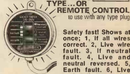
**Safety fast! Shows at once; 1, If all wires correct. 2, Live wire fault. 3, If neutral fault. 4, Live and neutral reversed. 5, Earth fault. 6, Live and earth reversed.**
