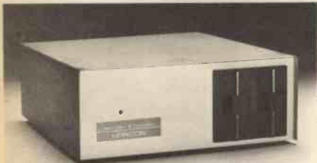
The Horizon microcomputer has dual mini floppy drives and is available with a Disc Operating system
