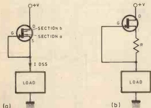
EG 58 Fig. 9. Constant current "diode" principle
