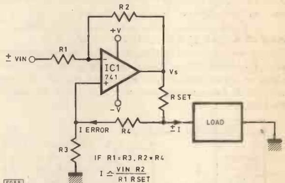
Fig. 6. A bipolar transconductance amplifier
