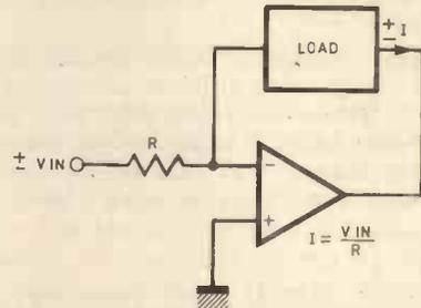
Fig. 5. Simple feedback current generator
