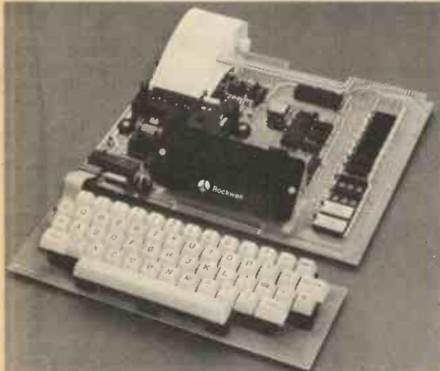
**The AIM65 from Rockwell uses a 6500 microprocessor and includes both a 20 column printer and keyboard**
