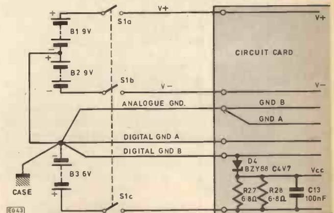
Fig. 1(b). Power supply arrangement
