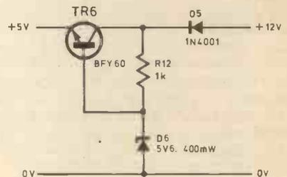
**T**HIS circuit was devised as a simple car alarm which did not require an external de-sense switch. The circuit consists of two parts, the sensor and timer and the relay drivers.
