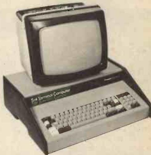
**The SOL terminal computer from Processor Technology is an S100 compatible system using the 8080 microprocessor** time, rather it is used to process the high level language statements in the source program to produce a new machine code version of the program which can then be run by itself. A typical compiled high level language is FORTRAN (FORmula TRANslator) which is widely used for scientific applications. Programming in FORTRAN goes like this:
