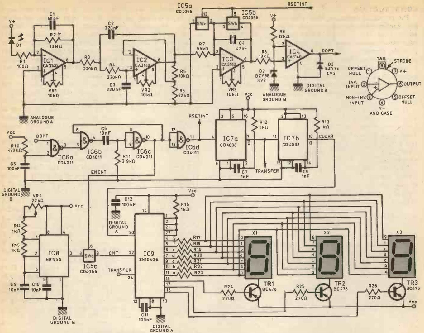
Fig. 2. Circuit diagram. IC1-3 powered by + and -9V, IC4 by +9V and DIGITAL GND B
