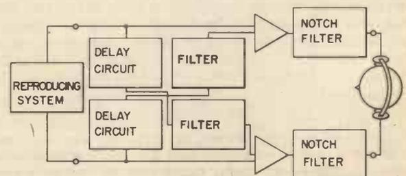
right channels when reproduction is through headphones rather than loudspeakers. To compensate for this Matsushita introduce electronic crosstalk (at low frequencies) between left and right channels. Additionally a slight delay is provided to simulate the slight delay which is introduced by the spacing of a pair of loudspeakers in front of a listener in a room.
