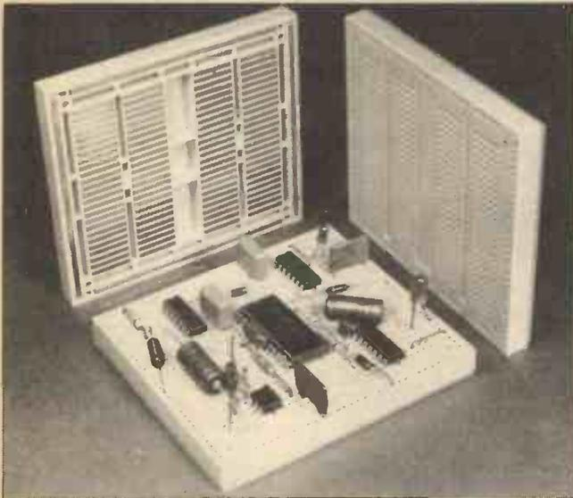
Logically laid out to accept both 0.3" and 0.6" pitch DIL packages as well as Capacitors, Resistors, LED's, Transistors and components with leads up to .85mm dia.
