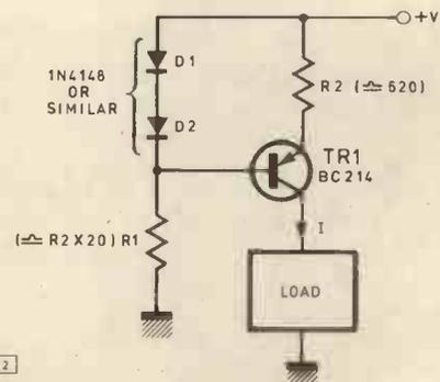
Fig. 3. Transistor current source
