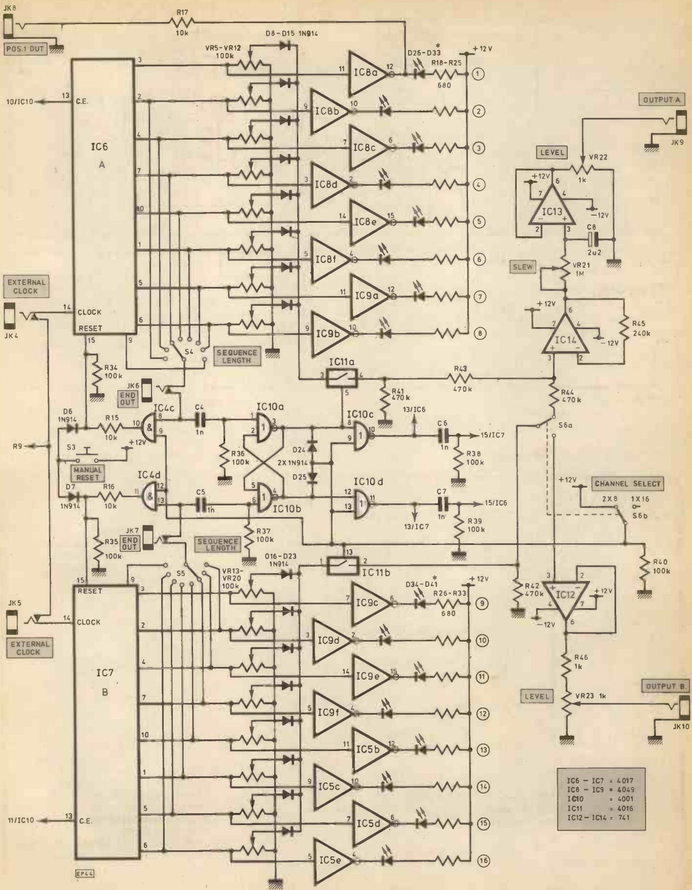
Fig. 3. Counters, channel switching and output stages
