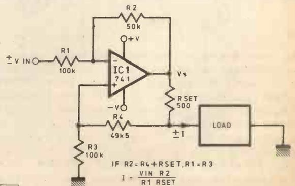
Fig. 7. An improved transconductance amplifier
