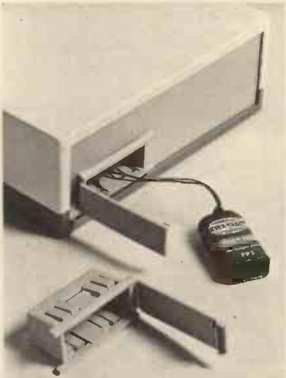
Injection moulding has enabled the design to incorporate moulded retaining clips (holder to case and battery in holder) and also a flip-over hinged cover which snaps shut.
