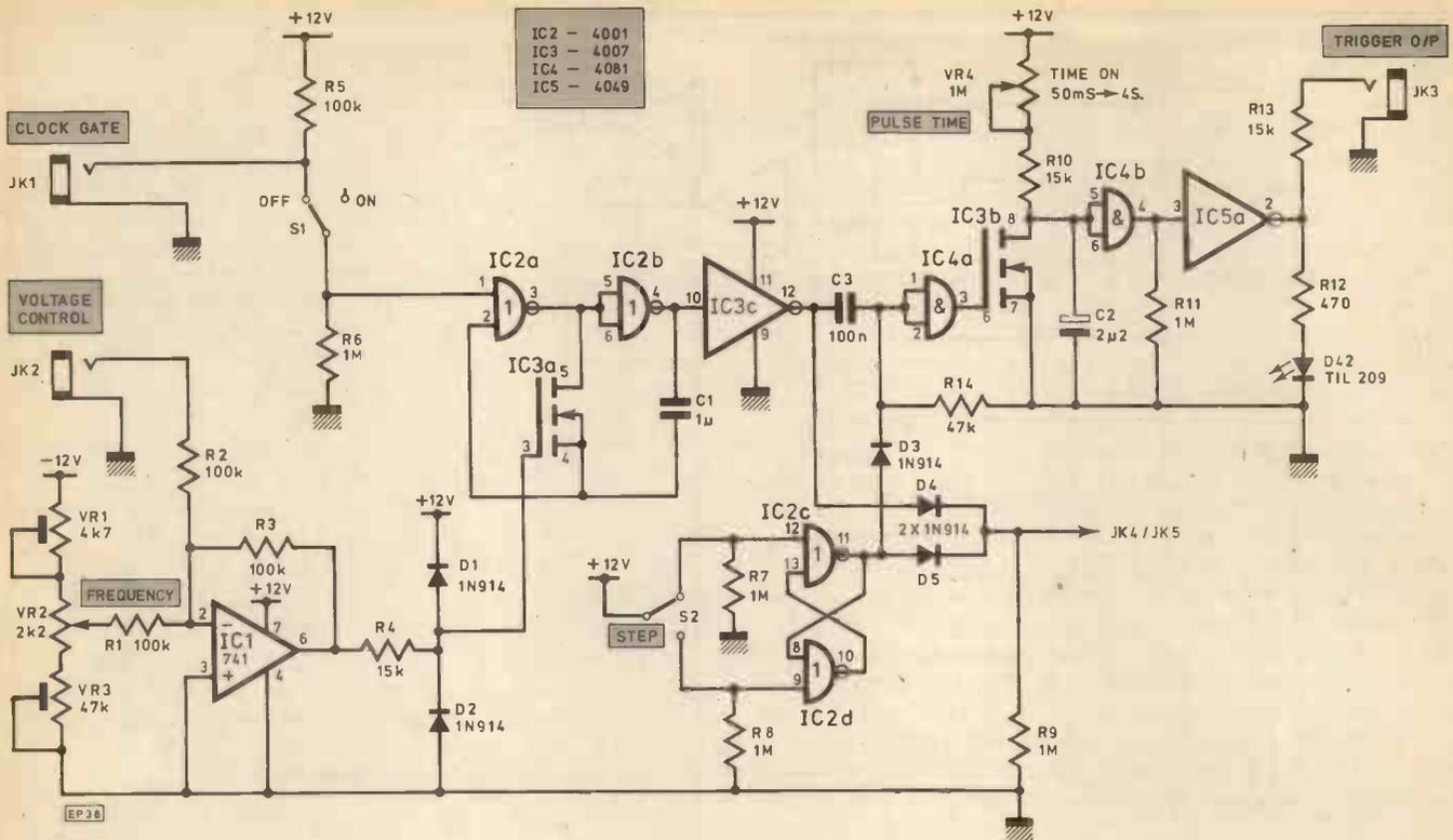
Fig. 2. Sequencer front end
