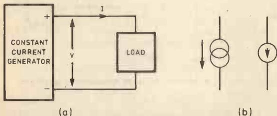
Fig. 1a. Block diagram of a current source
