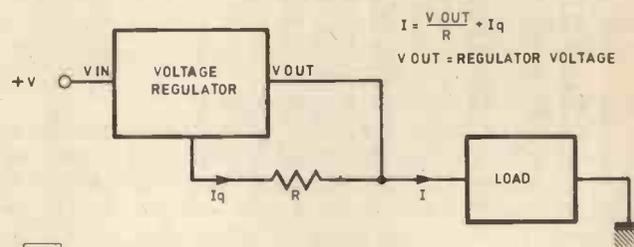
EG 59 Fig. 10. A voltage regulator as a current source
