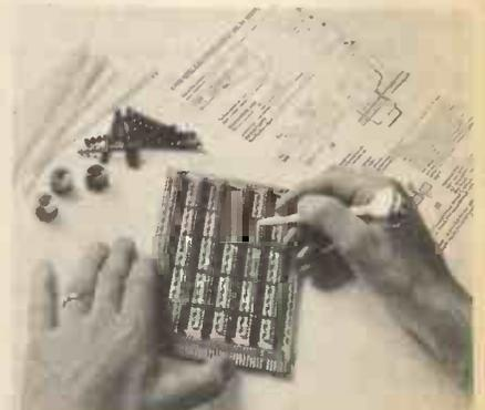
The wiring instrument, or "pencil", feeds the quick soldering enamelled wire from interchangeable bobbins. The instrument is balanced for easy handling and has a fine, long-life steel tip which aids accurate working, even in the most confined areas. Special features are the simple threading system which allows fast bobbin change and the facility provided for adjusting wire tension.
