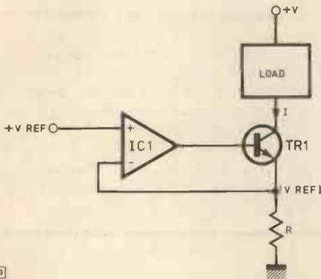
Fig. 4. Precision current sink using an op amp
