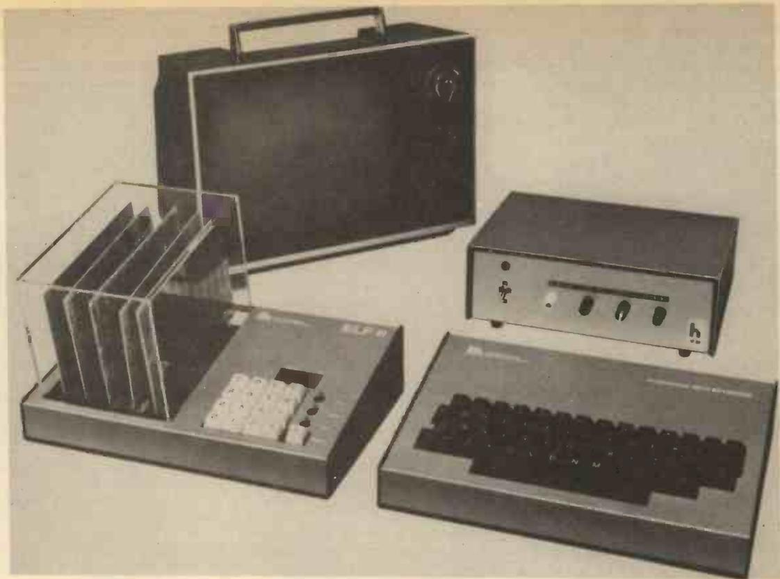
(Above) Elf II with 16K RAM on board, professional ASCII keyboard and power supply
