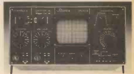
In the XY mode Channel "A" is switched into the horizontal deflection system giving fully matched sensitivities for both X and Y axes over the entire 10mV to 50V/cm range. When used in the conventional mode, the vertical amplifiers are complemented by a 16 range timebase of 1µs to 100ms/cm.
