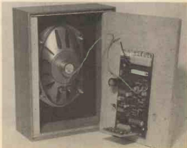
For TR4 to conduct, the voltage at its base must be low (ie 0V). This is achieved initially by the action of the push switch which when pressed connects the base of TR4 via R13 to the 0V rail. This action enables TR3 to supply a regulated voltage of 5V to the circuit which is maintained by the operation of IC1, IC2 and TR2.
