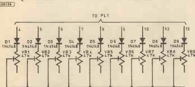
Fig. 2. Circuit diagram of the melody module.
