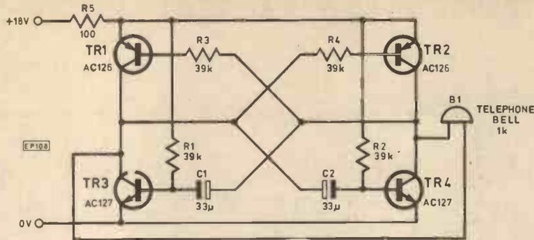
THE circuit shown is suitable for operating a polarised telephone bell from an 18V d.c. power supply (*on no account should P.O. systems be interfered with*).
