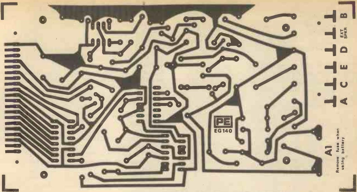
Fig. 3. P.c.b. layout for the Chimesonic
