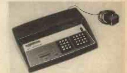
The unit, which is based on the Signetics 2650 microprocessor, is equipped with an S-100 expansion interface which allows it to be used as a small computer limited only by the peripheral boards used. In addition, the program/data-entry and debug facilities of the basic Instructor 50 can be extended to any device connected to the interface.
