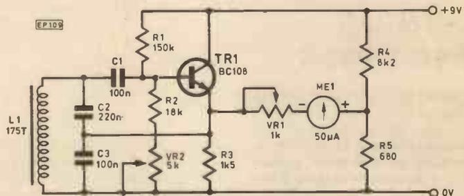
L1, it follows that the voltage across R3 will now fall towards its quiescent value. This change of voltage is indicated by a 50µA meter, zero adjustment being performed by VR2.
