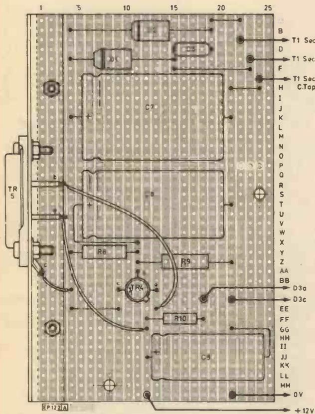
Fig. 4 Layout of p.s.u. board
