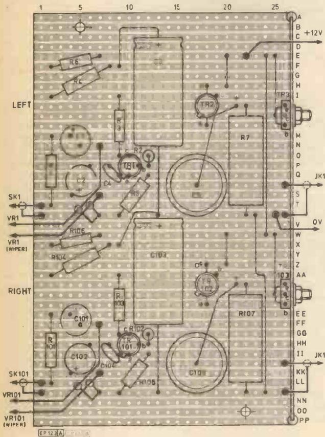
Fig. 3 Layout of stereo amplifier board
