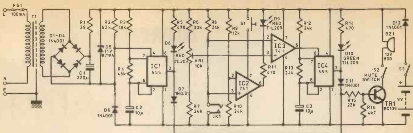
Fig 1. Circuit diagram of the Freezer Alarm.
