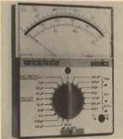
For values above  $3\mu$  a system of timing the interval between flashes of an l.e.d. provides direct indication of capacitance value. On two selected ranges, capacitance can be indicated as  $1\mu$  per second or  $100\mu$  per second, thus extending the range to several thousand  $\mu$ F.
