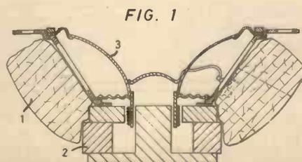
The earlier idea from Rank goes a stage further. As shown (in Fig. 2) there is again a doughnut shaped ring 1 which sits on the loudspeaker magnet 2 and backs onto the rear of the loudspeaker diaphragm. But additionally Rank provide a second damping element 3 which takes the form of an open cylinder of foam surrounding the loudspeaker unit. Together the damping elements 1 and 3 absorb and deflect the rearward directed sound from the diaphragm.
