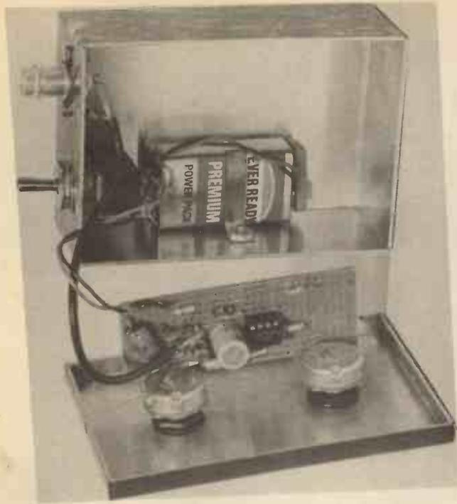
Although the prototype oscillated up to 7.5MHz, it was only calibrated up to 3MHz, because of the cramping of frequency above this. With a little thought, a fine tuning control could be connected around VR1 to make these frequencies available.
