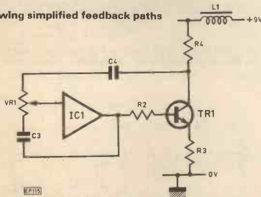
If the Veroboard layout is changed, and the pots mounted off the board, there may be trouble with stray capacitance. The board, BNC output socket and switch should be mounted in an all metal box for screening. For the prototype a 40 x 100 x 70mm aluminium box was used, with the pots mounted on the lid. These were considered sufficient support for the board.
