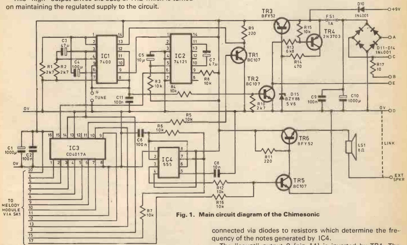
Fig. 1. Main circuit diagram of the Chimesonic
