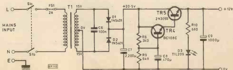
Fig. 2 Power supply circuit for both channels
