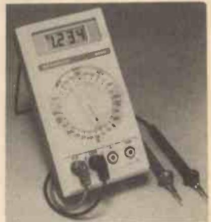
The meter has an input impedance of 22MΩ. Accuracy is to within 0.1 per cent + 1 digit on all d.c. voltage ranges. Both a.c. voltage and current are average r.m.s. measurements.
