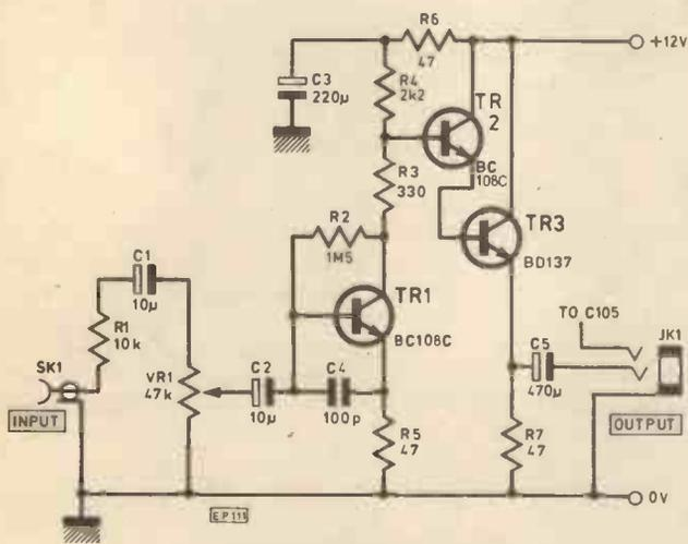
Fig. 1 Single channel of amplifier
