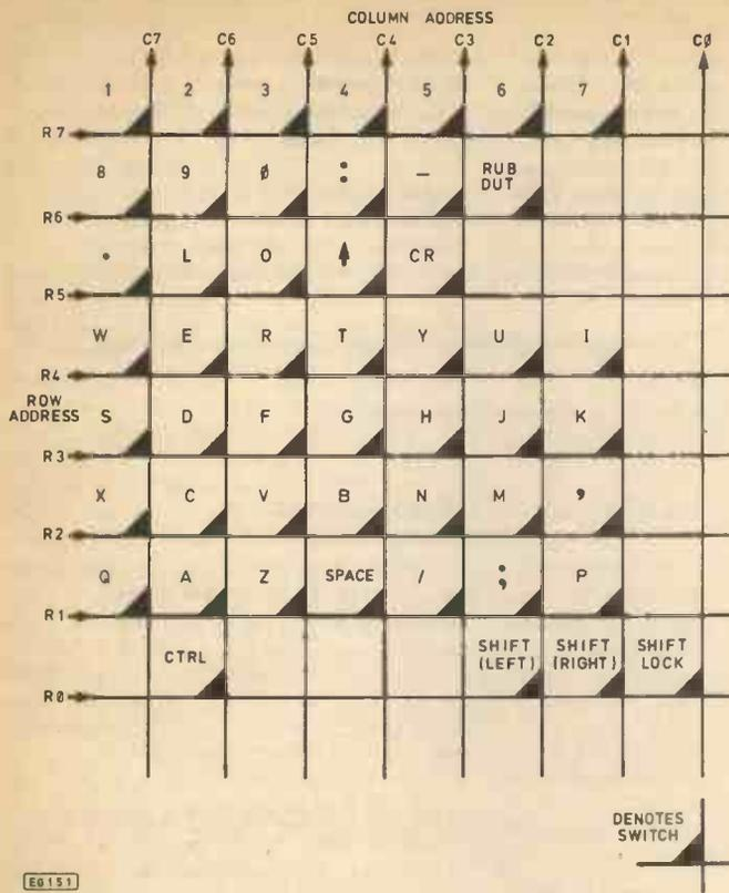
Fig. 3. Above: Keyboard switching matrix
