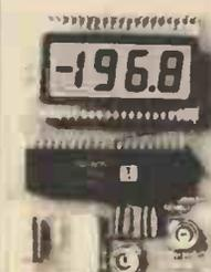
Based on the 7106 single IC 3½ digit D.V.M. the Kit contains a PCB, resistors, capacitors, pre-sets, I.C. and 0.5" liquid crystal display. Components are also included to enable the basic D.V.M. kit to be modified to a Digital Thermometer using a single transistor as the sensor. Requires a 2mA 9V supply (PP3 battery).
