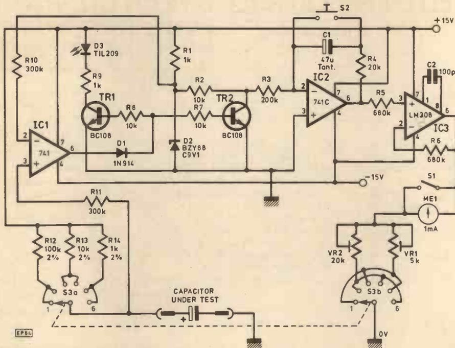
**C**APACITORS of values up to 10,000µF can be measured with this instrument, and 6 ranges are available as follows:
