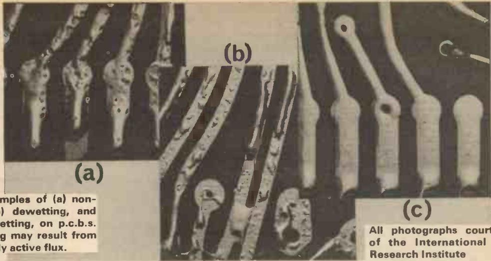
Typical examples of (a) non-wetting, (b) dewetting, and (c) good wetting, on p.c.b.s. Non-wetting may result from insufficiently active flux.
