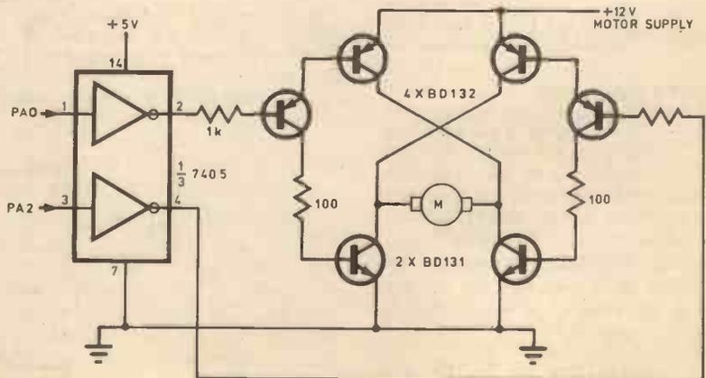
Fig. 3. Circuit which provides control of an electric motor from two logic-level lines
