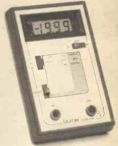
The instrument has 15 different ranges and can resolve voltage to 0.1mV, current to 0.1 $\mu$ A and resistance to 0.1 $\Omega$ . Auto-polarity and auto-zero are standard. Inputs are via 4mm terminals and are protected against overloads and transients.
