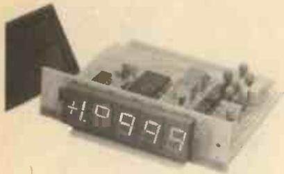
Accuracy is guaranteed to  $\pm 1$  count over the entire range, giving a resolution of up to  $10\mu\text{V}$ . Auto-polarity, auto-zero, b.c.d. outputs, digital hold and programmable decimal points are standard features.
