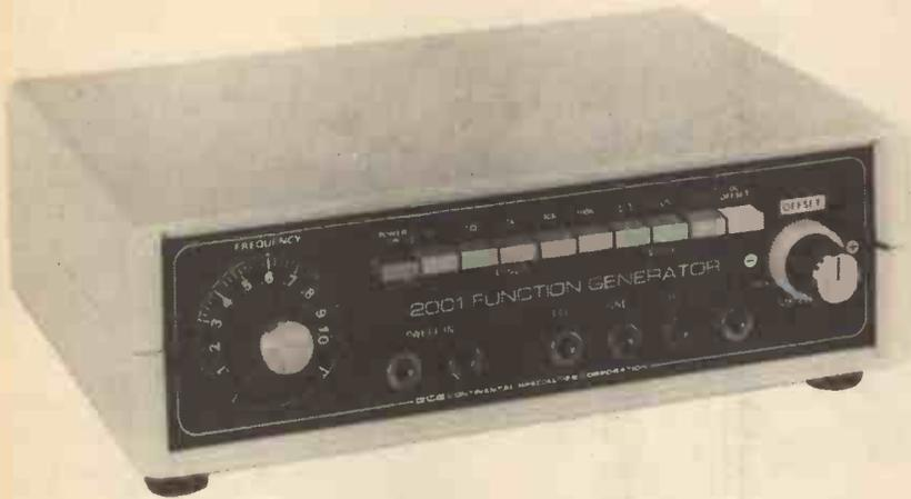
The variable d.c. offset amplitude control, once set, holds the output signal to within  $\pm 0.5$ dB over the entire frequency range.
