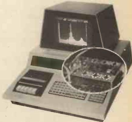
The manufacturers suggest that the plug in board can be used for measuring sound and noise levels, for optimising the equalisation of a hi-fi or public address system, for checking the frequency response of audio components, and for speech and sound pattern recognition.
