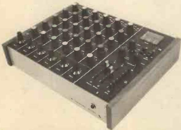
(Above) Prototype control panel layout. In the modified design the limiter switch is excluded. (Below) Headphone outlet is on the front panel with inputs to the rear
