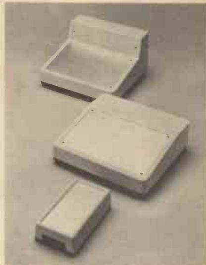
The other case, 150 x 85 x 45 mm high, has a front panel for identification and controls, which is protected by a raised edge all round. Assembly of components and connections to the front panel is simple as, with the case cover removed, components are accessible from all sides. The front panel is connected to the base by moulded posts and retained by the case cover. P.c.b. mounting pillars are moulded into the base, and a raised end surface is provided for cable grommets or components.
