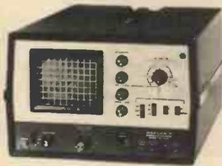
IO 4105—Single Beam 5 MHz Oscilloscope
