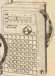
This neat three band Superhet receiver not only provides an invaluable service, checking your channel and TX, but gives normal broadcast reception when you need it as well.
