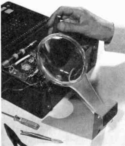
The lens, the wide rim protecting it and the flat handle are made as a single integral moulding from a high-grade acrylic material, which is shatter-resistant and has a better light transmittance than any glass lens. It has a diameter of 96mm (approx 4 inches), permitting both eyes to be used to view the work. Magnification is about 2 times.
