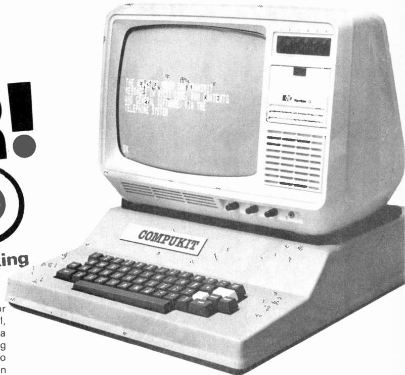
This beautiful orange and black finish plastic case is available for Superboard II, CompuKit UK101 or, with an uncut keyboard panel, for mounting many other hobby computers. It is supplied with a mounting wedge to give a suitable keyboard angle and fixing screws for Superboard or CompuKit. The case is strong enough to support a small portable TV or video monitor and has ventilation slots and a cable access panel at the back. It **does not** carry the "PE CompuKit" badge shown in the photograph.
