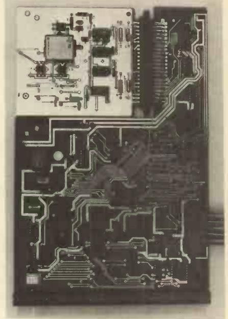
The real time clock has a deac battery back up, the capacity is sufficient to power the CMOS clock chip for approximately 12 months in the absence of system power.
