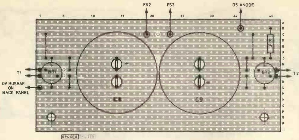
Fig. 11. Veroboard layout of the p.s.u
