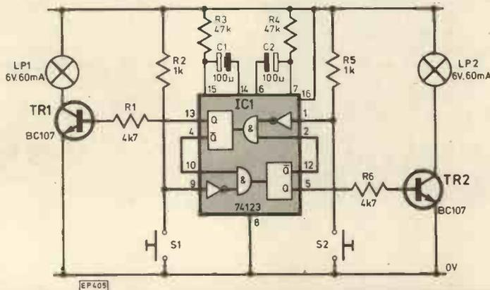
**I**F S1 is shorted, the one shot will be triggered and LP2 will light for about 3 seconds assuming that the other stage is not already in a triggered state. While lamp one is alight any closure of S2 will not cause LP1 to light as the one shot is inhibited by a logical 0 at pin 2. The same applies if the order is reversed.
