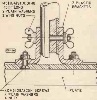
**Fig. 6 (left). Search plate mounting assembly**
