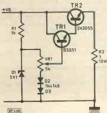
**W**HEN carrying out battery capacity checks, it is extremely useful to have a load that does not need constant adjustment to maintain a steady current as the voltage falls.
