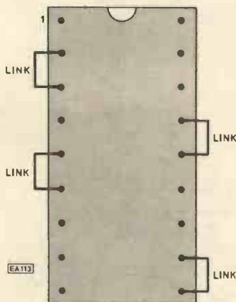
Fig. 8. Blanking plugs for IC6 and IC7 sockets on the 101
