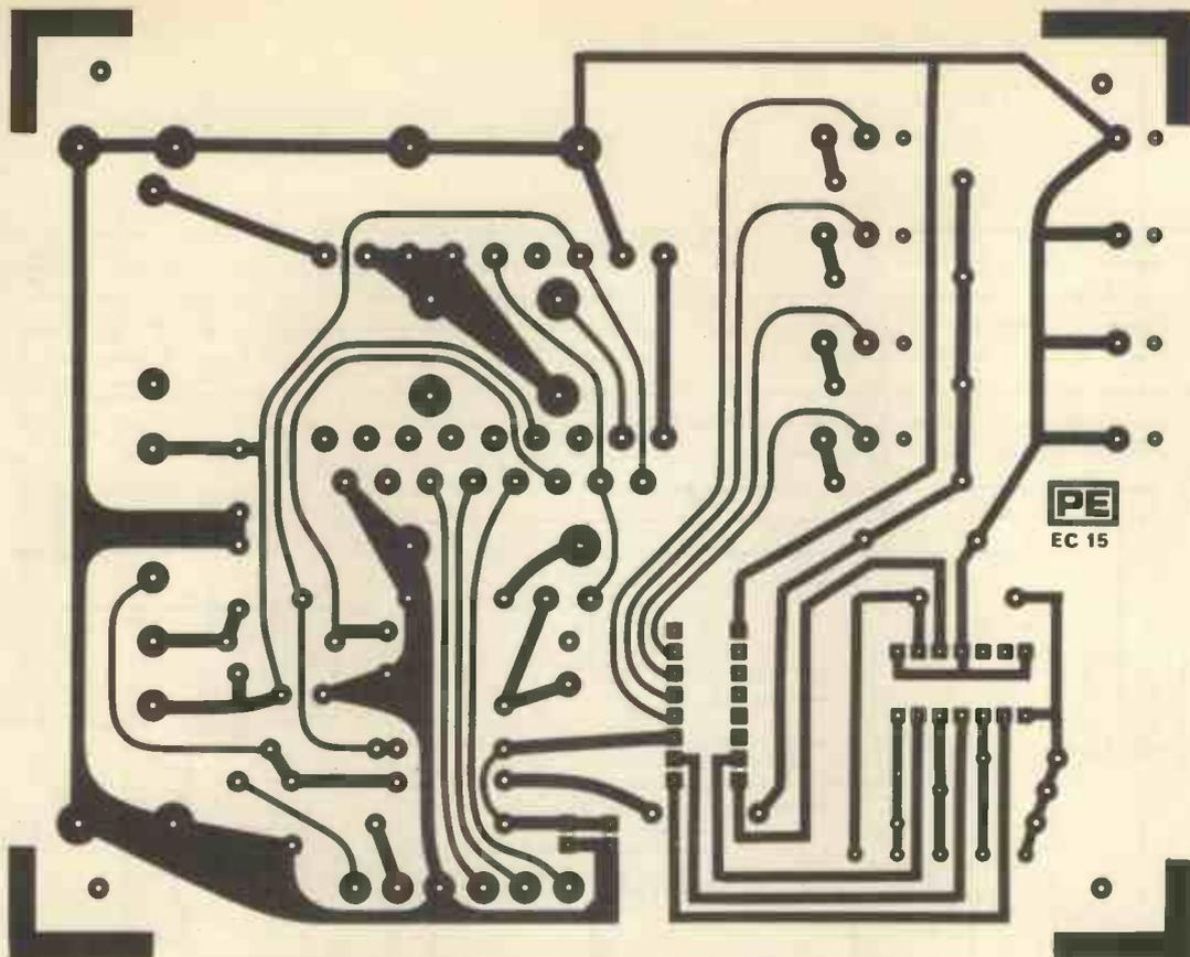
Fig. 2.3. P.c.b. design of the Tuner
