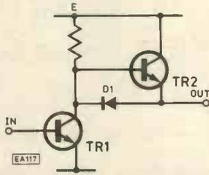
Fig. 4. Basic Class A stage with an emitter follower
