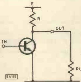
Fig. 2. Simple Class A circuit
