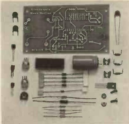
The sound effects board has been designed around the SN76477 sound generator and includes a noise generator, VCO, noise filter, mixer, attack/decay circuit, audio amplifier and control circuitry. A prototype area is provided on the p.c.b. for experiments and among the many sounds available are one-shot controls for gun shots, explosions etc., bird sounds, sirens, race car crashes, steam trains, etc.,
