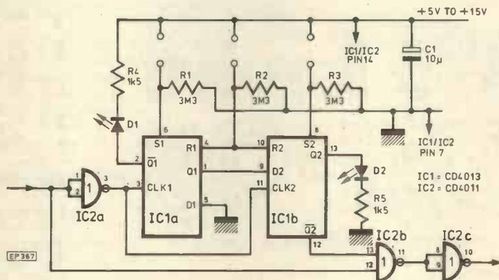
thing for the next pulse but one. Since the input is an alarm signal, the circuit will selectively inhibit this signal for the following two days.
