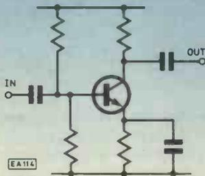
Fig. 1. Conventional R.C. coupled stage
