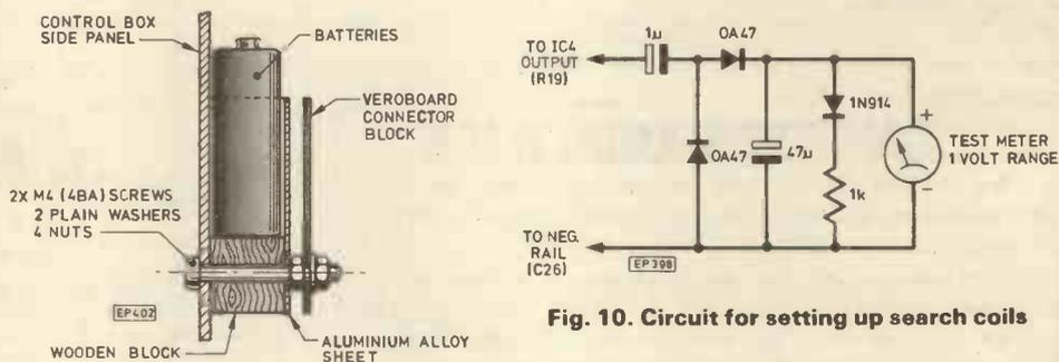
Fig. 10. Circuit for setting up search coils
