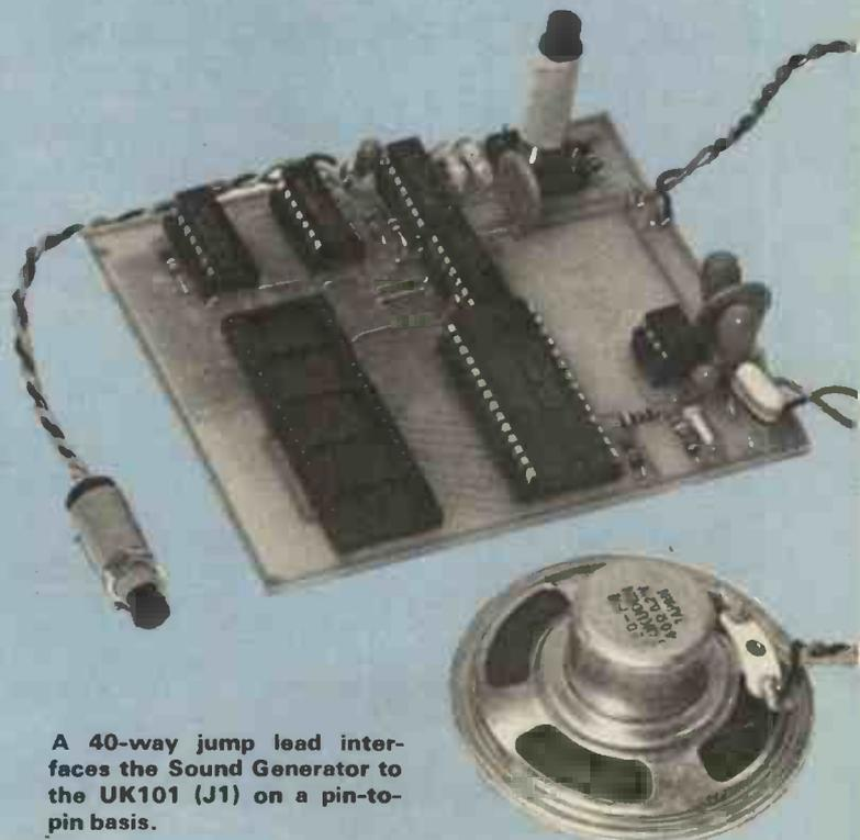
A 40-way jump lead interfaces the Sound Generator to the UK101 (J1) on a pin-to-pin basis.
