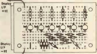
You will need; One EXP 300 or EXP 350 breadboard, 15 silicon diodes, 6 resistors, 6 Light Emitting Diodes.
