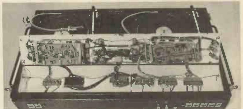
decoupled at high frequencies for stability (C41 etc) and additional capacitors (C37-40) are provided to attenuate common mode RF1 and to decouple the supply rails at audio frequencies.
