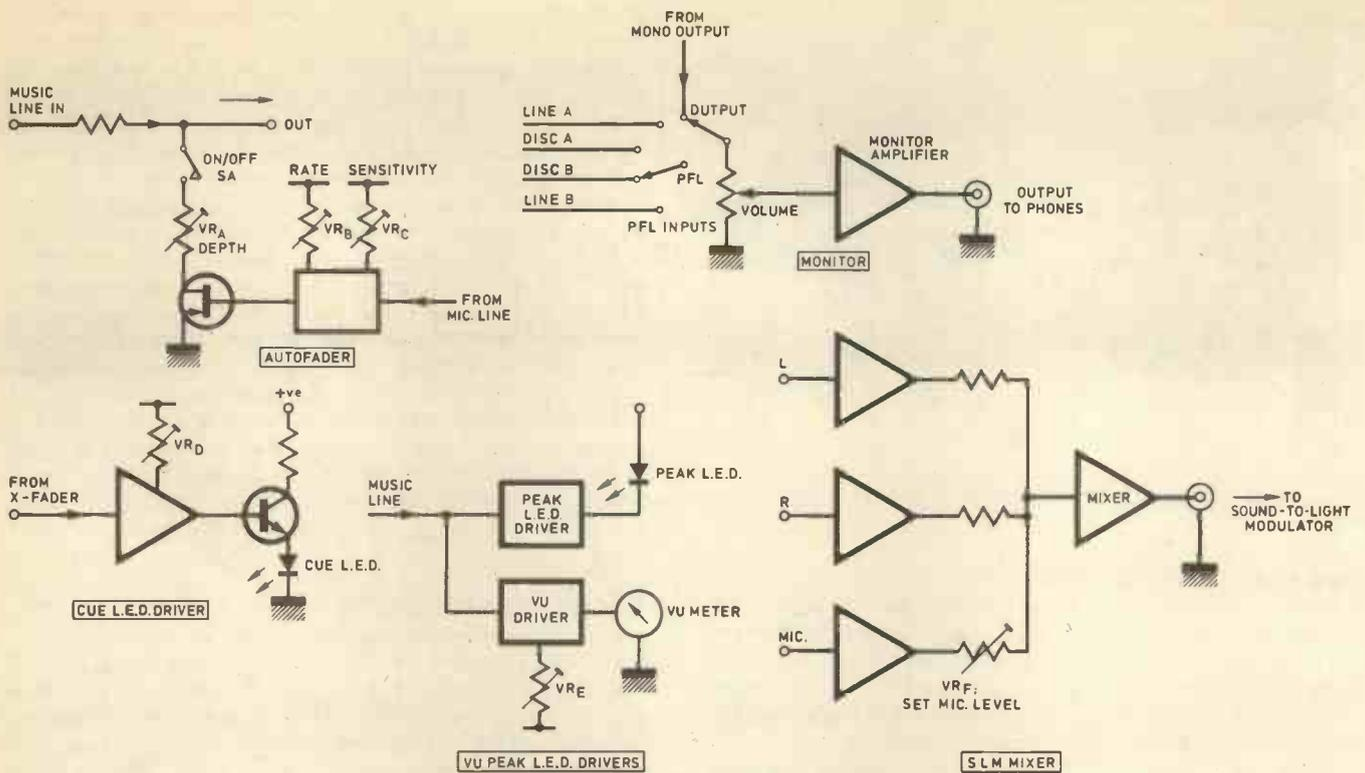
Fig. 2. Block diagram of auxiliary functions
