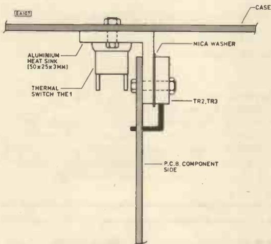
Fig. 10. Mounting details for the heatsink
