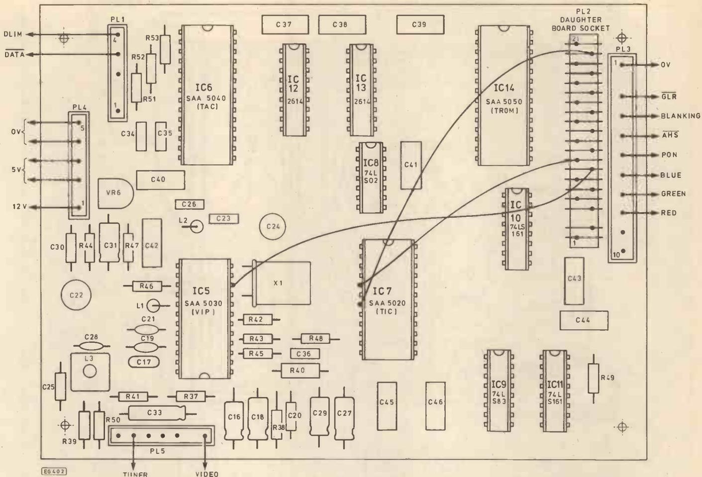
Fig. 2.6. Component layout of the Decoder Board. Note C32 is not used on the supplied board
