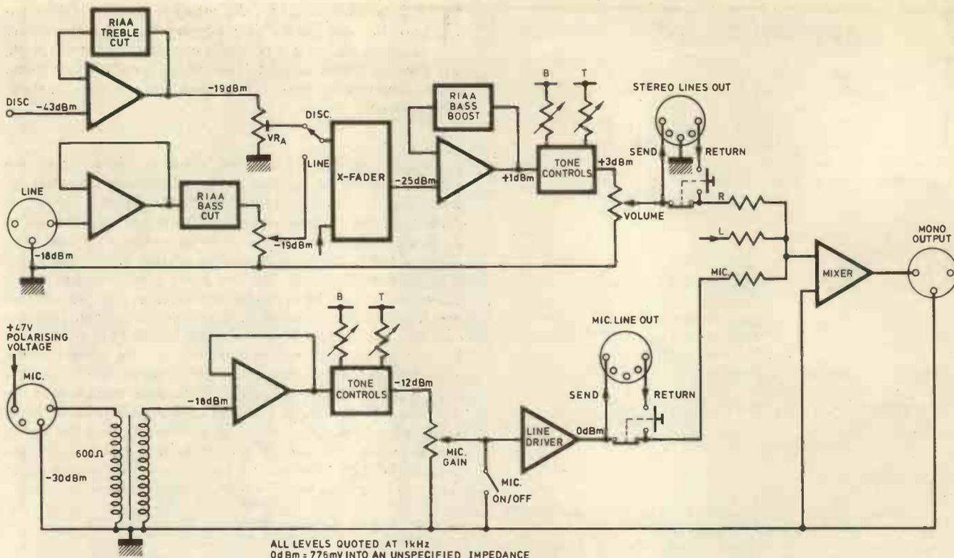
Fig. 1. Block diagram of main circuitry
