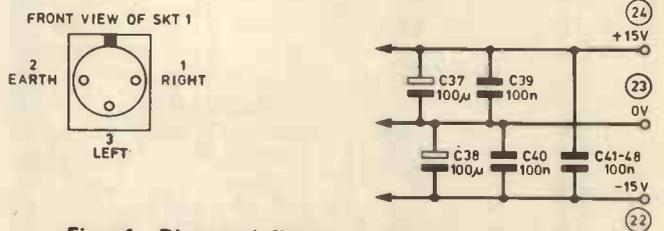
**Fig. 4. Disc and line input stages (Card 1), socket detail and line decoupling**
