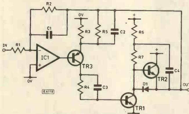
Fig. 5. Improved Class A circuit
