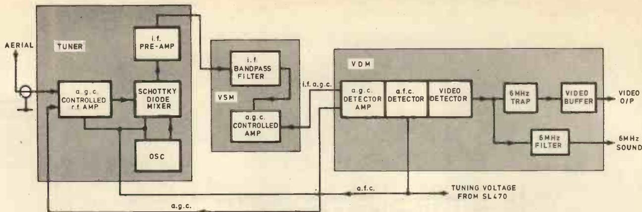
Fig. 2.1. Block diagram of the Tuner
