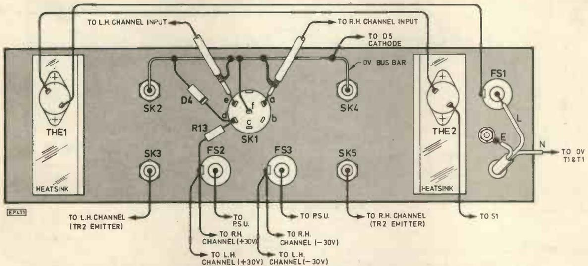
Fig. 12. Wiring diagram for the rear panel.
