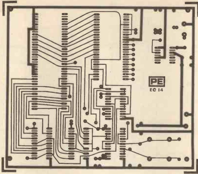
Fig. 6. Printed Circuit layout (actual size)
