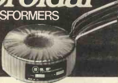
We use advanced winding technology to make our toroidal transformers. They have only half the weight and height of their laminated equivalents and are appreciably more efficient. Our toroidals cost virtually the same as their now outdated laminated equivalents and hum is down to a negligible tenth of what it used to be. Supplied with rigid mounting kit with centre bolt, two neoprene and one steel washer. Available so far in a range of 37 sizes with more to come.
