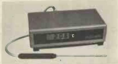
Its dual range facility enables temperature in the range of 120°C to 700°C to be resolved at the flick of a switch without the need to change the indicator or probe. This eliminates the tolerance errors in indicator and probe that are applicable to a single-range instrument.
