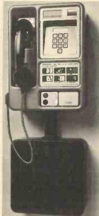
The PP2000 is a microprocessor controlled payphone developed by Plessey engineers at Liverpool
