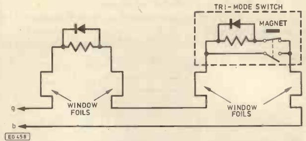
Fig. 2.10. Tamper-proof system for window foils.
