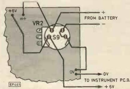
**Fig. 6. Wiring connections to S9**
