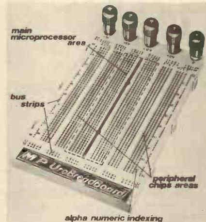
Capable of accepting .3", .4", .5" and .6" pitch d.i.l. packages without needlessly wasting auxiliary pin positions and breadboarding areas, every contact is alpha-numeric indexed, this being imperative for education and training applications where step-by-step build-up instructions are used.
