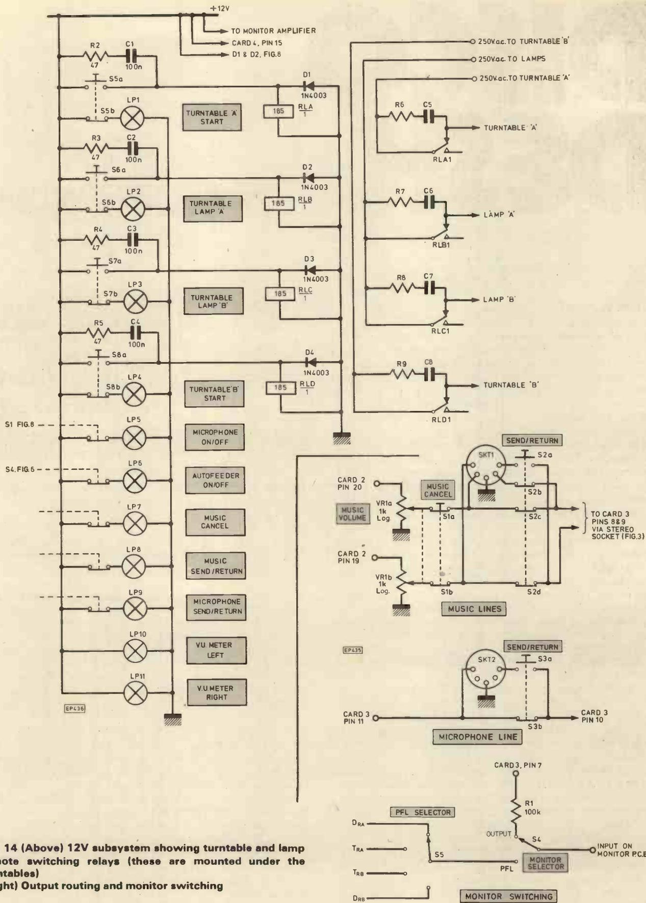
**Fig. 14 (Above) 12V subsystem showing turntable and lamp remote switching relays (these are mounted under the turntables) (Right) Output routing and monitor switching**
