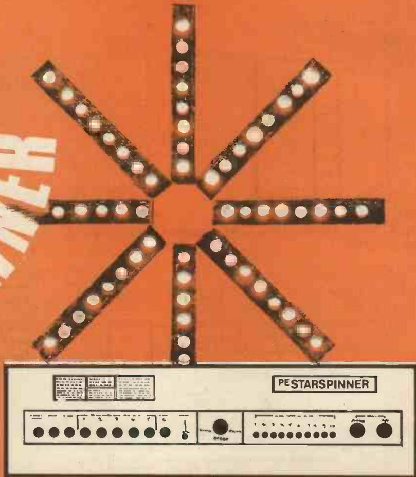
Most people have seen the fascinating rotating and radiating displays available from modern "zoning" or "matrixing" lighting systems. The *PE StarSpinner* can produce 62 dynamic effects of this type plus two static effects and a sound to light advance facility—full circuit and construction details start next month.
