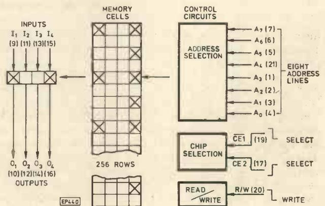
Fig. 1. Showing simplified operation of a 5101
