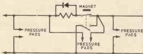
Fig. 2.9. Shunt sensors can be connected across the loop or across a 'tri-mode' sensor
