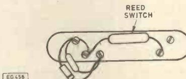
Fig. 2.6. After soldering, the resistor and diode should be fitted inside the switch. Note the reed switch is fitted inside the body of the switch and cannot be seen.
