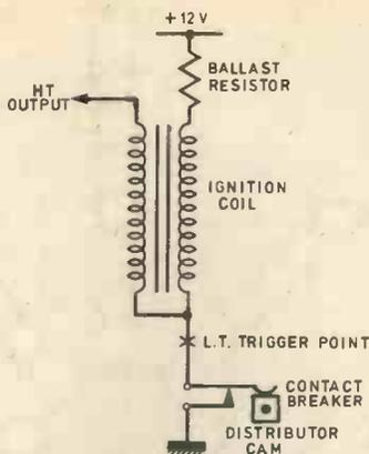
Fig. 4. Ignition system triggering
