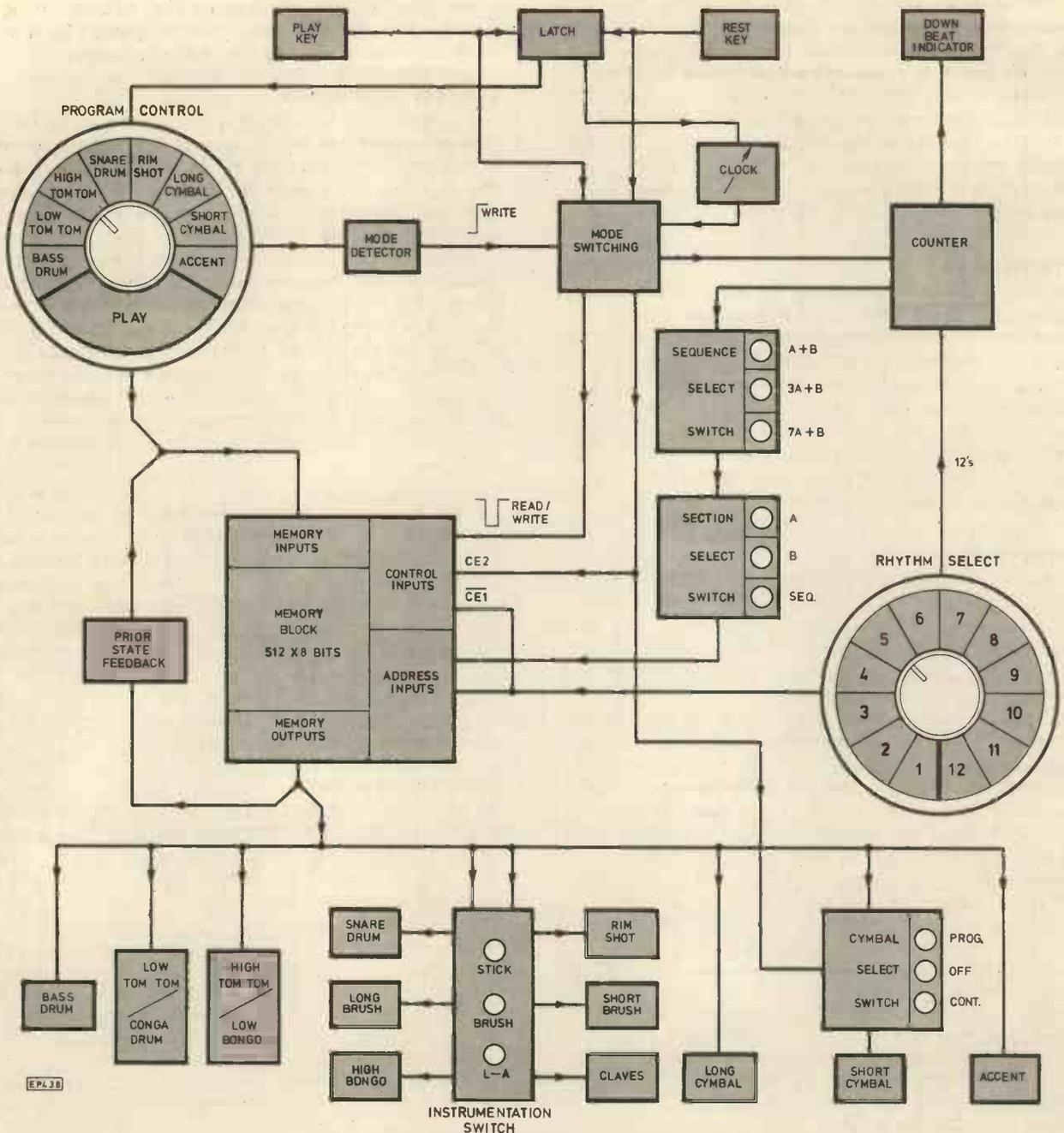
Fig. 2. Schematic of Master Rhythm
