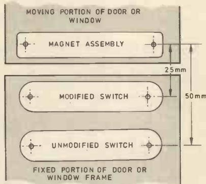
Fig. 2.8. Switch mounting details
