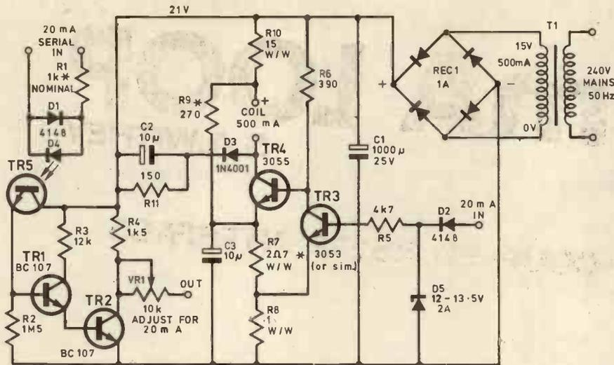
Fig. 1. Circuit diagram of opto-coupled 20mA loop. When in opto-isolated mode, the OUT from VR1 is connected to IN at D2 (as on p.c.b.) The input at D2 can be used as a non-isolated RS232 input
