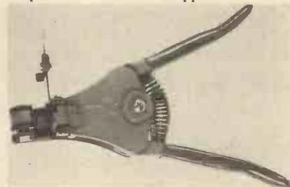
A single squeeze operation strips the insulation from single and stranded wires without damage. Its wide jaws permit fast and accurate stripping without any nicking or scraping of the wire and a gauge is supplied to ensure consistent lengths of stripping during fast production work. Five diameters of wire can be used on this tool, which has the following size cutter: 1.0, 1.6, 2.0, 2.6 and 3.2mm. Of an all metal construction, it is available ex stock priced £10.50.
