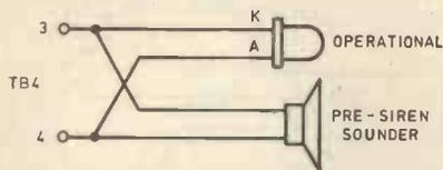
Fig. 2.5. Pre-signal unit wiring
