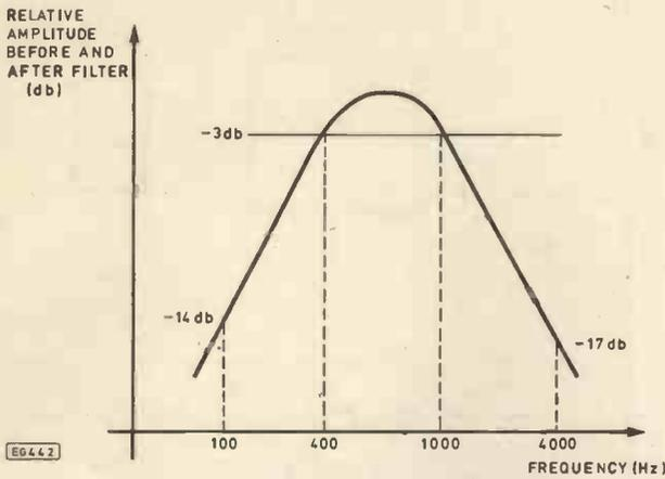
Fig. 2.3. Bandpass filter characteristics
