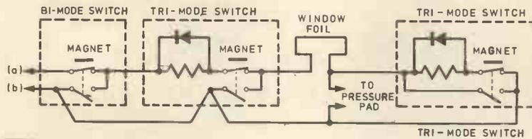
Fig. 2.7. Basic loop system. If a shunt device is used at the end of a loop then an extra wire is required. To overcome this problem each loop should end with a tri-mode switch
