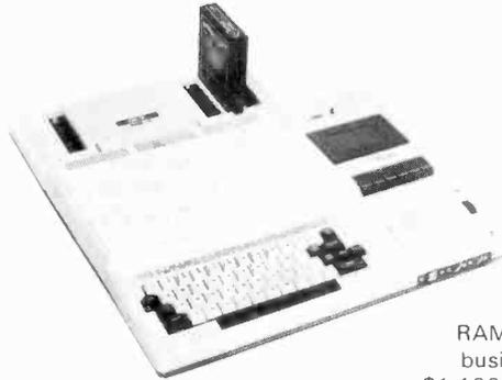
The Imagination Machine II with 27K RAM, 14K ROM, is a small business system with r.r.p. \$1,199. It features up to eight video colours, sound synthesiser, BASIC or 6800 m/c, object orientated and point resolution graphics. Photo shows floppy interface module inserted. *Courtesy of APF Electronics.*
