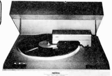
New Revox B795 direct drive turntable with Linatrak tangential tracking system. Motors are controlled by Hall effect sensors via quartz-referenced phase locked loops. Courtesy Studer Revox America Inc.
