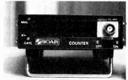
The unit which measures only 100x32x120mm has a frequency range of 10Hz to 50MHz and can measure up to 500MHz with a prescaler. Powered by either 4 penlight batteries or an external d.c. supply (8 to 11V) the instrument has a 4 digit display and a resolution of 10Hz/10kHz with a maximum input of 20V.
