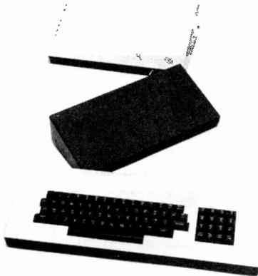
The consoles are of all aluminium construction and incorporate ventilation slots in both rear and bottom panels with a gasket fitted between the panels to reduce vibration.
