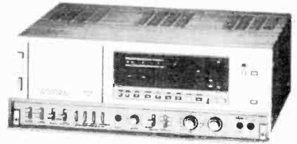
Put a tape of any oxide formulation into this cassette deck, and the on-board computer will have adjusted to correct bias, equalisation and sensitivity within seconds. Functions are solenoid (logic) controlled. The fluorescent bar meter allows for peak hold, and Dolby noise reduction is included in the GX-F95. *Akai America Ltd.*
