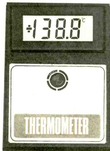
**Precision Digital Thermometer;**  $-55^{\circ}\text{C}$  to  $+150^{\circ}\text{C}$ ; stainless steel probe; laser trimmed i.c. sensor giving excellent linearity and easy calibration.
