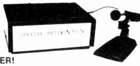
**BIG EARS** opens the door to direct man-machine communication. The system comprises analogue frequency separation filters, preamps and signal conversion, together with a quality microphone and extensive software. Words, in any language, are stored as "voice-prints" by simply repeating them a few times in "learn" mode. Using keyword selection techniques, large vocabularies can be constructed.
