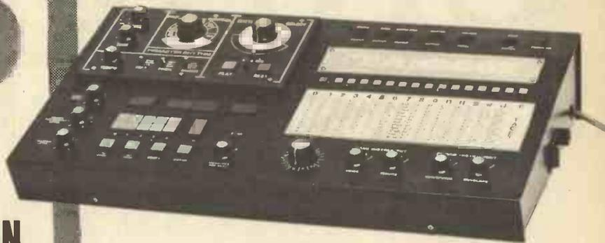
**T**O complete assembly of the Band-Box, the Display board requires to be joined to the System board and various interconnecting leads prepared. A seven pin DIN socket is also required to be fitted to the Master Rhythm to provide the necessary control pulses and drum audio to the Band-Box.
