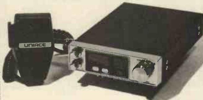
Details of the Uniden Uniace 100 FM mobile CB rig arrived in our offices too late to be included in our rig guide last month. The Uniace 100 features the basic channel, volume and squelch controls, plus PA/CB and 4W/0.4W power switches. Being only 40mm high, it is not as cumbersome as rigs with more features (including its big brother, the Uniace 200), which is worth bearing in mind if you own a small car.
