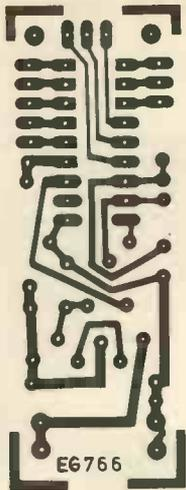
Fig. 1. P.c.b. design for the transmitter
