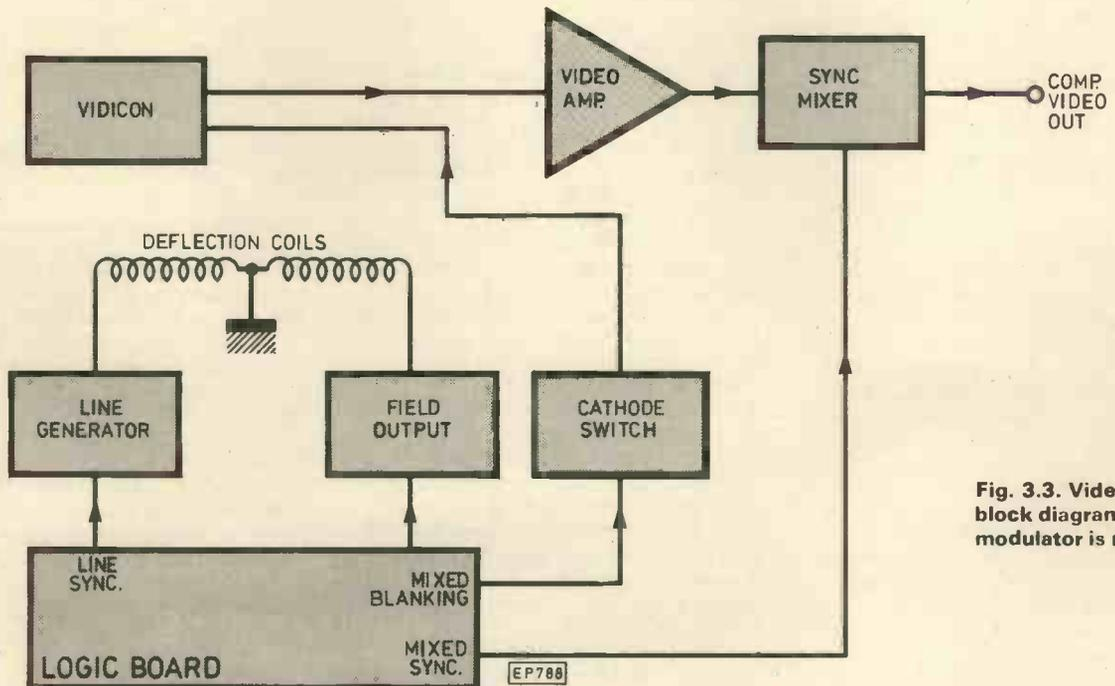
Fig. 3.3. Video and logic block diagram. The UHF modulator is not shown
