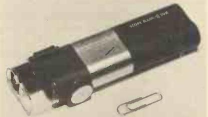
Can't quite make out that dry joint or broken p.c.b. track? What you may need is a pocket microscope, and Stotron Ltd. have recently introduced one which could be just what you need. With 20X magnification and a graticule showing linear and angular measurements, the unit is only 125mm long. Illumination is powered by standard 1.5V penlight batteries, and a micro-stand with spring clips for sample slides is also available, so the microscope can be used like a conventional model.
