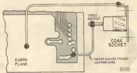
Fig. 3.4. Connection to the VHF modulated video output socket
