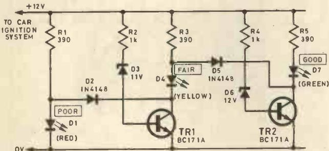
Fig. 1. Circuit of Indicator
