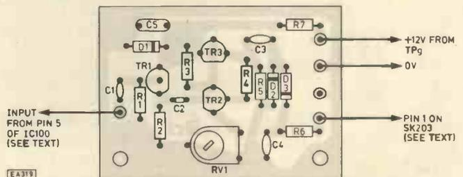
Fig. 3.3. Component layout for the S-meter module
