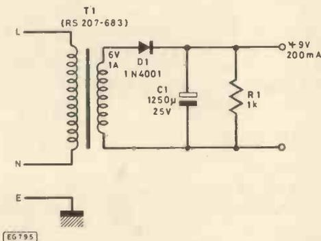
Fig. 2. A mains supply that can be used
