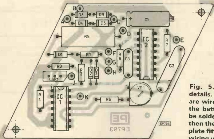
Fig. 3. Component layout for the p.c.b. If T1 has a centre-tapped secondary, leave D8 and D9 off the board. If T1 has a single-winding secondary, use terminals A and C only, and include D8 and D9.
