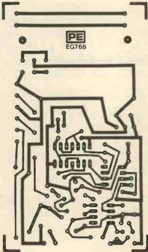
Fig. 5. P.c.b. design for the Receiver board
