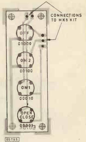
Fig. 4. Switch layout
