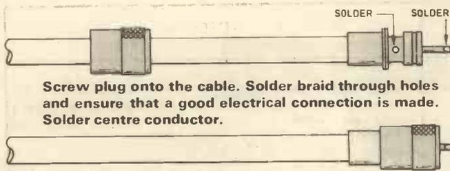
Screw plug onto the cable. Solder braid through holes and ensure that a good electrical connection is made. Solder centre conductor.
