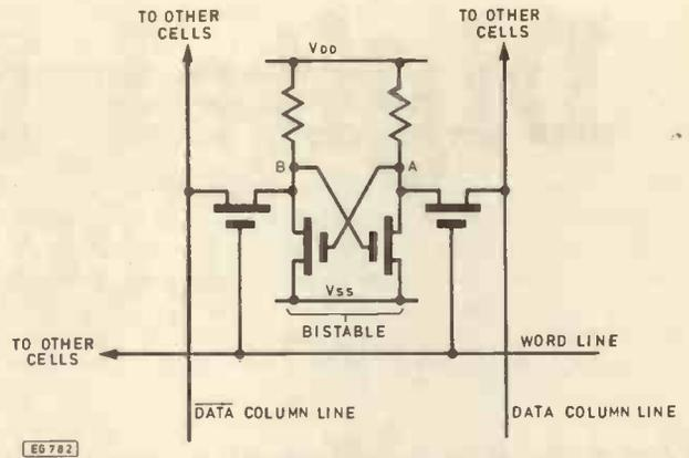
Fig. 8.1. The static memory cell
