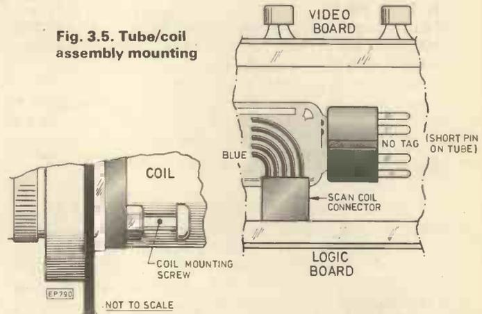
Fig. 3.5. Tube/coil assembly mounting
