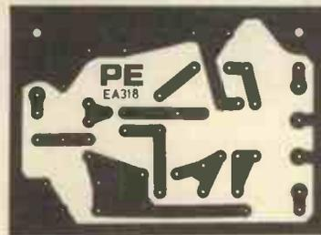
Fig. 3.2. P.c.b. design for the S-meter module
