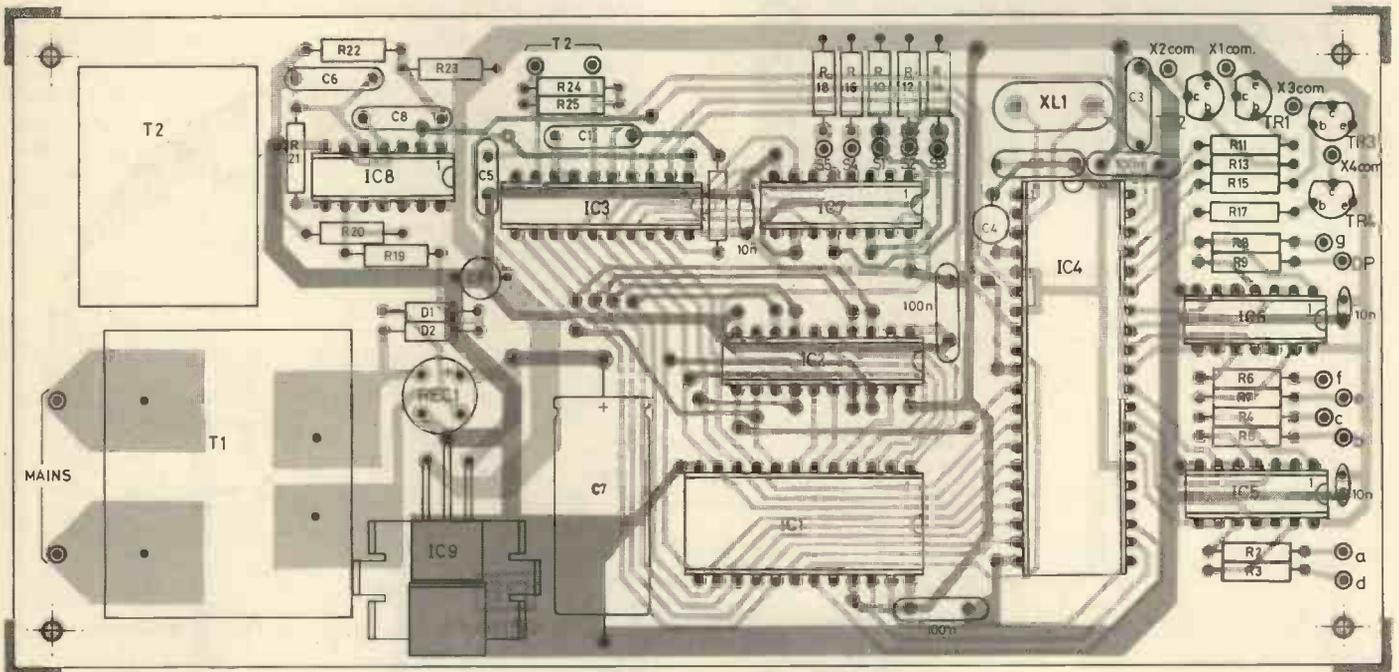
Fig. 8. Assembly details of board
