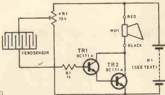
Fig. 1. Circuit of Alarm
