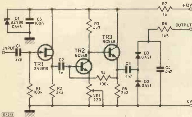
Fig. 3.1. Circuit diagram of the S-meter module
