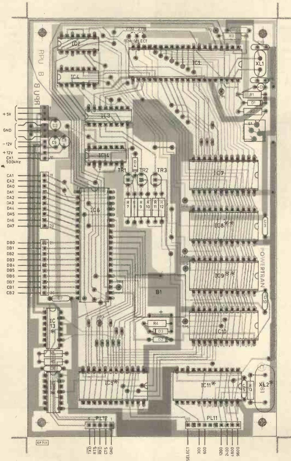
Fig. 1. Robot controller \*RS232 version only. \*\*Not used at present
