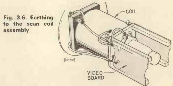
Fig. 3.6. Earthing to the scan coil assembly
