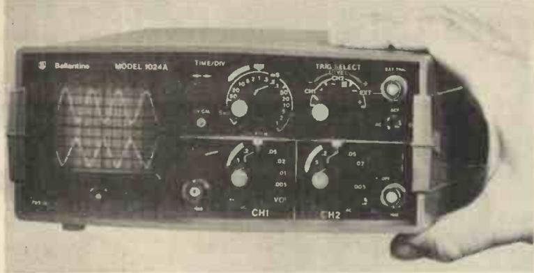
The new Ballantine 1024A mini oscilloscope, available from PPM Limited, has been designed to suit the needs of the field engineer, and light weight and small size have been achieved without reduction in instrument performance. The 1024A's specification is equal to laboratory bench scopes two or three times larger and heavier; it is shock and weather proof and will operate in harsh environments. The 1024A weighs 2.1 kilos and measures 87mm x 203mm x 220mm.
