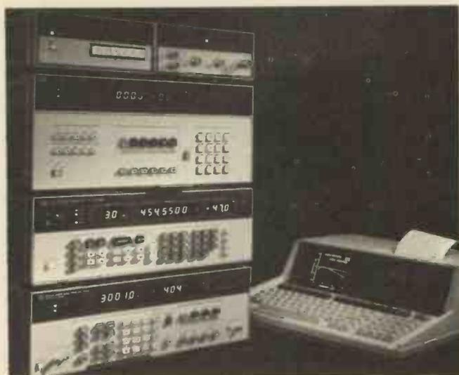
Hewlett Packard 8903A transceiver test set under the control of an HP85F
