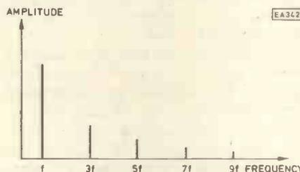
Fig. 3 Frequency spectrum for a square wave
