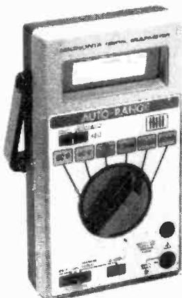
Features "beep" continuity check and autoranging function! Measures up to 1000 VDC, 500 VAC, 200 mA (both AC and DC), 2 megs resistance. Accurate to within  $\pm 1$  digit. 6 3/8". Requires two "AA" batteries. 22-192 ..... £69.95
